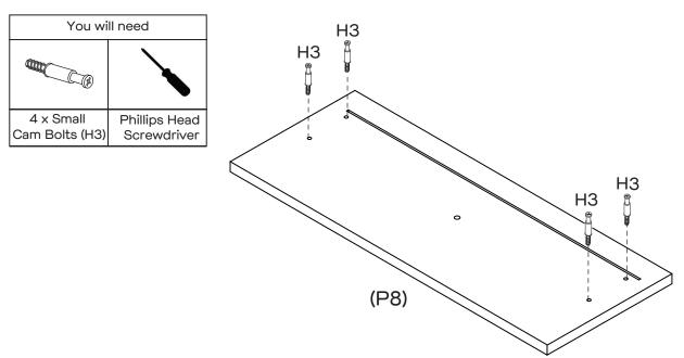
Attach 4 x Small Cam Bolts (H1O) into Drawer Front (P8). Tighten with a Phillips Head Screwdriver.
