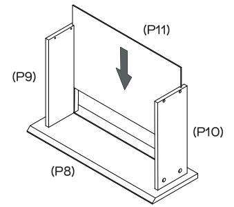
Slide Drawer Base (P11) into the groove in Drawer Sides (P9) and (P10).
