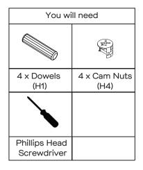
Insert 4 x Dowels (H1) into Side Panels (P2) and (P3).Insert 4 x Cam Nuts (H4) into the holes of Side Panels (P2) and (P3).Rotate the cam nuts so the arrows point towards the incoming cam bolts. Attach Top Panel (P1) and tighten the cam nuts.
