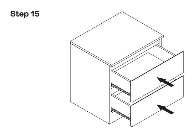
Insert the assembled drawers into the corresponding compartments as shown. Ensure the drawers slide easily along the rails.
