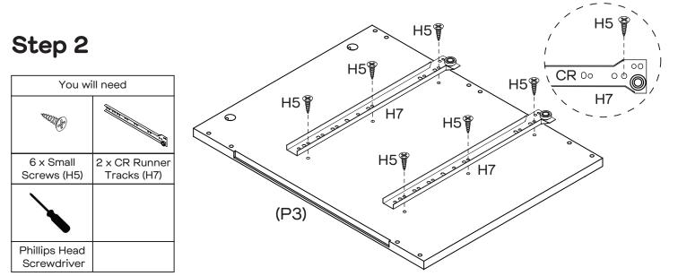
Attach  $2 \times CR$  Runner Tracks (H7) to Right Side Panel (P3) with  $6 \times Small Screws$  (H5) by tightening with the Phillips Head Screwdriver.
