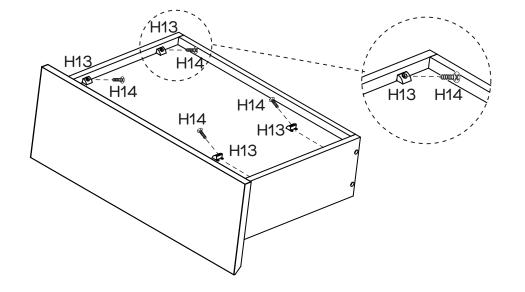
Attach 4 x Wedges (H13) into the gap between Drawer Sides (P9,P10) and Drawer Base (P11) with 4 x Screws (H14).
