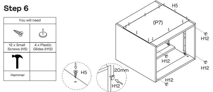
Put Back Panel (P7) into the groove on the back of the chest, screw it with  $12 \times \text{Small Screws}$  (H5). Then hammer  $4 \times \text{Plastic Glides}$  (H12) on Side Panels (P2) and (P3).
