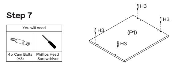
Attach 4 x Cam Bolts (H3) into Top Panel (P1) as shown. Tighten with a Phillips Head Screwdriver.
