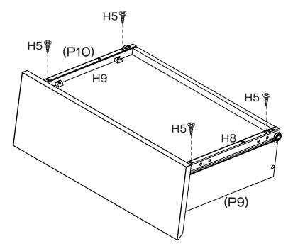
Attach 1 x DL Runner (H8) to the bottom of Left Drawer Side (P9) and 1 x DR Runner (H9) to the bottom of Right Drawer Side (P10) with  $4 \times$  Small Screws (H5). Repeat step 9 to step 14 to assemble the other drawer.
