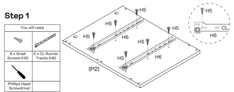
Attach  $2 \times CL$  Runner Tracks (H6) to Left Side Panel (P2) with  $6 \times Small Screws$  (H5) by tightening with the Phillips Head Screwdriver.
