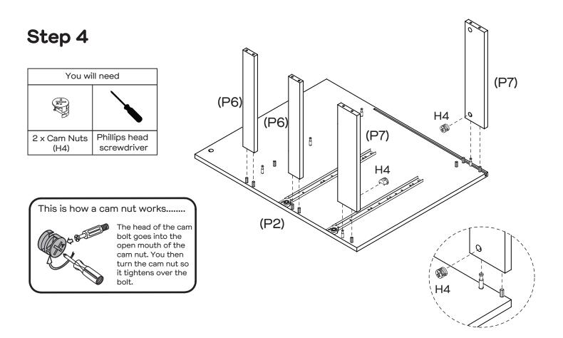
Insert 1 x Cam Nut (H4) into each Rail (P7x2). Rotate the cam nuts so the arrows point towards the incoming cam bolts. Attach Rails (P7x2) to the Left Side Panel (P2) by tightening the cam nuts with the Phillips Head Screwdriver. Attach Rails (P6x2) to Left Side Panel (P2) as shown.
