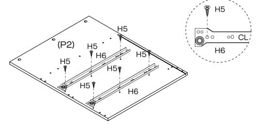
Attach 2 x CL Runner Tracks (H6) to Left Side Panel (P2) with 6 x Small Screws (H5) by tightening with the Phillips Head Screwdriver.
