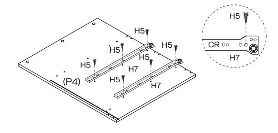
Attach 2 x CR Runner Tracks (H7) to Divider (P4) with  $6 \times 8$  Small Screws (H5) by tightening with the Phillips Head Screwdriver.
