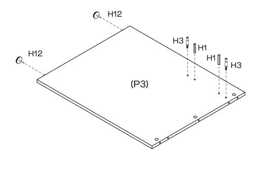
Insert 2  $\times$  Dowels (H1) into Right Side Panel (P3). Attach 2  $\times$  Cam Bolts (H3) to Right Side Panel (P3) by tightening with the Phillips Head Screwdriver. Use the Hammer to secure the 2  $\times$  Plastic Glides (H12) to the bottom of Right Side Panel (P3) as shown.
