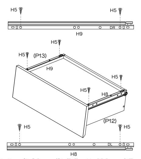
Attach 1 x DL Runner (H8) to the bottom of Left Drawer Side (P12) and 1 x DR Runner (H9) to the bottom of Right Drawer Side (P13) with  $4 \times 5$  Small Screws (H5) by tightening with the Phillips Head Screwdriver. Repeat steps for the second drawer
