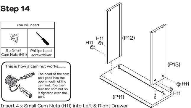
Sides (P12&P13). Rotate the cam nuts so the arrows point towards the incoming cam bolts. Attach Left & Right Drawer Sides (P12&P13) to the Drawer Front (P11) by tightening cam nuts with the Phillips Head Screwdriver. Repeat steps for the second drawer.
