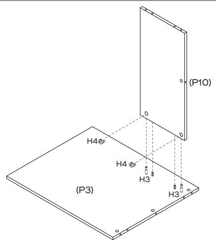
Insert 2 x Cam Nuts (H4) into Back Panel (P10). Rotate the cam nuts so the arrows point towards the incoming cam bolts. Attach Back Panel (P10) to Right Side Panel (P3) by tightening cam nuts with the Phillips Head Screwdriver.
