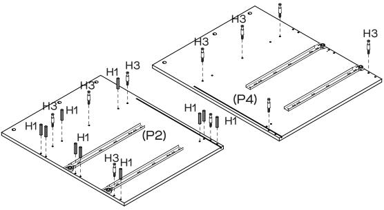
Insert 10 x Dowels (H1) into Left Side Panel (P2). Attach 10 x Cam Bolts (H3) into Left Side Panel (P2) and Divider (P4) by tightening with the Phillips Head Screwdriver as shown
