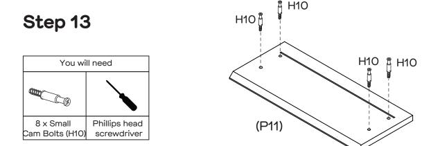
Attach 4 x Small Cam Bolts (H10) to Drawer Front (P11) by tightening with the Phillips Head Screwdriver. Repeat steps for the second drawer.
