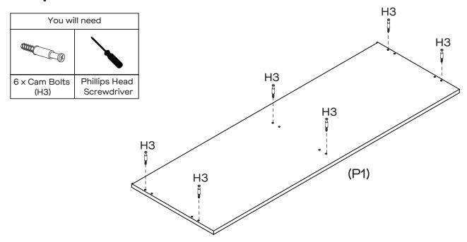
Attach 6 x Cam Bolts (H3) into Top Panel (P1) as shown. Tighten with a Phillips Head Screwdriver.
