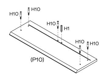
Insert 1 x Dowel (H1) into Drawer Front (P10). Attach 5 x Small Cam Bolts (H10) as shown.
