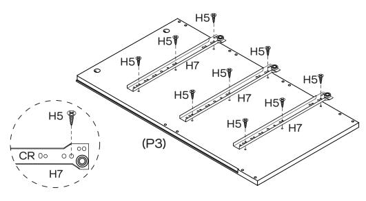
Attach 3 x CR Runner Tracks (H7) to Right Side Panel (P3) with  $9 \times 1$  Small Screws (H5) by tightening with the Phillips Head Screwdriver.
