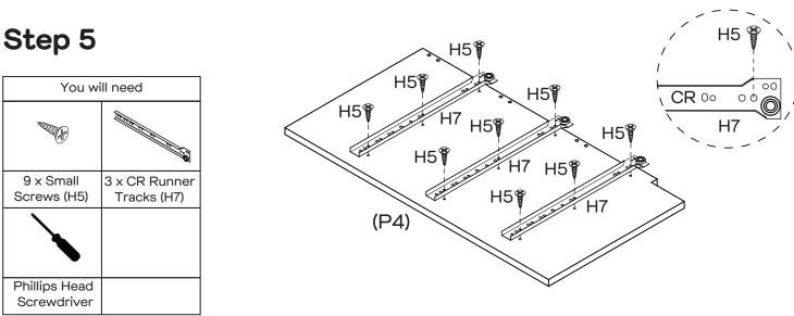
Turn Divider (P4) over to the other side, and then attach  $3 \times CR$  Runner Tracks (H7) with  $9 \times Small$  Screws (H5).
