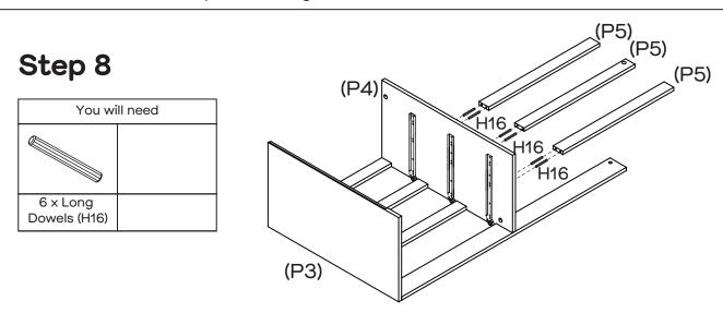
Insert 6 x Long Dowels (H16) into 3 x Rails (P5) and Divider (P4).
