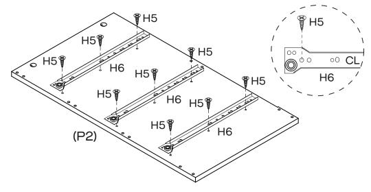
Attach 3  $\times$  CL Runner Tracks (H6) to Left Side Panel (P2) with 9  $\times$  Small Screws (H5) by tightening with the Phillips Head Screwdriver.
