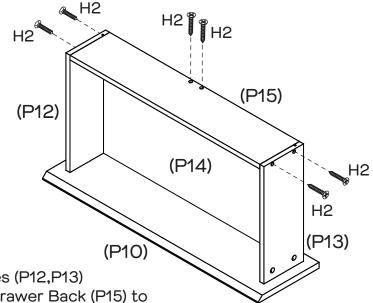
Attach Drawer Back (P15) to Drawer Sides (P12,P13) with  $4 \times 1$  Long Screws (H2), then attach Drawer Back (P15) to Support Rail (P16) with  $2 \times 1$  Long Screws (H2).
