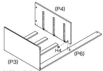
Insert 1 x Cam Nut (H4) into the hole of Divider (P4).
