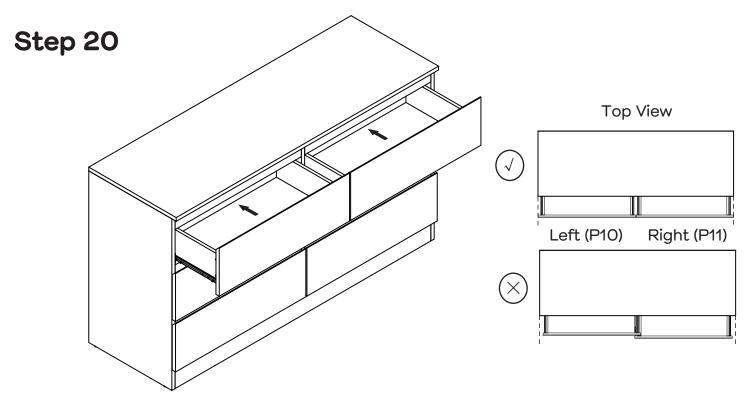
There are specific Left (P10) and Right (P11) Drawers. Put the drawers into the chest. So the drawer fronts align with the outside of the side panels.
