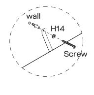
Move the dresser to the final position, and attach the safety strap to the wall securely. Make sure it is firmly attached and snug fit.
