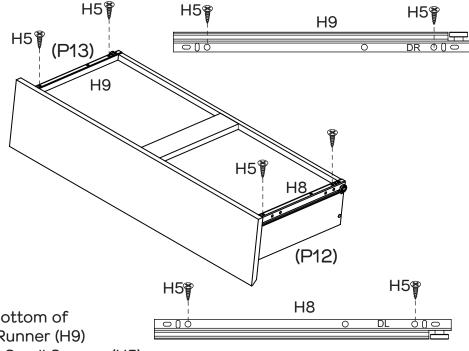
Attach 1 x DL Runner (H8) on the bottom of Left Drawer Side (P12) and 1 x DR Runner (H9) of Right Drawer Side (P13) with 4 x Small Screws (H5).
