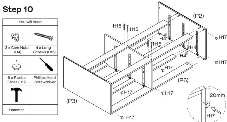
Insert 3 x Cam Nuts (H4) into the holes of Rails (P6,P7) and (P8). Rotate the cam nuts so the arrows point towards the incoming cam bolts. Push Left Side Panel (P2) into place and tighten the cam nut. Attach Rails (P7) and (P8) to Divider (P4) with 4 x Long Screws (H15). Then hammer 6 x Plastic Glides (H17) on Side Panels (P2,P3) and Divider (P4).
