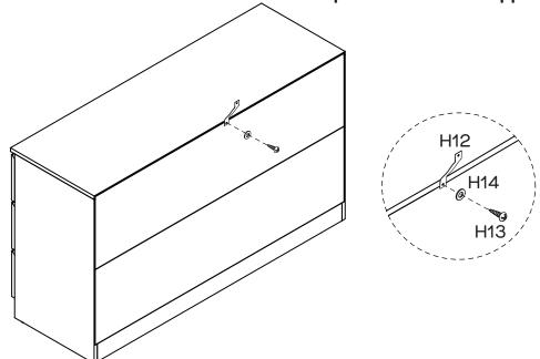
Attach Safety Strap (H12) to the Top Panel (P1) using 1 x Screw (H13) and 1 x Washer (H14).
