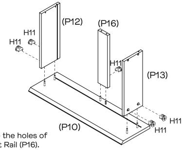
Insert 5 x Small Cam Nuts (H11) into the holes of Drawer Sides (P12,P13) and Support Rail (P16).
