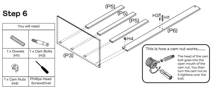
Insert 1 x Cam Nut (H4) into the hole of Rail (P6). Rotate the cam nut so the arrows point towards the incoming cam bolt. Insert 1 x Dowel (H1) into Rail (P6). Attach 1 x Cam Bolt (H3) into Rail (P6) as shown. Attach 3 x Rails (P5) and Rail (P6) to Right Side Panel (P3), then tighten the cam nuts.
