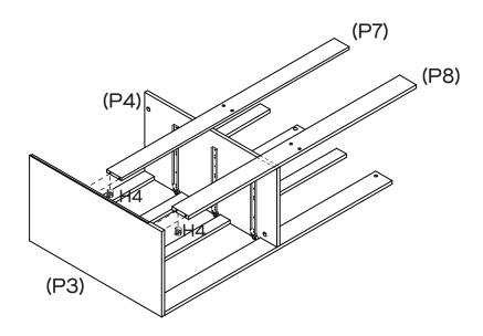
Insert 2 x Cam Nuts (H4) into the holes of Rails (P7) and (P8). Rotate the cam nuts so the arrows point towards the incoming cam bolts and tighten the cam nuts.
