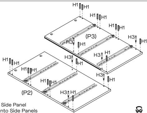
Insert 18 x Dowels (H1) into Left Side Panel (P2). Attach 6 x Cam Bolts (H3) into Side Panels
