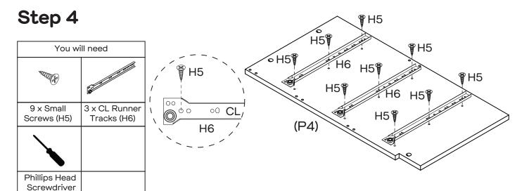
Attach 3 x CL Runner Tracks (H6) to Divider (P4) with 9 x Small Screws (H5) by tightening with the Phillips Head Screwdriver.
