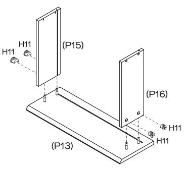
Insert 4 x Small Cam Nuts (H11) into the holes of Drawer Sides (P15,P16). Rotate the cam nuts so the arrows point towards the incoming cam bolts. Push Drawer Side (P15,P16) into place and tighten the cam nuts.
