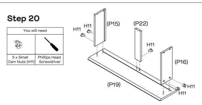
Insert 5 x Small Cam Nuts (H11) into the holes of Drawer Sides (P15, P16) and Support Rail (P22). Rotate the cam nuts so the arrows point towards the incoming cam bolts.
