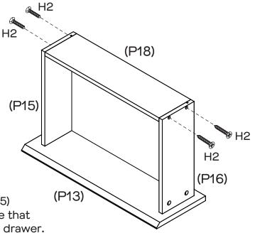
Attach Drawer Back (P18) to Drawer Sides (P15) and (P16) with 4 x Long Screws (H2),make sure that the groove lines up the whole way around the drawer.
