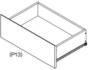
Repeat step 13 to step 17 with Drawer Front (P14) to assemble the other drawer.
