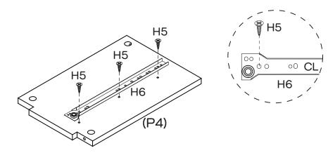
Attach 1 x CL Runner Track (H6) to Divider (P4) with 3 x Small Screws (H5) by tightening with the Phillips Head Screwdriver.
