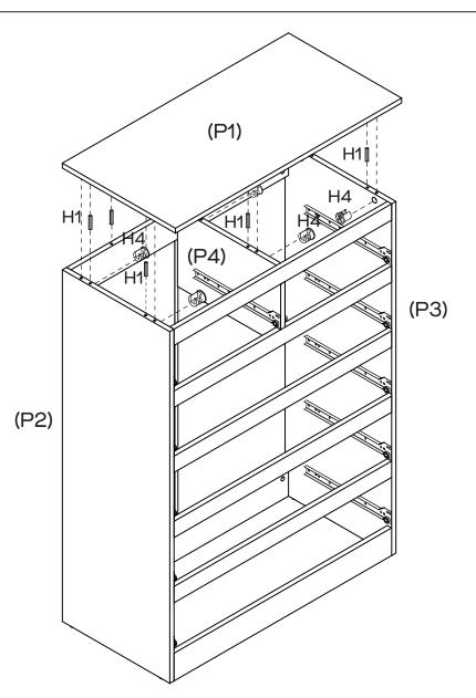
Insert 8 x Dowels (H1) into the holes of Side Panels (P2,P3), Divider (P4) and Rail (P9). Insert 6 x Cam Nuts (H4) into the holes of Side Panels (P2,P3) and Divider (P4). Rotate the cam nuts so the arrows point towards the incoming cam bolts. Attach Top Panel (P1) and tighten the cam nuts.
