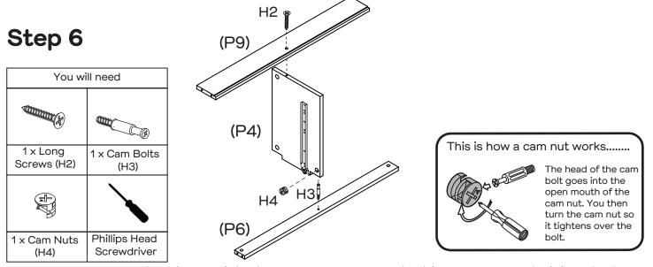
Attach 1 x Cam Bolt (H3) into Rail (P6). Insert 1 x Cam Nut (H4) into the hole of Divider (P4). Rotate the cam nut so the arrow point towards the incoming cam bolt. Push Divider (P4) into place and tighten the cam nut.
