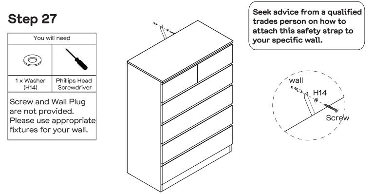
Move the dresser to the final position, and attach the safety strap to the wall securely. Make sure it is firmly attached and snug fit.
