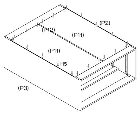
Join 2  $\times$  Back Panels (P11) with Connect Stick (P12), then put into the groove on the back of the chest, screw it with 22  $\times$  Small Screws (H5).
