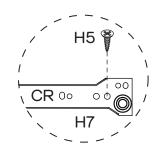
Turn Divider (P4) over to the other side, then attach 1 x CR Runner Track (H7) with 3 x Small Screws (H5) by tightening with the Phillips Head Screwdriver.
