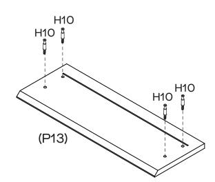
Attach 4 x Small Cam Bolts (H10) into Drawer Front (P13) by tightening with the Phillips Head Screwdriver.
