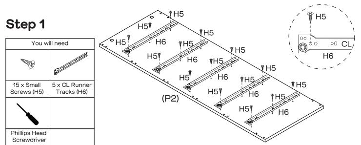
Attach 5 x CL Runner Tracks (H6) to Left Side Panel (P2) with 15 x Small Screws (H5) by tightening with the Phillips Head Screwdriver.
