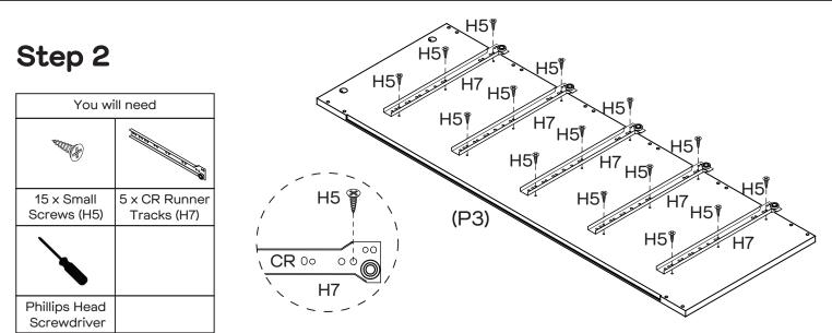
Attach 5 x CR Runner Tracks (H7) to Right Side Panel (P3) with 15 x Small Screws (H5) by tightening with the Phillips Head Screwdriver.
