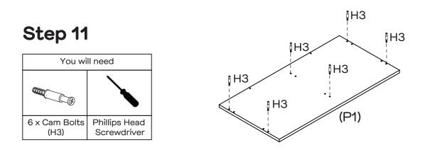
Attach  $6 \times Cam$  Bolts (H3) into Top Panel (P1) as shown by tightening with the Phillips Head Screwdriver.
