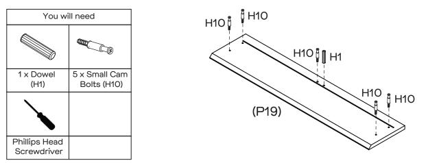
Insert 1 x Dowel (H1) into Drawer Front (P19),and attach 5 x Small Cam Bolts (H10) into it.
