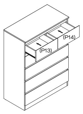
Insert the assembled drawers into the corresponding compartments as shown. Ensure the drawers slide easily along the rails.
