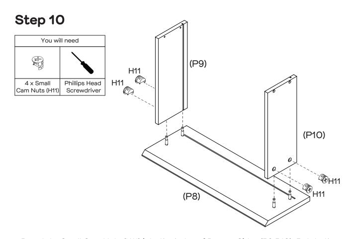
Insert 4 x Small Cam Nuts (H11) into the holes of Drawer Sides (P9,P10). Rotate the cam nuts so the arrows point towards the incoming cam bolts. Push Drawer Sides (P9,P10) into place and tighten the cam nuts.
