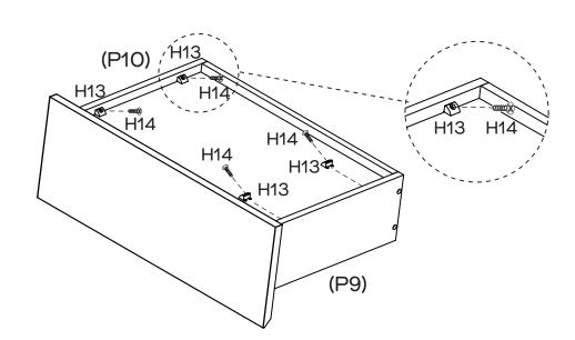
Attach 4 x Wedges (H13) into the gap between Drawer Sides (P9,P10) and Drawer Base (P11) with 4 x Screws (H14).
