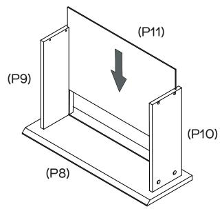
Slide Drawer Base (P11) into the groove in Drawer Sides (P9) and (P10).
