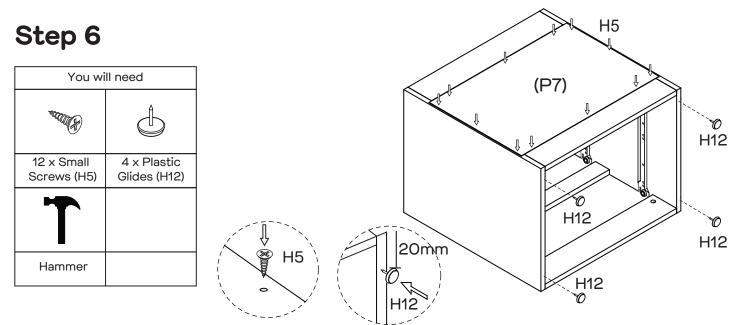
Put Back Panel (P7) into the groove on the back of the chest, screw it with 12  $\times$  Small Screws (H5). Then hammer 4  $\times$  Plastic Glides (H12) on Side Panels (P2) and (P3).
