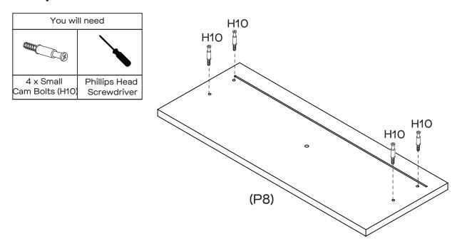
Attach 4 x Small Cam Bolts (H10) into Drawer Front (P8). Tighten with a Phillips Head Screwdriver.
