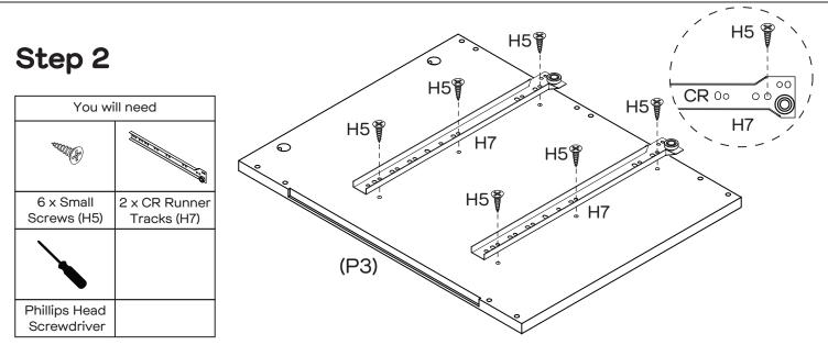
Attach 2  $\times$  CR Runner Tracks (H7) to Right Side Panel (P3) with 6  $\times$  Small Screws (H5) by tightening with the Phillips Head Screwdriver.
