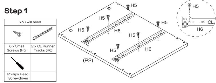
Attach 2 x CL Runner Tracks (H6) to Left Side Panel (P2) with 6 x Small Screws (H5) by tightening with the Phillips Head Screwdriver.
