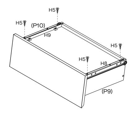
Attach 1 x DL Runner (H8) to the bottom of Left Drawer Side (P9) and 1 x DR Runner (H9) to the bottom of Right Drawer Side (P10) with 4 x Small Screws (H5). Repeat step 9 to step 14 to assemble the other drawer.
