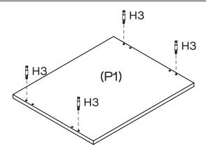
Attach 4 x Cam Bolts (H3) into Top Panel (P1) as shown. Tighten with a Phillips Head Screwdriver.
