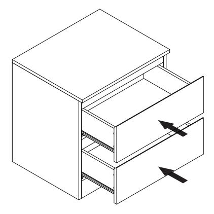
Insert the assembled drawers into the corresponding compartments as shown. Ensure the drawers slide easily along the rails.
