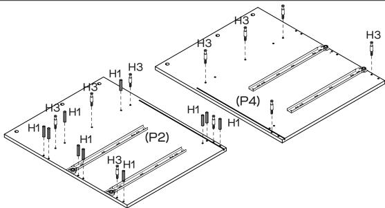
Insert 10  $\times$  Dowels (H1) into Left Side Panel (P2). Attach 10  $\times$  Cam Bolts (H3) into Left Side Panel (P2) and Divider (P4) by tightening with the Phillips Head Screwdriver as shown
