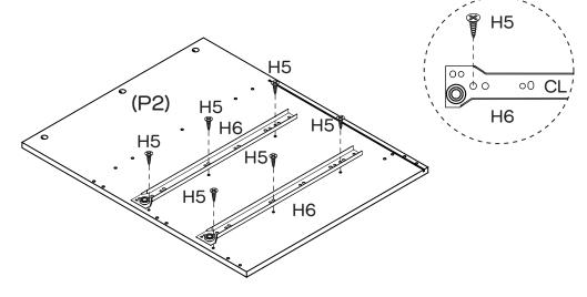
Attach 2  $\times$  CL Runner Tracks (H6) to Left Side Panel (P2) with 6  $\times$  Small Screws (H5) by tightening with the Phillips Head Screwdriver.
