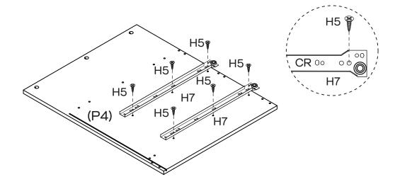
Attach 2 x CR Runner Tracks (H7) to Divider (P4) with  $6 \times 5$  Small Screws (H5) by tightening with the Phillips Head Screwdriver.
