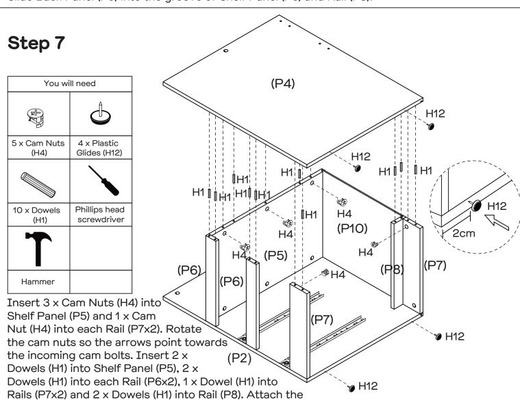
Divider Panel (P4) to the partially assembled unit by tightening the cam nuts with the Phillips Head Screwdriver. Use the Hammer to secure the 4 x Plastic Glides (H12) to the bottom of Left Side Panel (P2) and Divider Panel (P4) as shown.
