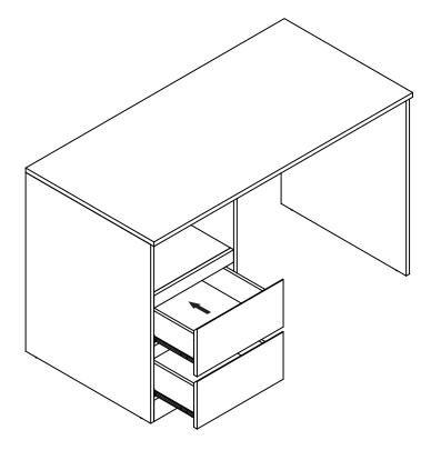
Carefully insert the drawers into the desk by gently guiding the runners into the tracks.
