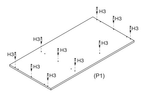
Attach 10  $\times$  Cam Bolts (H3) to Top Panel (P1) by tightening with the Phillips Head Screwdriver.
