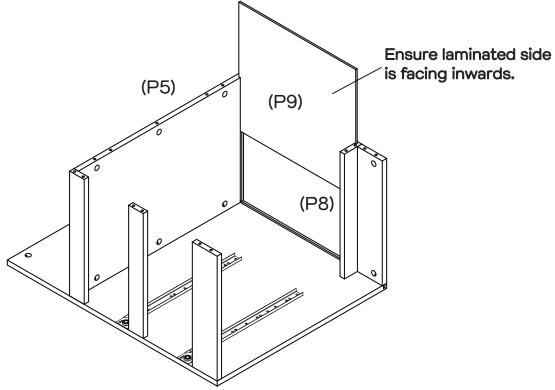
Slide Back Panel (P9) into the groove of Shelf Panel (P5) and Rail (P8).
