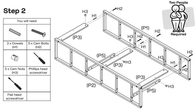
Insert 3 x Dowels (H1) into Left Side Frame (P1). Push 5 x Cam Bolts (H2) through Left Side Frame (P1) attach with Rails (P3, P5) with 5 x Cam Nuts (H3) using a Flat head screwdriver. Tighten with Phillips head screwdriver.
