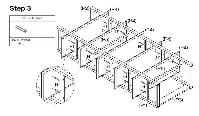
Insert 20 x Dowels (H1) into Side Frames (P1, P2) and attach with Shelf Panels (P4).
