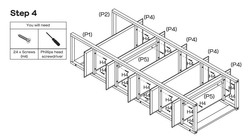
Attach Shelf Panels (P4) to Side Frames (P1, P2) and Shelf Panels (P4) to Rails (P5) with 24 x Screws (H4) using a Phillips head screwdriver. Tighten with Phillips head screwdriver.
