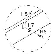
Use Screw (H6) and Washer (H7) to connect Safety Strap (H5) on Rail (P3).
