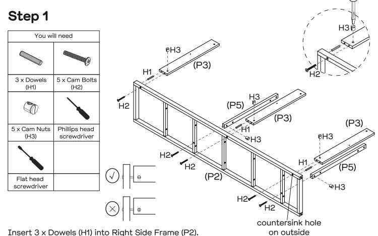
Insert 3  $\times$  Dowels (H1) into Right Side Frame (P2). Push 5  $\times$  Cam Bolts (H2) through Right Side Frame (P2) attach with Rails (P3, P5) with 5  $\times$  Cam Nuts (H3) using a Flat head screwdriver. Tighten with Phillips head screwdriver.
