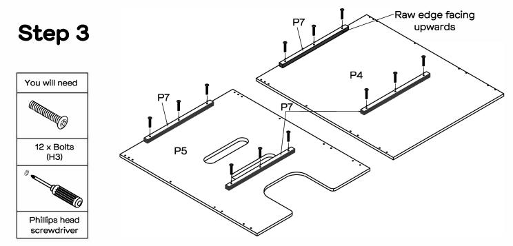
Attach 4 x Short Support Panels (P7) to Headboard (P4) and Footboard (P5) by using  $12 \times Bolts$  (H3).
