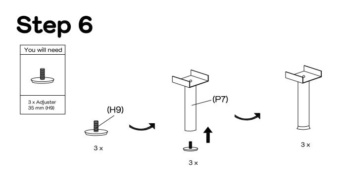
Attach adjuster (H9) to support legs (P7). Please ensure the adjuster (H9) is completely retracted / screwed in.
