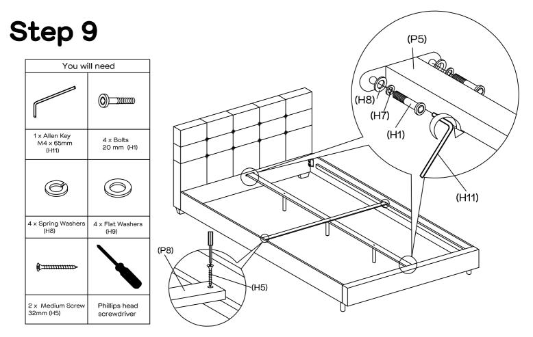
Attach centre rail (P5) to the Headboard (P1) and Footboard (P2) using 4x bolts (H1), Spring Washers (H7) and Flat Washers (H8) as shown. Attach the cross rail (P8) to the centre of side rails (P3,P4) using medium screw (H5).
