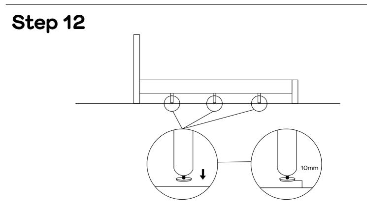
Using two people to move this bed to its final resting position. Extend adjuster (H9) such that they sit / rest 10 mm above the floor before you place the mattress on the bed.
