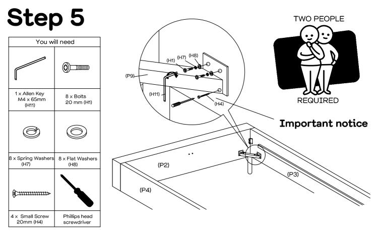
Attach P9 to side-rail and footboard, on both corners. 2 people required (1 person needs to support the other corner while attaching the 1st P9 to the bed.) **(Important notice : Please ensure H4 is attach into P3,P4 and P2. This is important.)**
