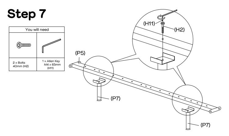
Attach each support legs (P7) to the centre rail (P5) using 2x bolts (H2) as shown.
