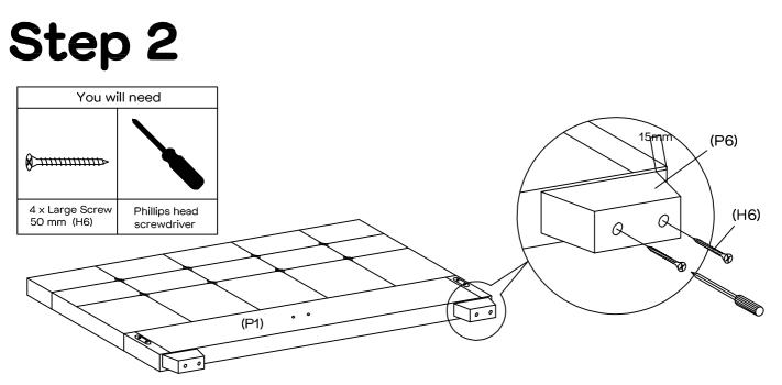
Attach legs (P6) to the bottom of headboard (P1) with 4 x large screws (H6). The self-tapping screws provided do not require a hole to attach. Apply some pressure to the screw at the beginning, it will start to work itself into the timber frame. Keep applying the pressure as you screw until the leg is firmly attached. Repeat for the 3 other screws.
