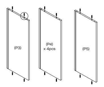
Using a mallet, gently tap 24x Wood Dowels (H2) into pre-drilled holes in Top Panel (P3), 4x Shelf Panels (P4) and Bottom Panel (P5).
