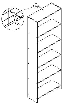
Move furniture to its final position, then connect the end of the Webbing (H4) to the wall, ensuring it is firmly attached. Seek advice from a qualified trades person on how to attach this to your specific wall. Screws and wall plugs are not supplied. Please use appropriate fixtures for your wall.
