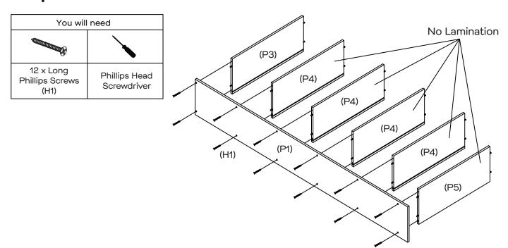
Attach Top Panel (P3), 4x Shelf Panels (P4) and Bottom Panel (P5) to the Side Panel Left (P1) with 12x Long Phillips Screws (H1). Tighten with a phillips head screwdriver.
