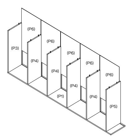
Slide 5x Back Panels (P6) into grooves of Top Panel (P3), 4x Shelf Panels (P4) and Bottom Panel (P5).
