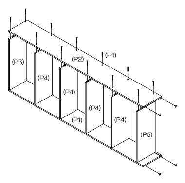
Fix Side Panel Right (P2) to main assembly with 12x Long Phillips Screws (H1) and tighten with a phillips head screwdriver. Using a Mallet, gently tap 4x Plastic Leg Studs (H3) into the base of both Shelf Panels (P1 and P2) as shown.
