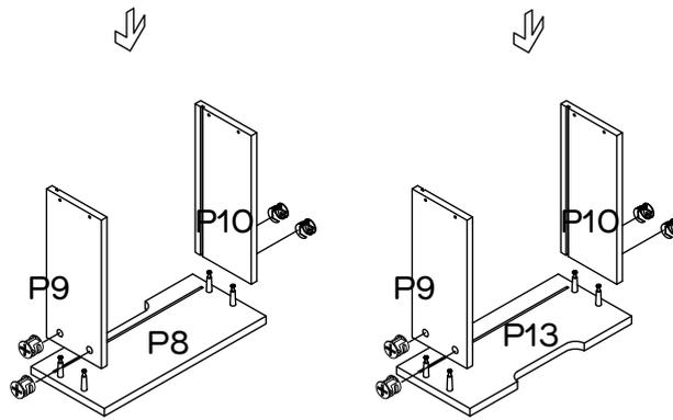
Insert 8 x Cam Nuts (H2) into holes on (P9) & (P10), rotate the Cam Nuts, so the arrow point towards the incoming Cam Bolts. Attach Left Drawer Side (P9) and Right Drawer Side (P10) to the Drawer Front (P8) & (P13), turn the Cam Nuts clockwise to tighten.
