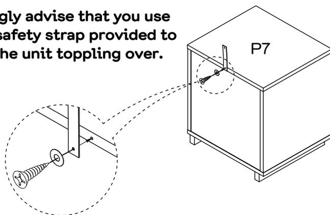
Attach the Washer (H11) to the top panel (P7) using 1 x screw (H13) and 1 x Wall strap (H12).
