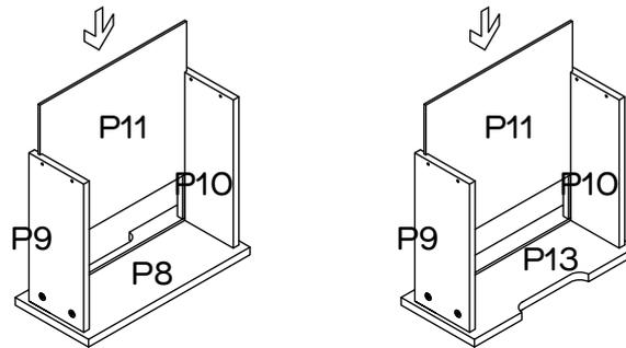
Insert the Drawer Bottom (P11) to the Drawer Frame as shown.
