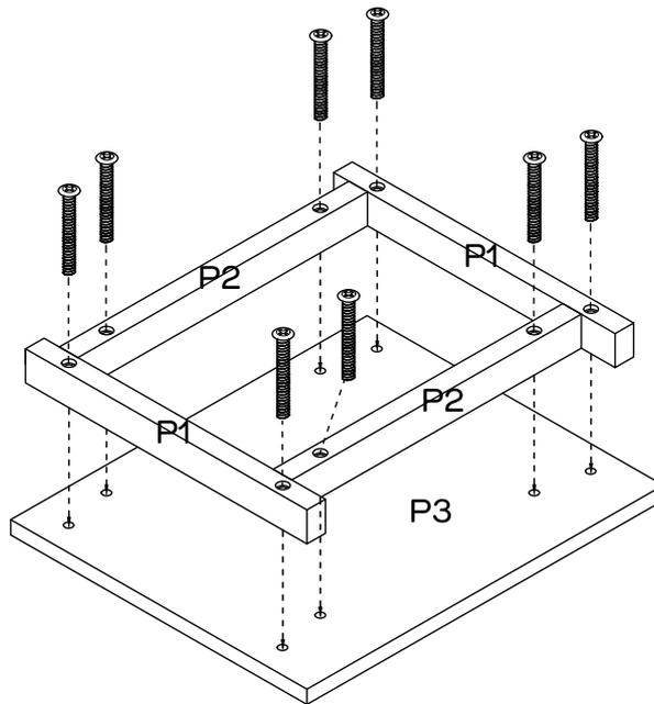
Attach 2 x Long Bottom Rails (P1), 2 x Short Bottom Rails (P2) to Base Panel (P3) with 8 x Bolts (H4) by using a Phillips head screwdriver.
