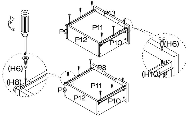
Attach 2 x Left Drawer Runners to 2 x Left Drawer Side (P9) and 2 x Right Drawer Runners to 2 x Right Drawer Side (P10) with 12 x Screws (H6) by using a Phillips head screwdriver.
