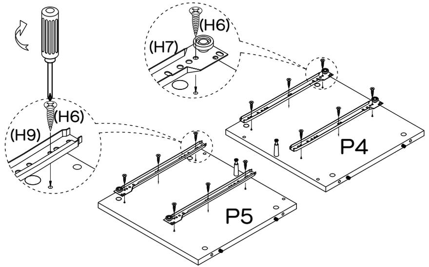
Attach 2 x Right Runner Tracks (H9) to Right Side Panel (P5) and 2 x Left Runner Tracks (H7) to Left Side Panel (P4) with 12 x Screws (H6) by using a Phillips head screwdriver.
