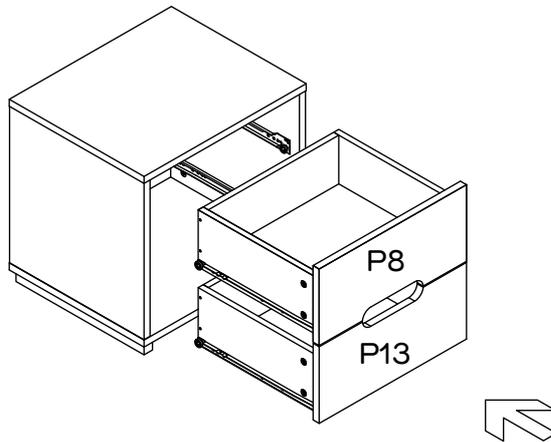
To insert the drawers, just gently put the left and right drawer runner on the Left and right track runner and push the drawers close.
