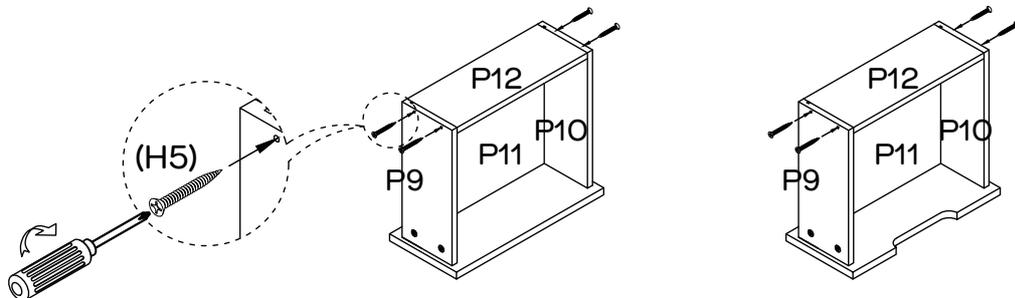
Attach the Drawer Back (P12) to the Left & Right Drawer Side (P9) & (P10) with 8 x Screws (H5) by using a Phillips head screwdriver.
