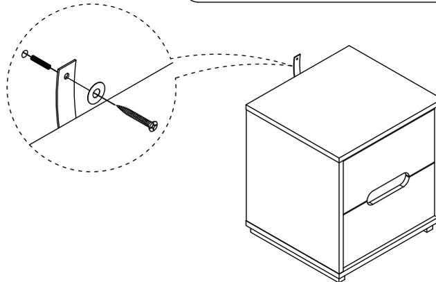
Move the Chest to final position. Attach the safety strap to the wall. Make sure it is firmly attached and make sure it is snug fit.
