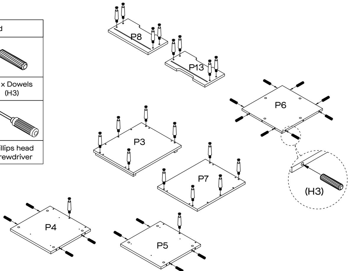
Insert 20 x Cam Bolts (H1), to panels (P3), (P4), (P5), ( P6), (P7), (P8), (P13) and 16 x Dowels (H3) to panels (P4), (P5), (P6) as shown.
