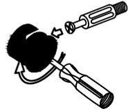
The head of the cam bolt goes into the open mouth of the cam nuts. You then turn the cam nuts so it tightens over the bolt.
