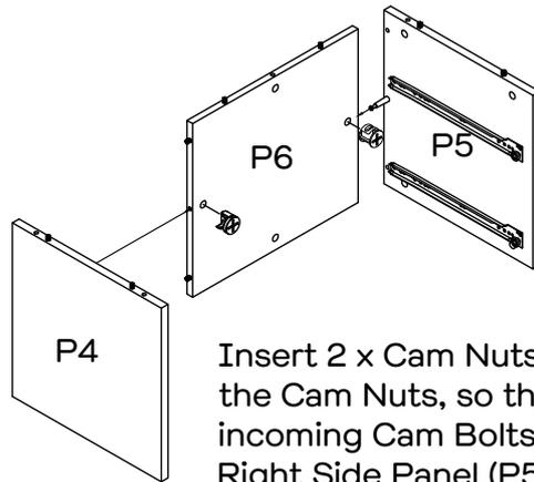
**This is how a cam nuts works.....**
