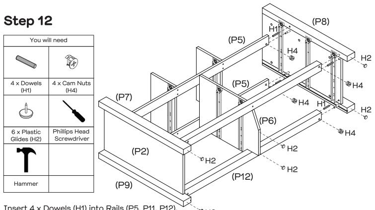
Insert 4 x Dowels (H1) into Rails (P5, P11, P12). H2 Insert 4 x Cam Nuts (H4) into the holes of Rails (P5, P11, P12). Rotate the cam nuts so the arrows point towards the incoming cam bolts. Attach Right Side Panel (P2) with Rails (P5, P11, P12) securely and tighten the cam nuts. Attach 6 x Plastic Glides (H2) on Legs (P7, P8, P9, P10) and Divider (P6) with a Hammer.
