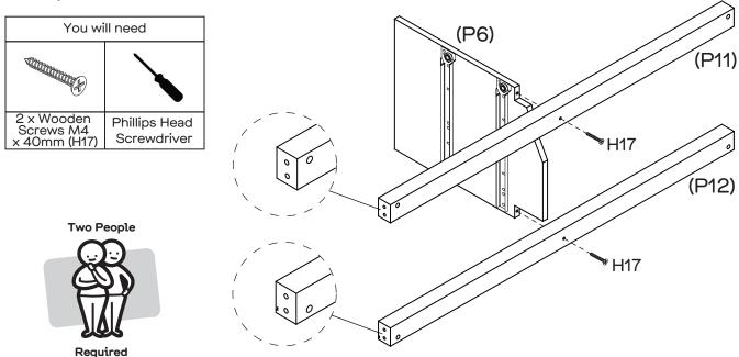
Attach Rails (P11, P12) to Divider (P6) with 2 x Wooden Screws (H17) using a Phillips head screwdriver.
