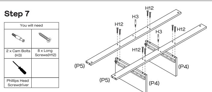
Attach Rails (P5) to Dividers (P4) with 8 x Long Screws (H12). Insert 2 x Cam Bolts (H3) into the holes of Rails (P5).
