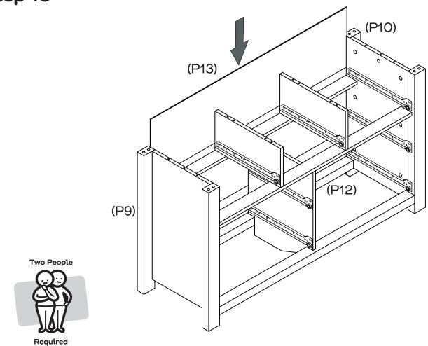
Carefully turn the cabinet over to an upright position. Slide Back Panels (P13) in through the grooves of Legs (P9, P10) and Rail (P12).
