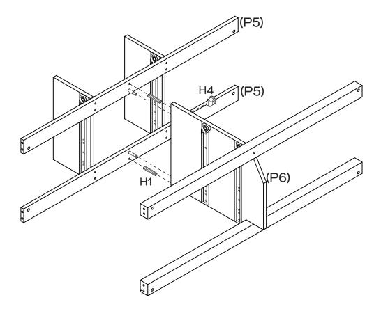
Insert 2 x Dowels (H1) into the holes of Rails (P5). Insert 2 x Cam Nuts (H4) into the holes of Divider (P6). Rotate the cam nuts so the arrows point towards the incoming cam bolts. Push Rails (P5) into place and tighten the cam nuts.
