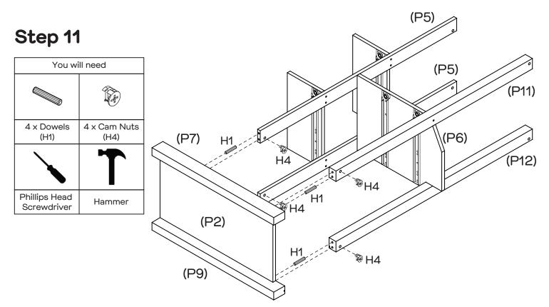
Insert 4 x Dowels (H1) into Rails (P5, P11, P12). Insert 4 x Cam Nuts (H4) into the holes of Rails (P5, P11, P12). Rotate the cam nuts so the arrows point towards the incoming cam bolts. Attach Left Side Panel (P2) with Rails (P5, P11, P12) securely, and tighten the cam nuts.
