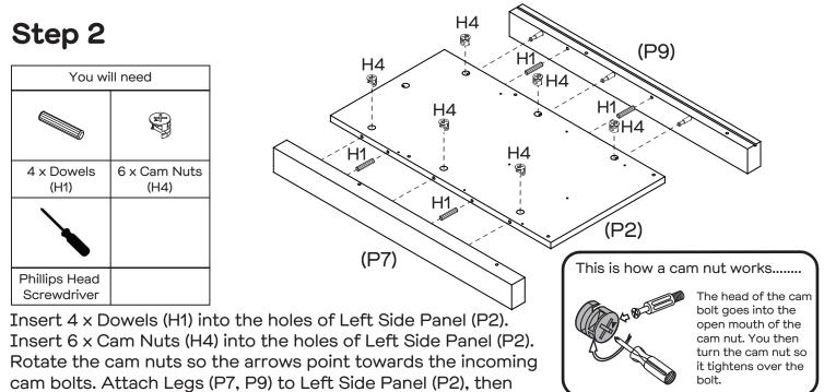
tighten the cam nuts.
