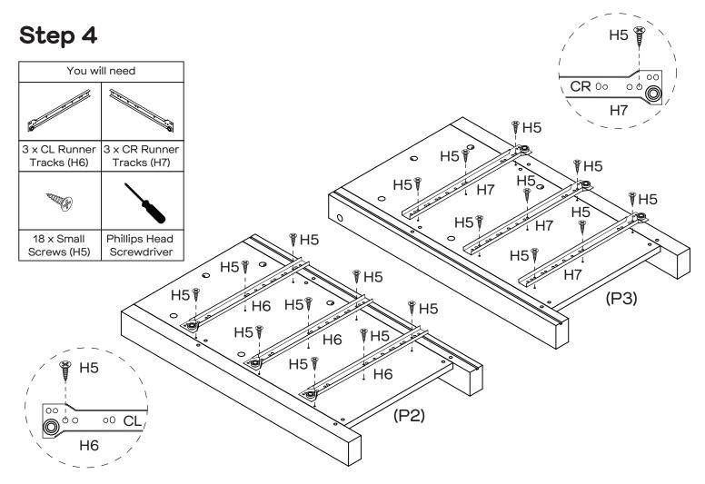
Attach 3 x CL Runner Tracks (H6) to Left Side Panel (P2) with 9 x Small Screws (H5). Attach 3 x CR Runner Tracks (H7) to Right Side Panel (P3) with 9 x Small Screws (H5).
