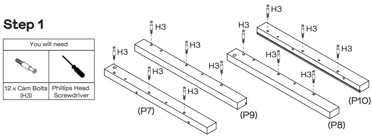
Attach 12 x Cam Bolts (H3) into Legs (P7, P8, P9, P10).
