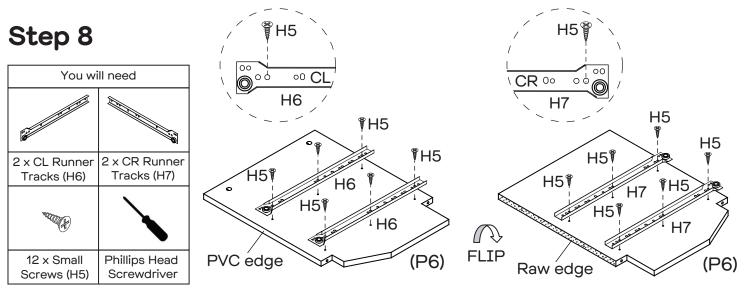
Attach 2 x CL Runner Tracks (H6) to Divider (P6) with 6 x Small Screws (H5). Turn Divider (P6) over to the other side, then attach 2 x CR Runner Tracks (H7) with 6 x Small Screws (H5).
