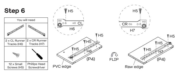
Attach 1 x CL Runner Track (H6) to Divider (P4) with 3 x Small Screws (H5). Turn Divider (P4) over to the other side, then attach 1 x CR Runner Track (H7) with 3 x Small Screws (H5). Repeat Step 6 for the other Divider (P4).
