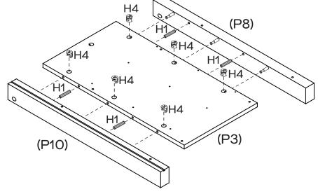
Insert 4 x Dowels (H1) into the holes of Right Side Panel (P3). Insert 6 x Cam Nuts (H4) into the holes of Right Side Panel (P3). Rotate the cam nuts so the arrows point towards the incoming cam bolts. Attach Legs (P8, P10) to Right Side Panel (P3), then tighten the cam nuts. fantasticfurniture.com.au
