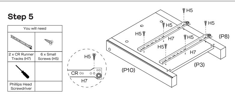
Attach 2 x CR Runner Tracks (H7) to Right Side Panel (P3) with 6 x Small Screws (H5).
