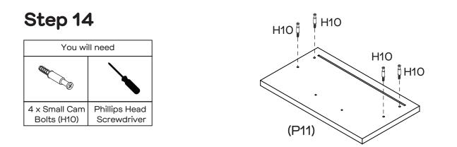
Screw 4 x Small Cam Bolts (H10) into Drawer Front (P11) with a Phillips head screwdriver.
