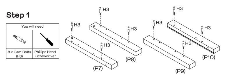
Attach 8 x Cam Bolts (H3) into Legs (P7, P8, P9, P10).
