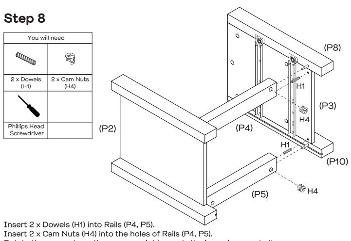
Rotate the cam nuts so the arrows point towards the incoming cam bolts. Align the holes and attach Legs (P8, P10) to Right Side Panel (P3). Tighten the cam nuts.
