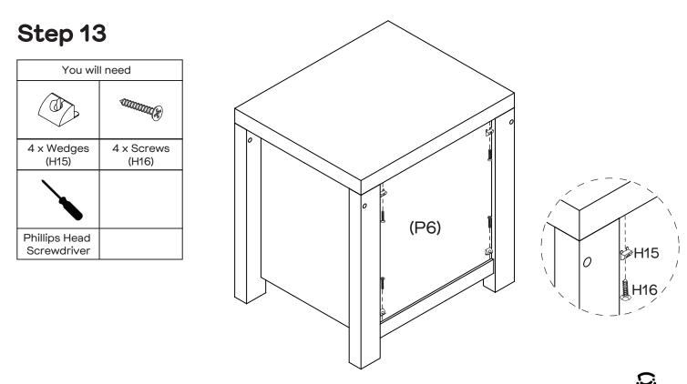
Secure Back Panel (P6) in place with 4 x Wedges (H15) using 4 x Screws (H16). fantasticfurniture.com.au
