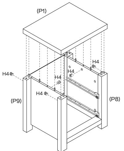
Insert 6 x Cam Nuts (H4) into the holes of Side Panels (P2, P3) and Legs (P7, P8, P9, P10). Rotate the cam nuts so the arrows point towards the incoming cam bolts. Attach Top Panel (P1) to the frame and tighten the cam nuts using a Phillips head screwdriver.
