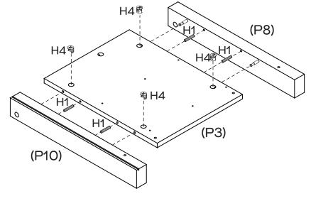
Insert 4 x Dowels (H1) into the holes of Right Side Panel (P3). Insert 4 x Cam Nuts (H4) into the holes of Right Side Panel (P3). Rotate the cam nuts so the arrows point towards the incoming cam bolts. Attach Legs (P8, P10) to Right Side Panel (P3), then tighten the cam nuts.
