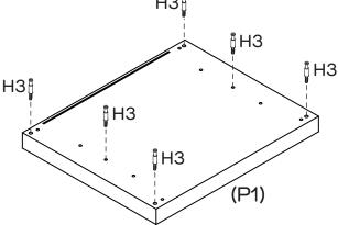
Attach 6 x Cam Bolts (H3) into Top Panel (P1) as shown.
