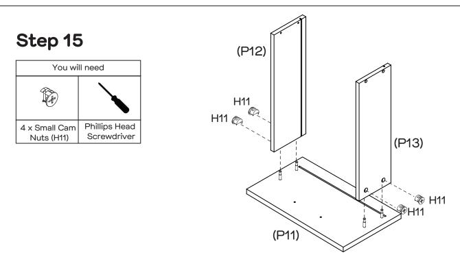
Insert 4 x Small Cam Nuts (H11) into the holes of Drawer Sides (P12, P13). Rotate the cam nuts so the arrows point towards the incoming cam bolts. Align the holes together, secure Drawer Sides (P12, P13) into place and tighten the cam nuts using a Phillips head screwdriver.
