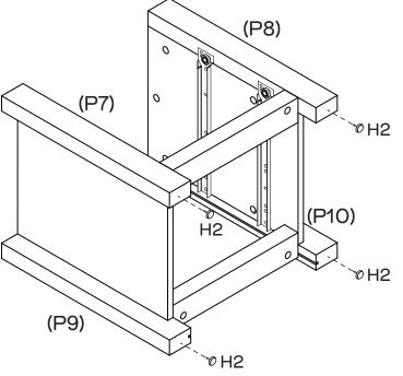
Attach 4 x Plastic Glides (H2) to the bottom of Legs (P7, P8, P9, P10) with a Hammer.
