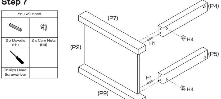
Insert 2 x Dowels (H1) into Rails (P4, P5). Insert 2 x Cam Nuts (H4) into the holes of Rails (P4, P5). Rotate the cam nuts so the arrows point towards the incoming cam bolts. Align the holes and attach Legs (P7, P9) to Left Side Panel (P2). Tighten the cam nuts.
