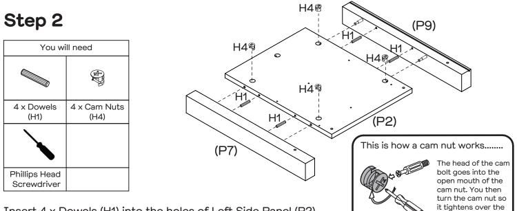
Insert 4 x Dowels (H1) into the holes of Left Side Panel (P2). Insert 4 x Cam Nuts (H4) into the holes of Left Side Panel (P2). Rotate the cam nuts so the arrows point towards the incoming cam bolts. Attach Legs (P7, P9) to Left Side Panel (P2), then tighten the cam nuts.
