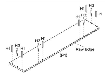
Insert 6 x Dowels (H1) into the holes of Top Panel (P1). Attach 4 x Cam Bolts (H3) into Top Panel (P1) as shown. fantasticfurniture.com.au
