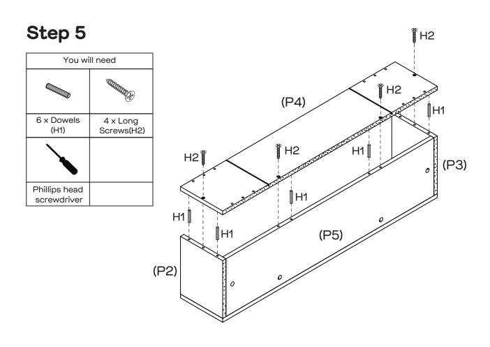
Insert 6 x Dowels (H1) into the holes of Side Panels (P2, P3) and Back Panel (P5). Attach Bottom Panel (P4) to the right place with 4 x Long Screws (H2) using a Philips head screwdriver.
