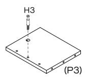
Attach 2 x Cam Bolts (H3) into Side Panels (P2, P3) as shown.
