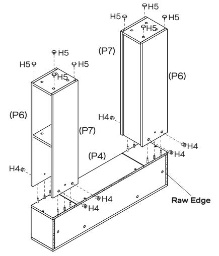
Insert 8 x Cam Nuts (H4) into the holes of Side Panels (P6, P7). Rotate the cam nuts so the arrows point towards the incoming cam bolts. Push the two frame into place, then tighten the cam nuts using the Phillips Head Screwdriver. Hammer 8 x Plastic Glides (H5) on the bottom of Side Panels (P6, P7) as shown.
