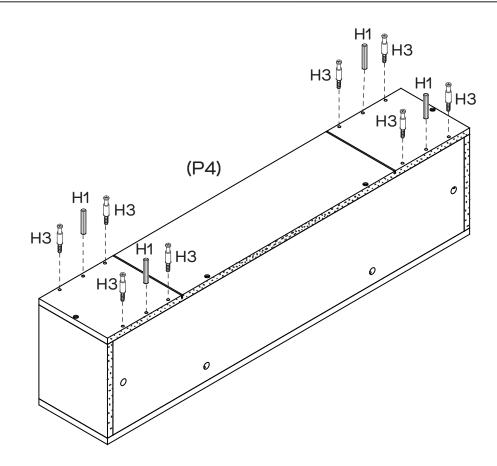
Insert 4 x Dowels (H1) into the holes of Bottom Panel (P4). Attach 8 x Cam Bolts (H3) into Bottom Panel (P4) as Shown.
