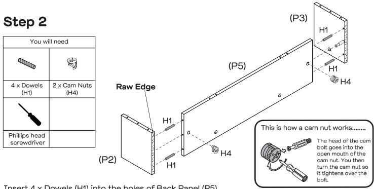
Insert  $4 \times Dowels$  (H1) into the holes of Back Panel (P5).
