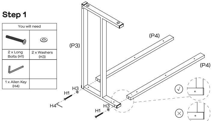
Attach Rails (P4) to Right Frame (P3) with 2 x Long Bolts (H1) and 2 x Washers (H3). — Tighten the bolts using an Allen Key (H4).
