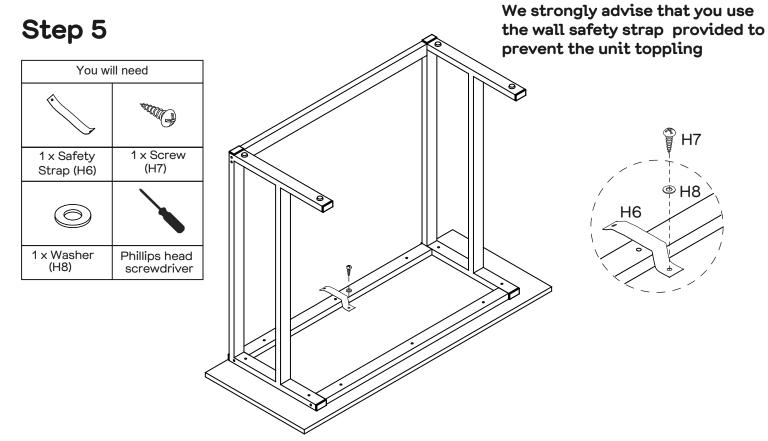
Use Screw (H7) and Washer (H8) to attach Safety Strap (H6) securely on the bottom of Top Panel (P1) as shown.
