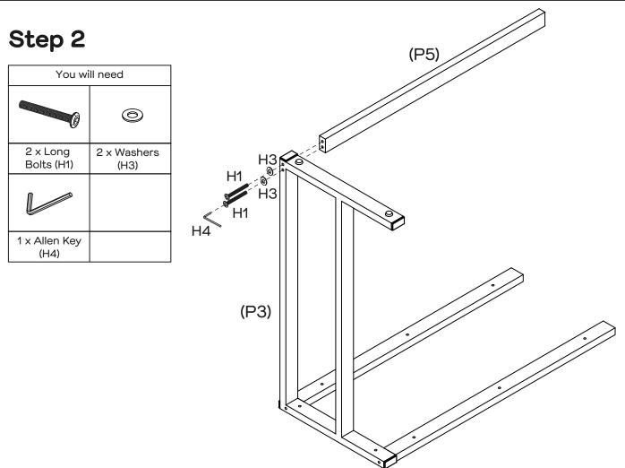
Attach Rail (P5) to Right Frame (P3) with  $2 \times \text{Long Bolts}$  (H1) and  $2 \times \text{Washers}$  (H3). Tighten the bolts using an Allen Key (H4).
