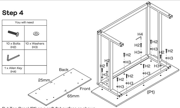
Put Top Panel (P1) on a soft flat surface as shown. Attach the frame to Top Panel (P1) with 10  $\times$  Bolts (H2) and 10  $\times$  Washers (H3) using an Allen Key (H4). Check and tighten all bolts.
