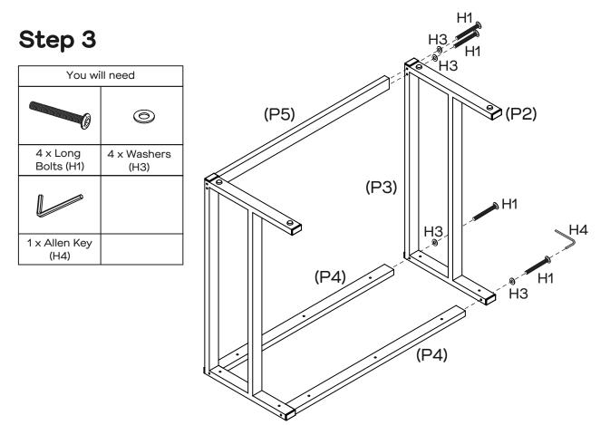
Attach Left Frame (P2) to Rails (P4, P5) with  $4 \times Long$  Bolts (H1) and  $4 \times Long$  Washers (H3). Tighten the bolts using an Allen Key (H4).
