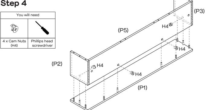
Insert 4 x Cam Nuts (H4) into the holes of Back Panel (P5) and Side Panels (P2, P3). Rotate the cam nuts so the arrows point towards the incoming cam bolts. Push Top Panel (P1) into place, then tighten the cam nuts using the Phillips Head Screwdriver.
