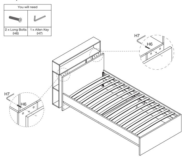
Attach the storage to bedhead with 2 x Long Bolts (H6) using Allen Key (H7).
