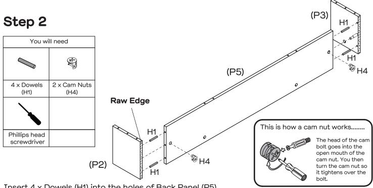
Insert 4 x Dowels (H1) into the holes of Back Panel (P5).
