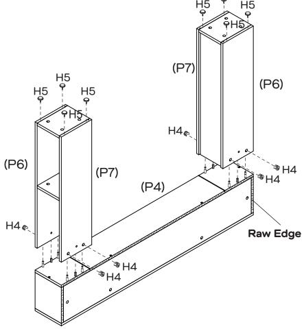
Insert 8 x Cam Nuts (H4) into the holes of Side Panels (P6, P7). Rotate the cam nuts so the arrows point towards the incoming cam bolts. Push the two frame into place, then tighten the cam nuts using the Phillips Head Screwdriver. Hammer 8 x Plastic Glides (H5) on the bottom of Side Panels (P6, P7) as shown.
