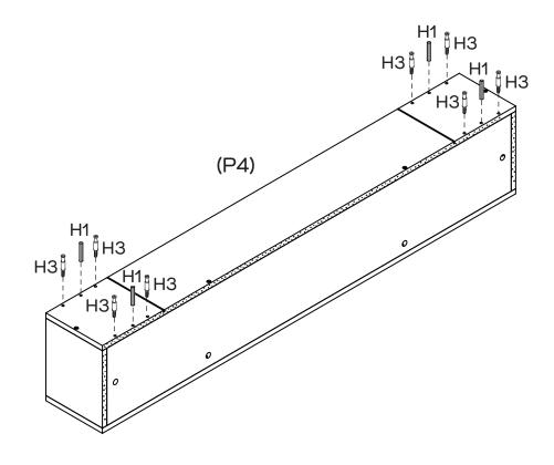
Insert 4  $\times$  Dowels (H1) into the holes of Bottom Panel (P4). Attach 8  $\times$  Cam Bolts (H3) into Bottom Panel (P4) as Shown.
