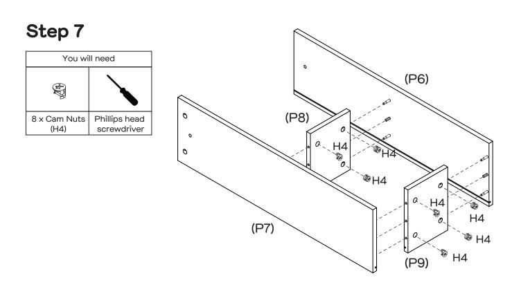
Insert 8  $\times$  Cam Nuts (H4) into the holes of Shelf Panels (P8, P9). Rotate the cam nuts so the arrows point towards the incoming cam bolts. Push Side Panels (P6, P7) into place, then tighten the cam nuts using the Phillips Head Screwdriver.
