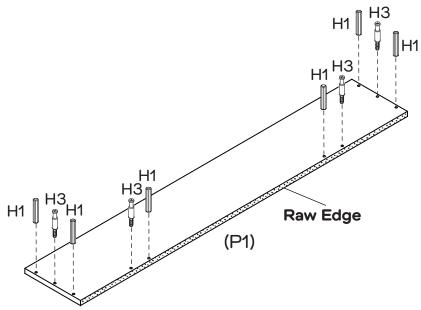
Insert 6 x Dowels (H1) into the holes of Top Panel (P1). Attach 4 x Cam Bolts (H3) into Top Panel (P1) as shown.
