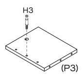
Attach 2 x Cam Bolts (H3) into Side Panels (P2, P3) as shown.
