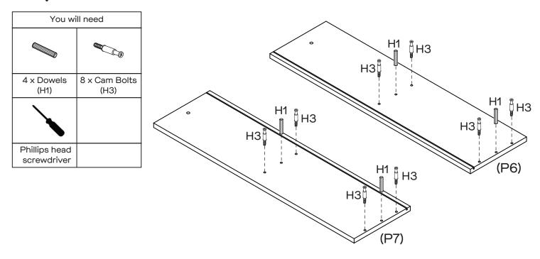
Insert 4 x Dowels (H1) into the holes of Side Panels (P6, P7). Attach 8 x Cam Bolts (H3) into Side Panels (P6, P7) as Shown.
