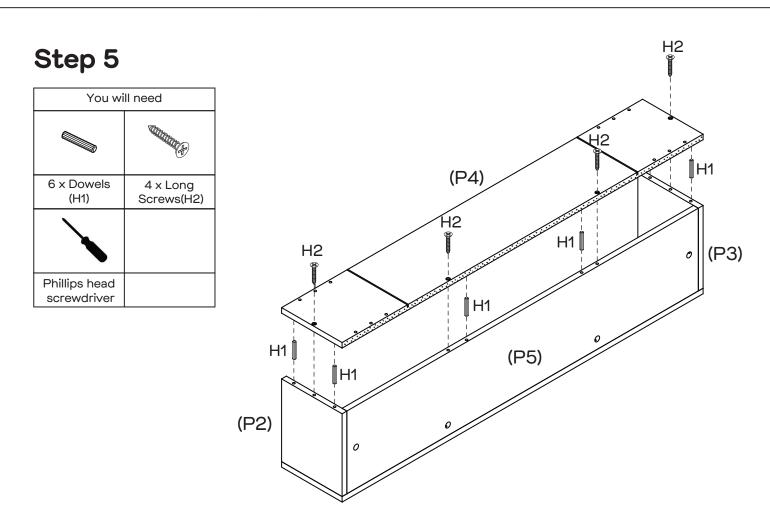
Insert 6 x Dowels (H1) into the holes of Side Panels (P2, P3) and Back Panel (P5). Attach Bottom Panel (P4) to the right place with 4 x Long Screws (H2) using a Philips head screwdriver.
