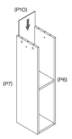
Put Back Panel (P10) into the grooves of Side Panels (P6, P7) as shown. Repeat Step 6 to Step 8 for the other Side Panels (P6, P7), Shelf Panels (P8, P9) and Back Panel (P10).
