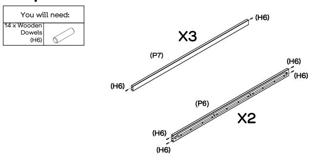
Insert 2 x Wooden Dowels (H6) into each roof bar (P7). Insert 4 x Wooden Dowels (H6) into each Side Rail (P6).
