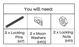
Screw 2 x Locking Pins (H7) to Legs (P3, P4). Attach Side Rail (P6) to Legs (P3, P4) by using 2 x Moon Washers (H10) and 2 x Locking Nuts (H11), tightening by Large Spanner (H8).
