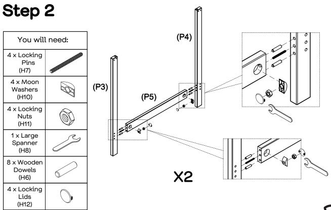
Insert 4 x Wooden Dowels (H6) and 2 x Locking Pin (H7) to Legs (P3, P4). Attach End Rail (P5) to legs (P3, P4) by using 2 x Moon Washers (H10) and 2 x Locking Nuts (H11), tightening by Large Spanner (H8). Put  $4 \times \text{Lids}$  (H12) on opening hole.
