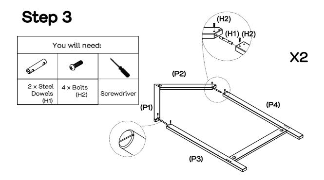
Insert 2 x Steel Dowels (H1) into the Legs and Rails (P1 and P3; P2 and P4). Attach 4 x Bolts (H2) by using a Phillips head screwdriver.
