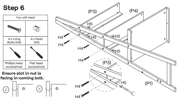
Insert 4 x Nuts (H5) into the holes on Shelf Panels (P3, P4), make sure the opening is facing incoming cam bolts. Push 4 x Long Bolts (H4) through Left Frame (P1), and connect with Shelf Panels (P3, P4) with 4 x Nuts (H5) using a Flat head screwdriver. Tighten the bolts with Phillips head screwdriver.
