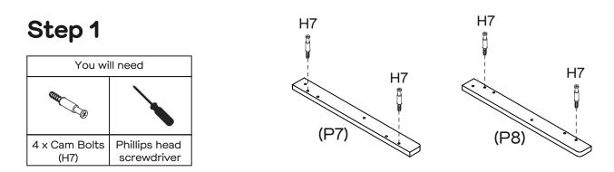
Attach 4 x Cam Bolts (H7) into Rails (P7, P8) with a Phillips head screwdriver.
