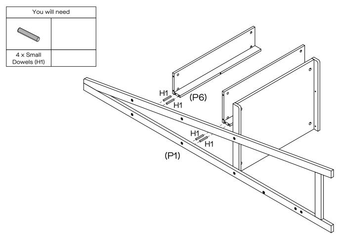
Insert 4 x Small Dowels (H1) into Rails (P6). Attach Shelf Panels (P3, P4) to Left Frame (P1) securely.
