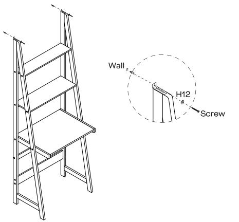
Move the bookcase to the final position, and attach the brackets to the wall securely. Make sure it is firmly attached and snug fit.
