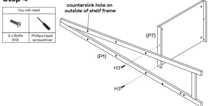
Attach Left Frame (P1) to Rail (P7) with 2 x Bolts (H3) using a Phillips head screwdriver.
