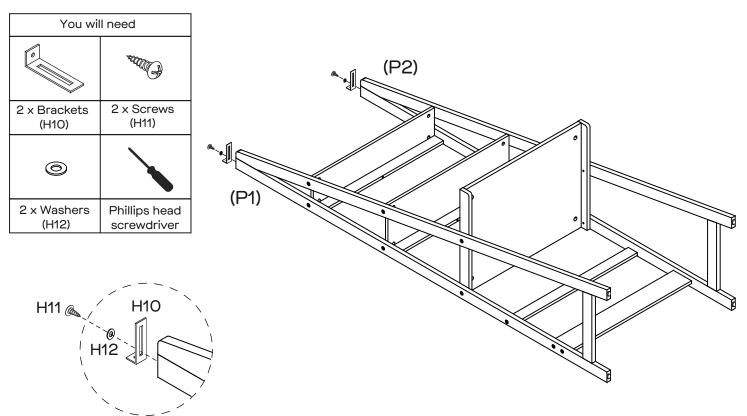
Attach 2 x Brackets (H1O) to the top of Frames (P1, P2) with 2 x Screws (H11) and 2 x Washers (H12), then tighten the screws with Phillips head screwdriver.
