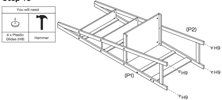
Carefully turn the frame over. Attach 4 x Plastic Glides (H9) to the bottom of Frames (P1, P2) with a Hammer.
