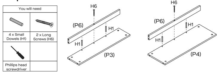
Insert 4 x Small Dowels (H1) into Shelf Panels (P3, P4). Attach Rails (P6) to Shelf Panels (P3, P4) with 2 x Long Screws (H6). Tighten Screws using a Phillips head screwdriver.
