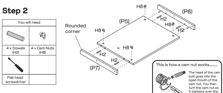
Insert 4 x Dowels (H2) into Shelf Panel (P5). Insert 4 x Cam Nuts (H8) into the holes of Shelf Panel (P5). Rotate the cam nuts so the arrows point towards the incoming cam bolts.
