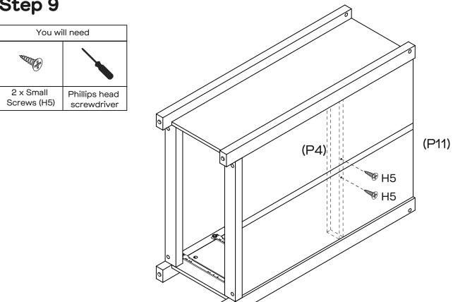
Use 2 x Small Screws (H5) to fix Back Panel (P11) onto Rail (P4). Tighten the screws with a Phillips head screwdriver.
