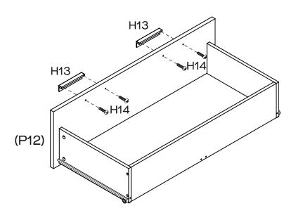
Attach 2 x Handles (H13) to Drawer Front (P12) with 4 x Round Head Bolts (H14). Tighten Round Head Bolts using a Phillips head screwdriver.
