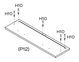
Screw  $5 \times Small Cam Bolts (H10) into Drawer Front (P12) with a Phillips head screwdriver.$
