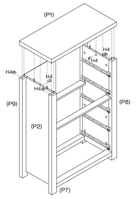
Insert 6 x Cam Nuts (H4) into the holes of Side Panels (P2, P3) and Legs (P7, P8, P9, P10). Rotate the cam nuts so the arrows point towards the incoming cam bolts.
