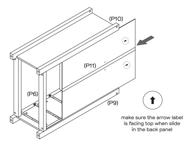
Slide Back Panel (P11) into the grooves of Legs (P9, P10) and Rail (P6).
