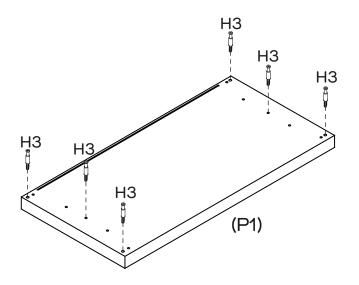
Attach 6 x Cam Bolts (H3) into Top Panel (P1) as shown.
