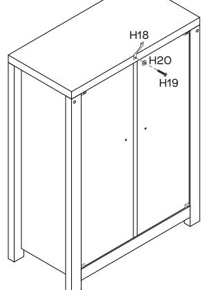
Use Screw (H19) and Washer (H20) to attach Safety Strap (H18) securely on Top Panel (P1) as shown. fantasticfurniture.com.au
