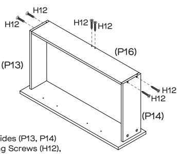
Attach Drawer Back (P16) to Drawer Sides (P13, P14) and Drawer Support (P17) with 6 x Long Screws (H12), make sure that the groove lines up the whole way around the drawer. Tighten Screws using a Phillips head screwdriver.
