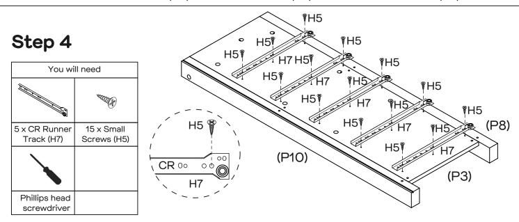
Attach 5 x CR Runner Tracks (H7) to Right Side Panel (P3) with 15 x Small Screws (H5).
