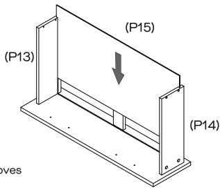
Slide Drawer Base (P15) into the grooves in Drawer Sides (P13, P14).
