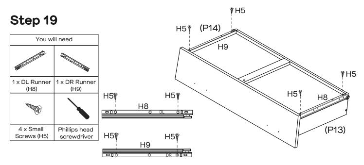
Attach 1 x DL Runner (H8) to the bottom of Left Drawer Side (P13) and 1 x DR Runner (H9) to the bottom of Right Drawer Side (P14) with 4 x Small Screws (H5). Tighten Screws using a Phillips head screwdriver.
