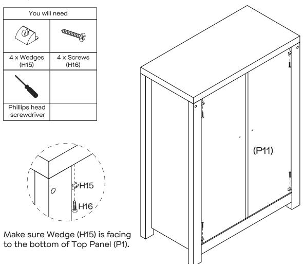
Secure Back Panel (P11) in place with  $4 \times \text{Wedges}$  (H15) using  $4 \times \text{Screws}$  (H16). Tighten the screws with a Phillips head screwdriver.
