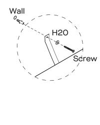
Move the tallboy to the final position, and attach the safety strap to the wall securely. Make sure it is firmly attached and snug fit.
