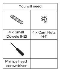
Insert 4 x Small Dowels (H2) into Left Side Panel (P2) and Legs (P7, P9). Insert 4 x Cam Nuts (H4) into the holes of Rails (P4, P5, P6). Rotate the cam nuts so the arrows point towards the incoming cam bolts.
