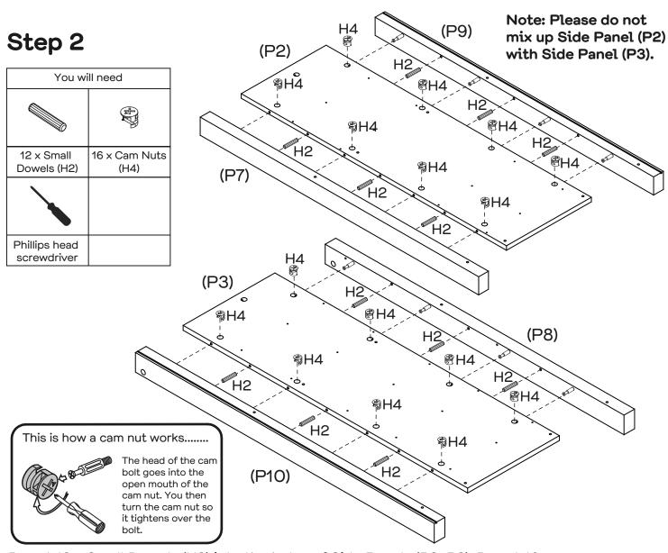
Insert 12 x Small Dowels (H2) into the holes of Side Panels (P2, P3). Insert 16 x Cam Nuts (H4) into the holes of Side Panels (P2, P3). Rotate the cam nuts so the arrows point towards the incoming cam bolts. Attach Legs (P7, P9) to Left Side Panel (P2) and Legs (P8, P10) to Right Side Panel (P3). Tighten the cam nuts using a Phillips head screwdriver.
