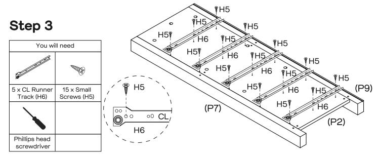
Attach 5 x CL Runner Tracks (H6) to Left Side Panel (P2) with 15 x Small Screws (H5).
