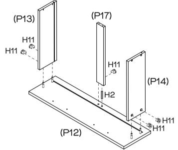
Insert 1 x Small Dowel (H2) into Drawer Front (P12) as shown.
