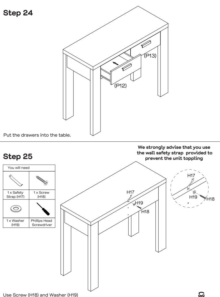
to attach Safety Strap (H17) securely on Top Panel (P1) as shown.
