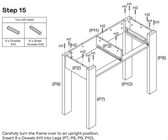
Insert 6 x Small Dowels (H2) into Side Panels (P2) and Divider (P3) as shown.
