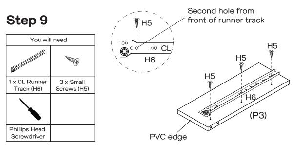
Turn Divider (P3) over to the other side. Attach 1 x CL Runner Track (H6) to Divider (P3) with 3 x Small Screws (H5).
