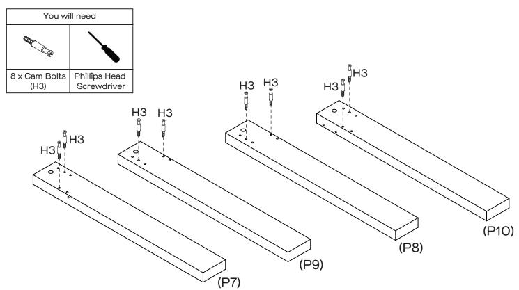
Insert 8 x Cam Bolts (H3) into the hole of Legs (P7, P8, P9, P10) as shown.
