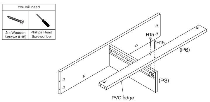
Attach Rail (P6) to Divider (P3) with 2  $\times$  Wooden Screws (H15) using a Phillips head screwdriver.
