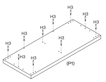
Insert 10 x Cam Bolts (H3) into the holes of Top Panel (P1) as shown.
