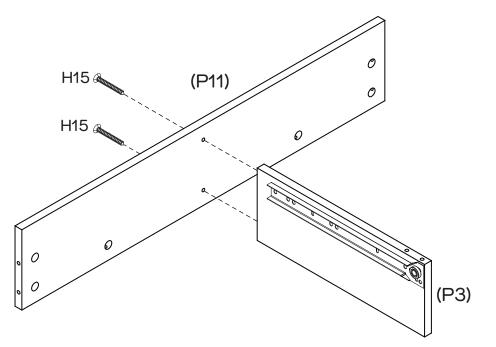
Attach Divider (P3) to Back Panel (P11) with 2 x Wooden Screws (H15) using a Phillips head screwdriver.
