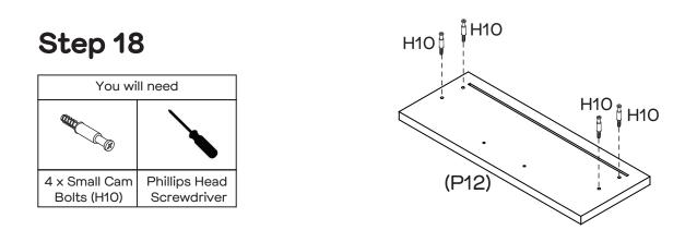
Screw 4 x Small Cam Bolts (H10) into Drawer Front (P12) with a Phillips head screwdriver.
