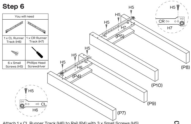
Attach 1 x CL Runner Track (H6) to Rail (P4) with 3 x Small Screws (H5). Attach 1 x CR Runner Track (H7) to Rail (P5) with 3 x Small Screws (H5).
