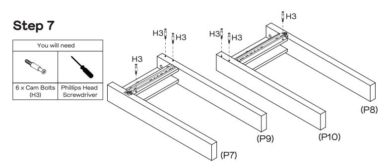
Insert 6 x Cam Bolts (H3) into the holes of Legs (P9, P10) and Rails (P4, P5) as shown.
