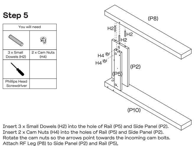
then tighten the cam nuts using a Phillips head screwdriver.
