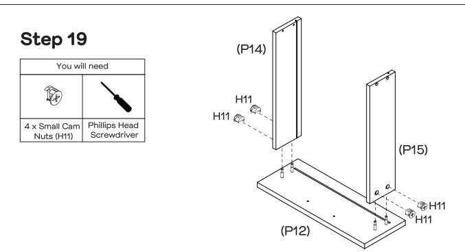
Insert 4 x Small Cam Nuts (H11) into the holes of Drawer Sides (P14, P15). Rotate the cam nuts so the arrows point towards the incoming cam bolts. Align the holes together, secure Drawer Sides (P14, P15) into place and tighten the cam nuts using a Phillips head screwdriver.
