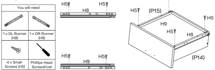
Attach 1 x DL Runner (H8) to the bottom of Left Drawer Side (P14) and  $1 \times DR$  Runner (H9) to the bottom of Right Drawer Side (P15) with  $4 \times Small Screws$  (H5). Tighten Screws using a Phillips head screwdriver.
