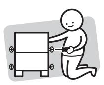
Unless instructed, do not fully tighten screws until the item is fully assembled.
