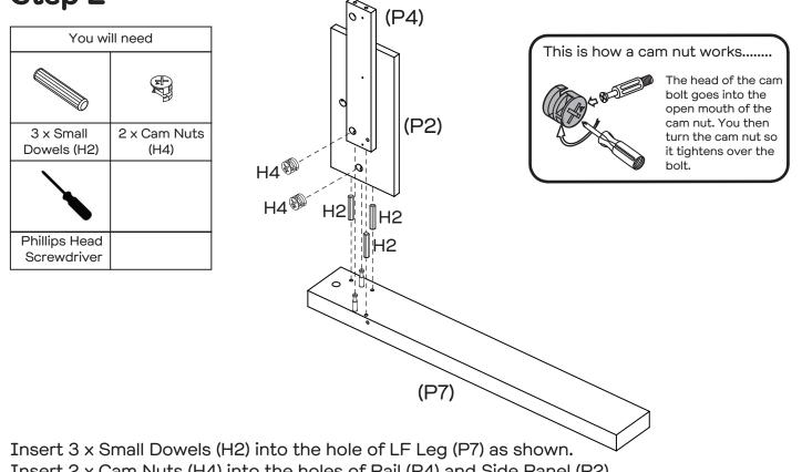
Insert 2 x Cam Nuts (H4) into the holes of Rail (P4) and Side Panel (P2). Rotate the cam nuts so the arrows point towards the incoming cam bolts. Attach Rail (P4) and Side Panel (P2) to LF Leg (P7), then tighten the cam nut.
