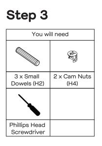
Insert 3 x Small Dowels (H2) into the hole of Rail (P4) and Side Panel (P2). Insert 2 x Cam Nuts (H4) into the holes of Rail (P4) and Side Panel (P2). Rotate the cam nuts so the arrows point towards the incoming cam bolts. Attach LR Leg (P9) to Side Panel (P2) and Rail (P4), then tighten the cam nut using a Phillips head screwdriver.
