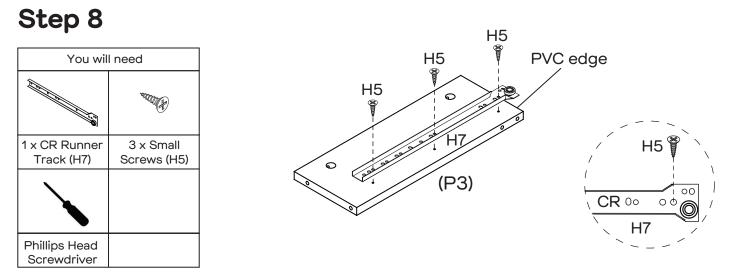
Attach 1 x CR Runner Track (H7) to Divider (P3) with 3 x Small Screws (H5).
