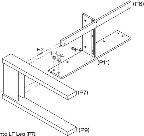
Insert 1 x Small Dowel (H2) into LF Leg (P7). Insert 3 x Cam Nuts (H4) into the holes of Rail (P6) and Back Panel (P11). Rotate the cam nuts so the arrows point towards the incoming cam bolts. Attach Rail (P6) and Back Panel (P11) into place. Tighten the cam nuts using a Phillips head screwdriver.
