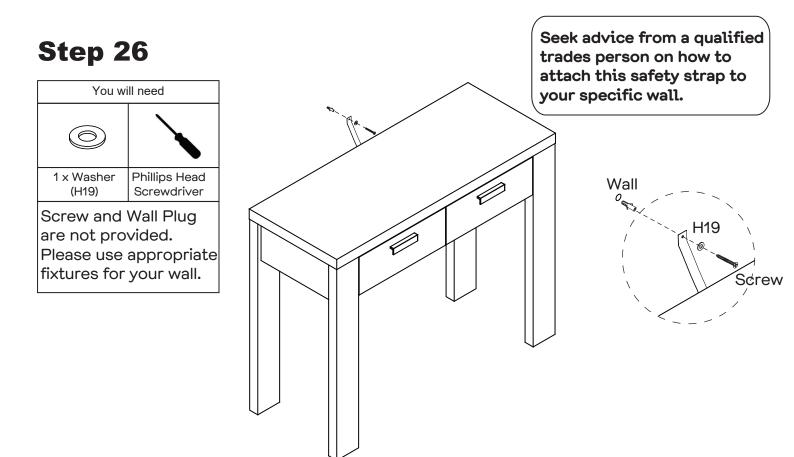
Move the table to the final position, and attach the safety strap to the wall securely. Make sure it is firmly attached and snug fit.
