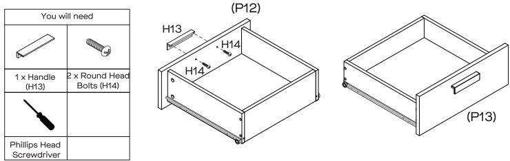
Attach 1 x Handle (H13) to Drawer Front (P12) with 2 x Round Head Bolts (H14). Tighten round head bolts using a Phillips head screwdriver. Repeat Step 18 to Step 23 with Drawer Front (P13) to assemble the other drawer.
