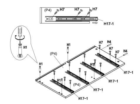
Insert 2 x Big Wood Dowels (H4) into Right Side Panel (P4). Screw 4 x Big Cam Bolts (H1) into Right Side Panel (P4). Attach 4 x the Separated Slide Tracks (H17-1) onto Right Side Panel (P4) with 12 x Screws (H7).
