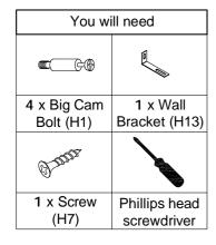
Screw 4 x Big Cam Bolts (H1) into Top Panel (P1) as shown.
