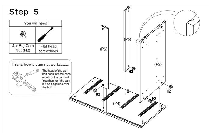
Position Bottom Panel (P2) over Right Side Panel (P4) so that their grooves are aligned. Fit Bottom Panel (P2), Front Rail (P5) & Back Rail (P6) to Right Side Panel (P4). Insert 4 x Big Cam Nuts (H2) into Back Rail (P6), Front Rail (P5) and Right Side Panel (P4) and turn lockwise to lock.
