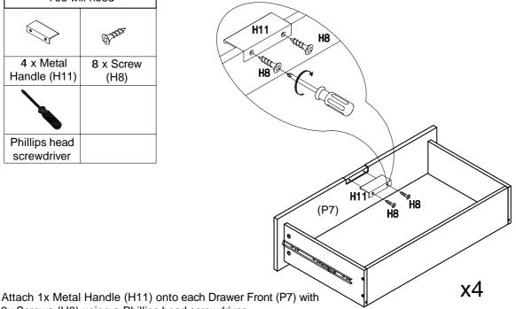
2x Screws (H8) using a Phillips head screwdriver.
