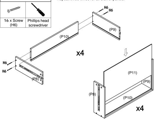
Slide 1x Drawer Base (P11) into the grooves in the Drawer Panels (P8), (P9) and (P10). Repeat three times for all Drawer Bases (P11).
