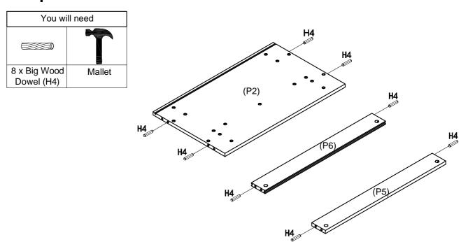
Insert 4 x Big Wood Dowels (H4) into Bottom Panel (P2). Insert 2 x Big Wood Dowels (H4) into Front Rail (P5). Insert 2 x Big Wood Dowels (H4) into Back Rail (P6).
