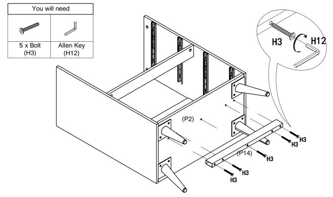
Attach Metal Bar (P14) onto Bottom Panel (P2) with  $5 \times 80$  using Allen Key (H12). With help, carefully turn the assembled unit over.
