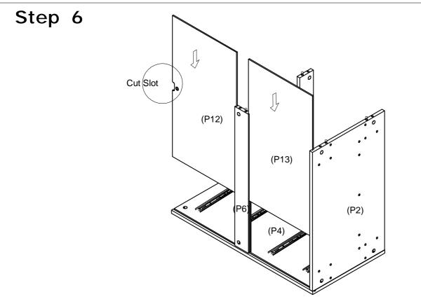
Slide Lower Back Panel (P13) & Upper Back Panel (P12) into grooves as shown.
