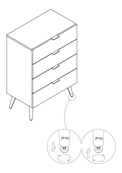
If the Tallboy is not level, you can adjust the height of each Leg by turning the feet of Legs clockwise or counter-clockwise.
