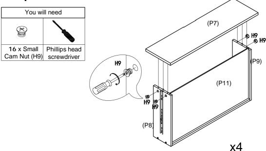
Position Drawer Front (P7) onto Drawer Sides (P8) & (P9). Rotate 1x Small Cam Nut (H9) so the arrow points towards the incoming cam bolt and insert the Small Cam Nut (H9) into Drawer Side Panel (P8) or (P9). Repeat with the remaining 3 x Small Cam Nut (H9). Turn Small Cam Nuts (H9) clockwise to lock.
