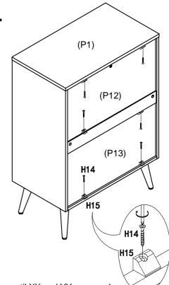
If necessary, gently adjust the Top Panel (P1) sideway in either direction until XX and YY are equal.
