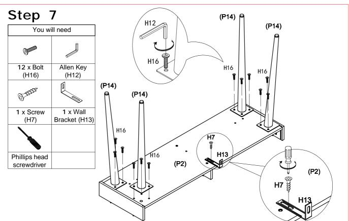
Fix each Metal Leg (P14) onto Bottom Panel (P2) with 3 x Bolts (H16) using Allen Key (H12). Fasten Wall Bracket (H13) onto Bottom Panel (P2) with Screw (H7) as shown. Do not fully tighten the Screw (H7).
