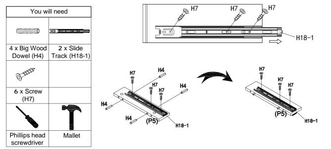
Insert 4 x Big Wood Dowels (H4) into Divider Panel (P5).
