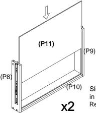
Slide 1x Drawer Base (P11) into the grooves in the Drawer Panels (P8), (P9) and (P10). Repeat with the other Drawer Base (P11).
