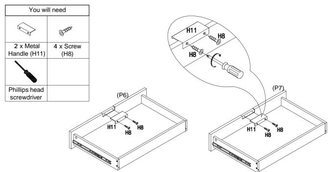
Attach 1x Metal Handle (H11) onto each Drawer Front (P6) or (P7) with 2x Screws (H8) using a Phillips head screwdriver. Do not over-tighten the screws (H8).
