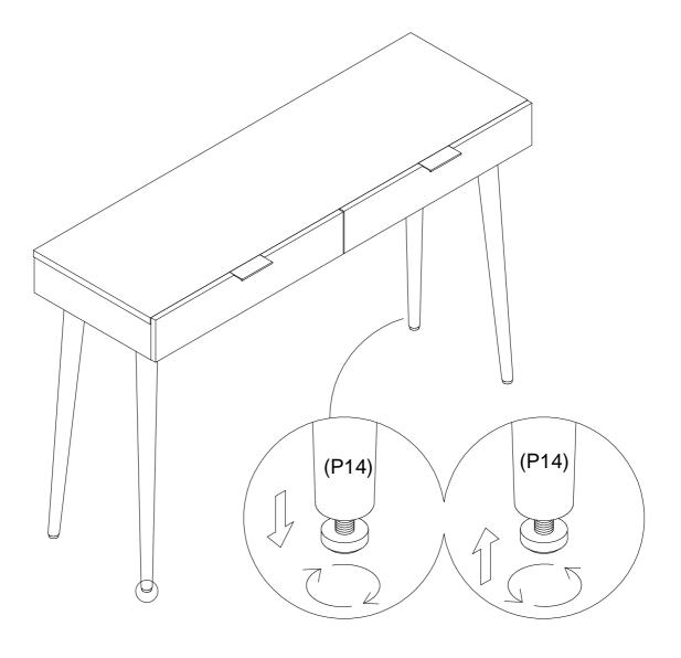
If the Hall Table is not level, you can adjust the height of each Leg by turning the feet of Legs clockwise or counter-clockwise.
