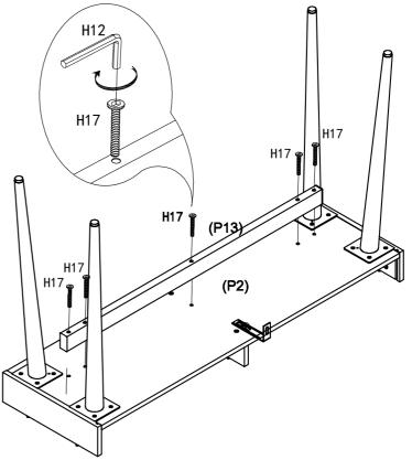
Attach Metal Bar (P13) onto Bottom Panel (P2) with  $5 \times 80$  using Allen Key (H12). With help, turn the assembled unit over carefully.
