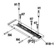
Screw 2 x Big Cam Bolts (H1) into Right Side Panel (P4). Attach 1 x Slide Tracks (H18-1) onto Right Side Panel (P4) with 3 x Screws (H7).
