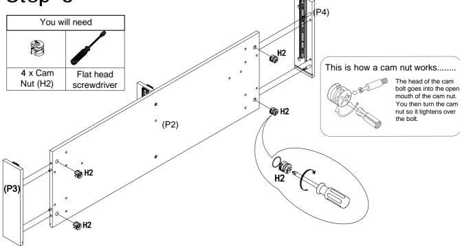
Position Left Side Panel (P3) and Right Side Panel (P4) onto Bottom Panel (P2), so that their grooves are aligned.
