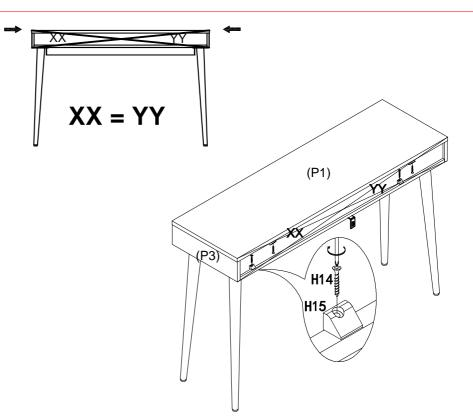
If necessary, gently adjust the Top Panel (P1) sideway in either direction until XX and YY are equal. Fix the Back Panel Connectors (H15) with Screws (H14) as shown.
