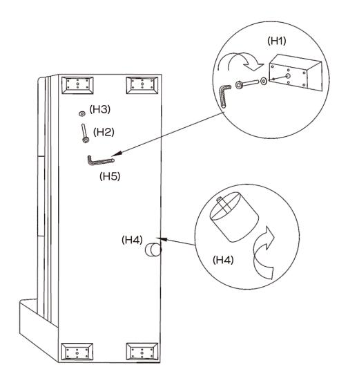
Attach  $4 \times legs$  (H1) and  $1 \times support leg$  (H4) into position as shown with  $4 \times bolts$  (H2) and  $4 \times washers$  (H3) with the allen key (H5).
