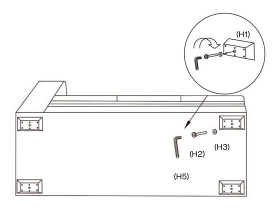
Attach  $4 \times legs$  (H1) into position as shown with  $4 \times bolts$  (H2) and  $4 \times washers$  (H3) with the allen key (H5).
