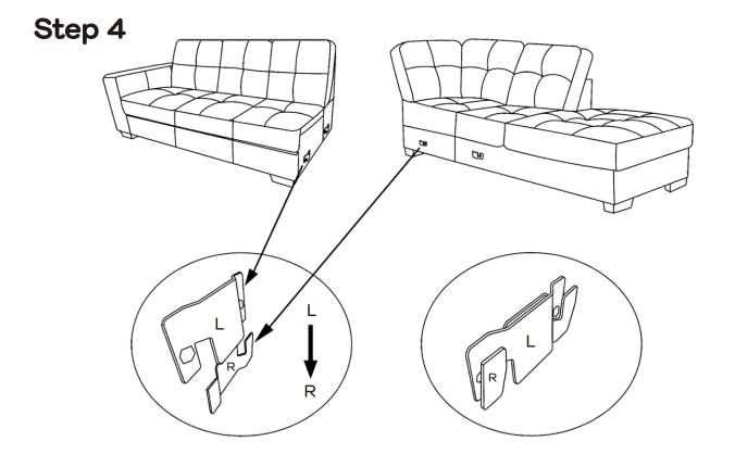
Align the clips and join the 2 pieces together.
