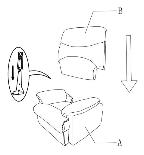
Attach seat back(B) to seat base(A) ,well align clips on two sides before inserting the back, ensure the clips are secured.
