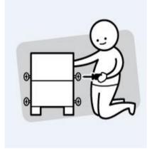
Unless instructed, do not fully tighten screws until the item is fully assembled.
