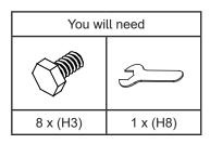
Attach legs (P2) to center block (P3) using bolts (H3) and wrench (H8). Be aware to only tighten bolts 80%
