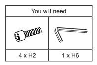
Attach legs (P2) to top (P1) by using 4 x bolts (H2) and allen key (H6), tighten all bolts (H2) 80%.
