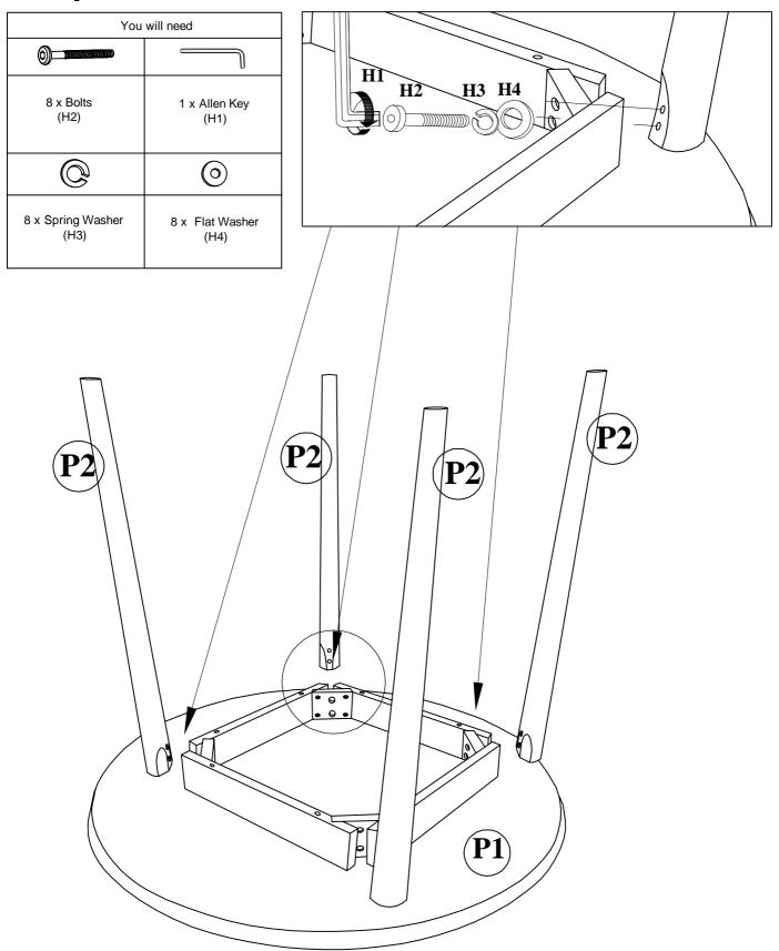
Attach table legs (P2) table top (P1) using Bolts (H2) and Washers (H3) & (H4). Note : Do not tighten bolts until table is on flat surface
