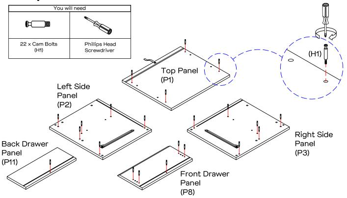
Insert 22 x cam bolts (H1) to panels as shown. Secure by tightening cam bolts (H1) with a phillips head screwdriver.
