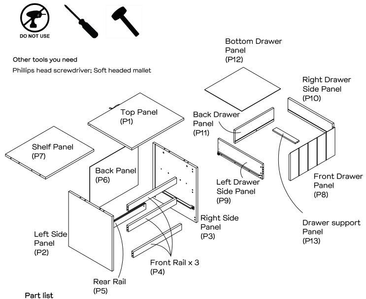
Top Panel (P1), Left Side Panel (P2), Right Side Panel (P3), Front Rails (P4), Rear Rail (P5), Back Panel (P6), Shelf Panel (P7), Front Drawer Panel (P8), Left Drawer Side Panel (P9), Right Drawer Side Panel (P10), Back Drawer Panel (P11), Bottom Drawer Panel (P12), Drawer Support Panel (P13), Hardware pack.
