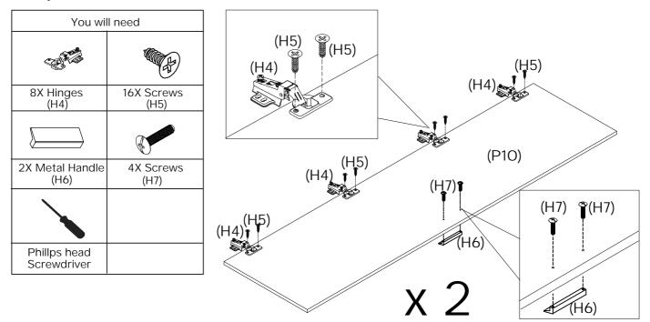
Fix 4 x Hinges (H4) to Door Panel (P10) using 8 x Screws (H5) by tightening with the Phillps Head Screwdriver.
