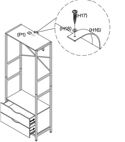
Attach the Wall Strap (H16) to Top Panel (P1) with  $1 \times$  Washer (H18) and  $1 \times$  Wall Strap Screw (H17) by tightening with the Phillips Head Screwdriver.
