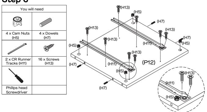
Attach 2 x CR Runner Tracks (H11) to Right Side Panel (P12) with 8 x Screws (H13) as shown by tightening with the Phillips Head Screwdriver.
