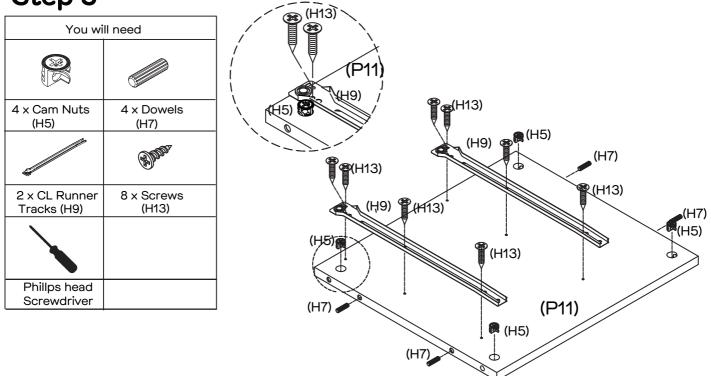
Attach 2 x CL Runner Tracks (H9) to Left Side Panel (P11) with 8 x Screws (H13) as shown by tightening with the Phillips Head Screwdriver.
