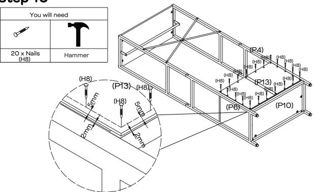
Secure Back Panel (P13) to the back of the partially assembled drawer unit as shown with 20 x Nails, approximately 5mm from the edge, using the Hammer. Ensure the Fantastic Furniture Back Panel is sitting square in the unit before securing, with about 2mm around each edge.
