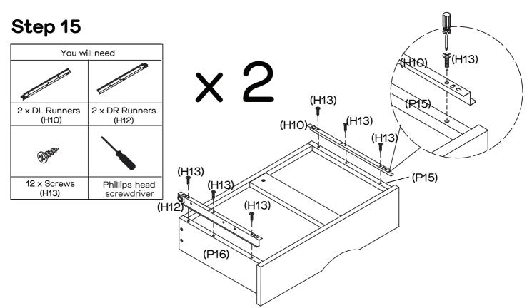
Secure 1 x DL Runner (H10) to Drawer Left Side Panel (P15) and 1 x DR Runner (H12) to Drawer Right Side Panel (P16) as shown with 6 x Screws (H13) by tightening with the Phillips Head Screwdriver.
