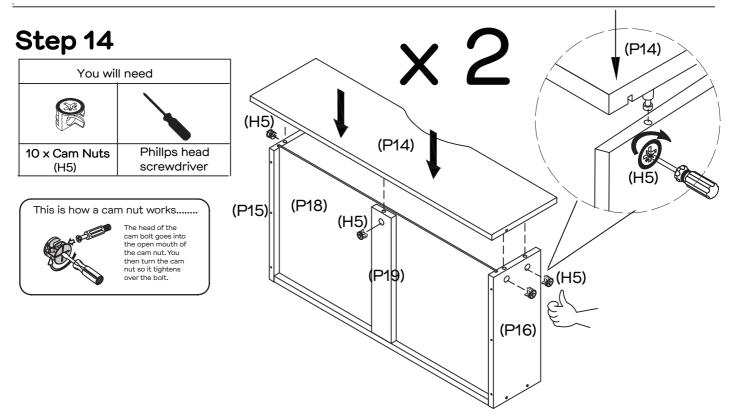
Insert 5 x Cam Nuts (H5) into Left & Right Drawer Sides (P15&P16) and Drawer Support Panel (P19) as shown. Rotate the Cam Nuts so the arrows point towards the incoming Cam Bolts. Secure the Drawer Front (P14) to Drawer Left & Right Side Panels (P15&P16) and Drawer Support Panel (P19) as shown by tightening 5 x Cam Nuts (H15) with the Phillips Head Screwdriver.
