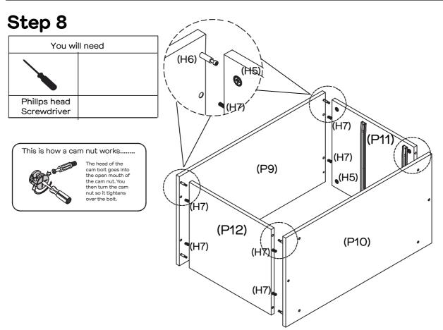
Rotate the Cam Nuts so the arrows point towards the incoming Cam Bolts. Secure the Drawer Top Panel (P9) and Base Panel (P10) to Left & Right Side Panels (P11&P12) as shown by tightening 8 x Cam Nuts (H5) with the Phillips Head Screwdriver. fantasticfurniture.com.au
