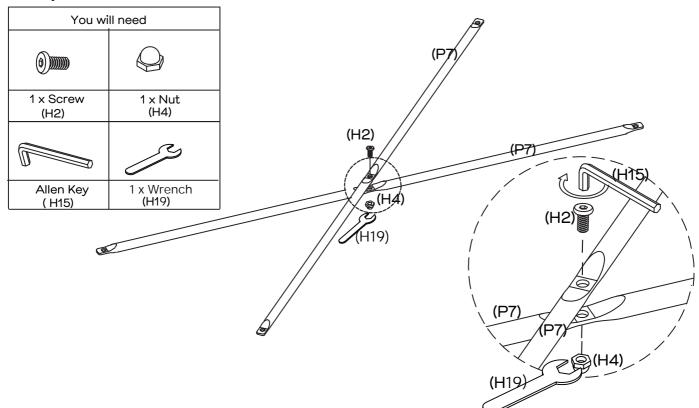
Secure Back Supports (P7x2) together as shown with 1 x Nut (H4) and 1 x Screw (H2) by tightening with the Allen Key (H15) and Wrench (H19).
