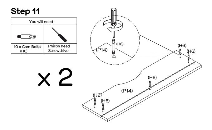
Secure 5 x Cam Bolts (H6) to Drawer Front (P14) by tightening with the Phillips Head Screwdriver.
