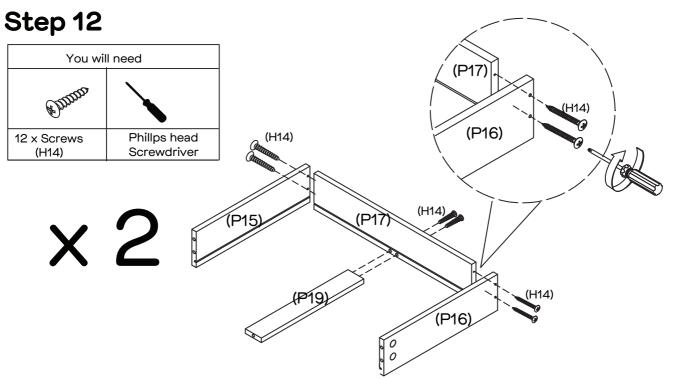
Secure Left & Right Drawer Sides (P15&P16) to Back Panel (P17) with 4 x Screws (H14) by tightening with the Phillips Head Screwdriver. Attach Drawer Support Panel (P19) to Back Panel (P17) with 2 x Screws (H14) by tightening with the Phillips Head Screwdriver. Repeat steps for the second Drawer.
