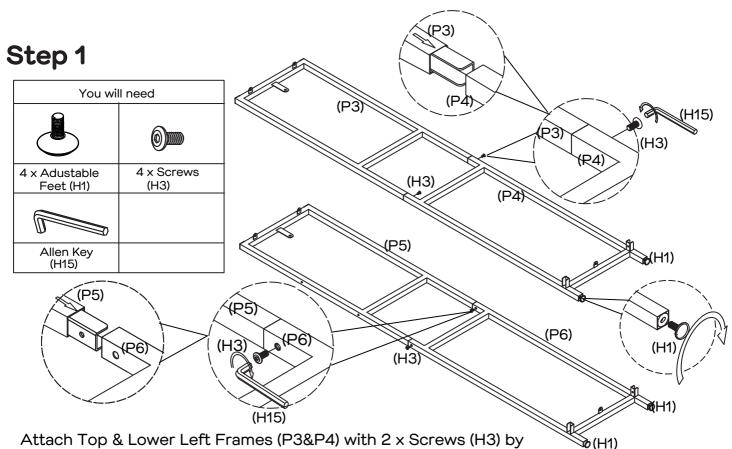
tightening with the Allen Key (H15).
