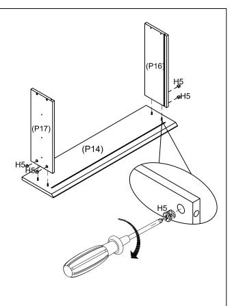
Position the 2 x Drawer Left Side (P16) and 2 x Drawer Right Side (P17) to the Drawer Front (P14,P15),insert 8 x Small Cam Nut (H5) into the holes on Panel (P16,P17) as shown, make sure the opening on cam nut is facing incoming cam bolts, turn clockwise to lock.
