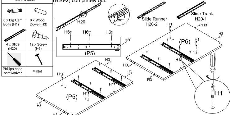
Insert 8 x Dowel (H3) onto the Middle Side Panel (P5,P6). Screw 6 x Big Cam Bolt (H1) onto the Middle Side Panel (P5,P6).By using a Phillip Head Screwdriver,attach 4 x Slide Track (H20-1) onto the Middle Side Panel(P5,P6) by using 12 x Screw (H6).
