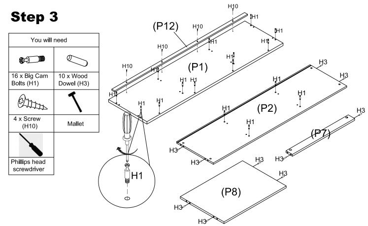
Using a mallet if needed, Insert 10 x Dowel (H3) onto the Bottom Panel (P2) and Middle Rail (P7) and Middle Shelf Panel (P8).
