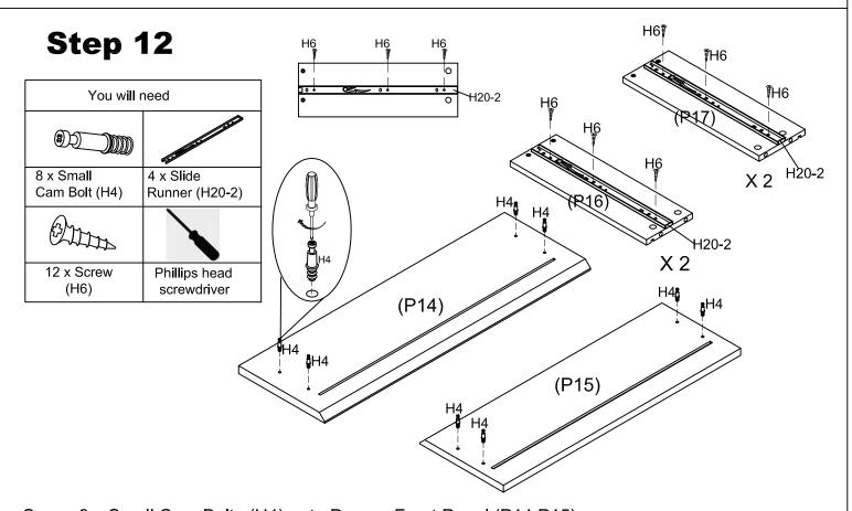
Screw 8 x Small Cam Bolts (H4) onto Drawer Front Panel (P14,P15) Attach 4 x Slide Runner (H20-2) to Drawer Side Panel (P16,P17) by using 12 x Screw (H6) as shown.
