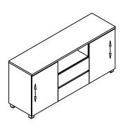
STEP 19.2 Adjust the door panels upward or downward
