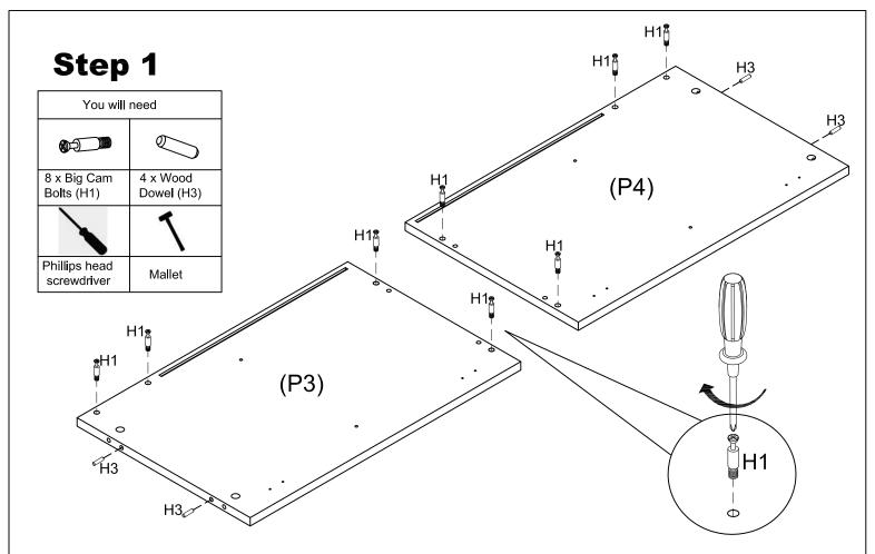
Using a mallet if needed, Insert 4 x Dowel (H3) onto the Left Side Panel (P3) and Right Side Panel (P4). Screw 8 x Big Cam Bolt (H1) onto the Left Side Panel (P3) and Right Side Panel (P4).
