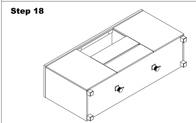
If the floor is uneven, please twist the adjustable leg to stabilize the unit.
