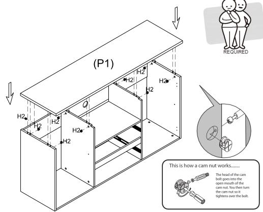
Position the Top Panel (P1) to the Left Side Panel (P3) and Right Side Panel (P4) and Middle Side Panel (P5,P6) and Back Rail (P10).
