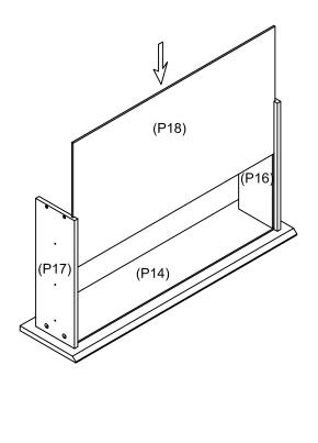
Insert the Drawer Bottom Panel (P18) into the grooves of the Drawer Front (P14,P15) and Drawer Left side Panel (P16) and Drawer Right side Panel (P17).
