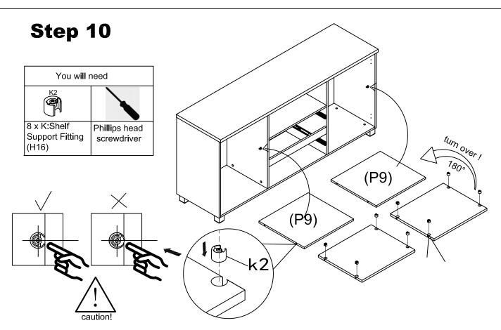
Insert 8 x Shelf Support Fitting (H16-K2) onto the Shelf Panel (P9) make sure the opening on Shelf Support Fitting is facing to the panel edge. Turn the panel down then position to the Shelf Support Fitting (H16-K1).
