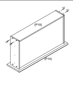
Screw the 2 x Drawer Back Panel (P19) to the Drawer Left Side (P16) and Drawer Right Side (P17) by using 8 x Screw (H7).
