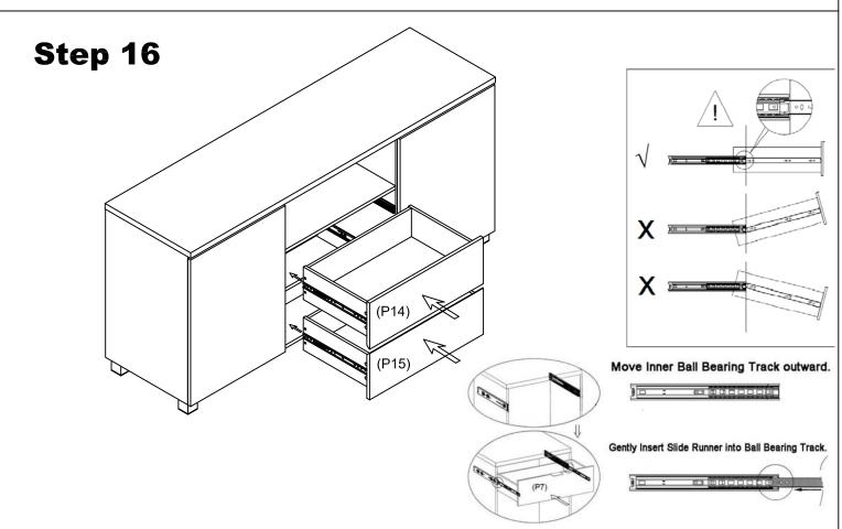
Position Drawer so that Slide Runner (H20-2) aligns with Slide Track (H20-1) as shown Gently push drawer into the closed position.
