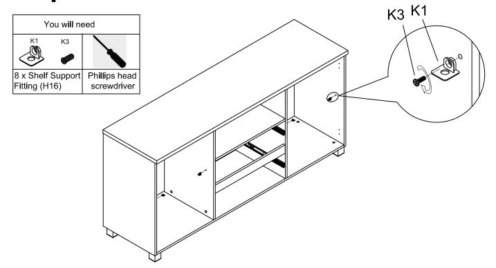
Insert 8 x Shelf Support Fitting (H16-K1) onto the Left Side Panel (P3) and Right Side Panel (P4) and Middle Side Panel (P5,P6) by using 8 x Shelf Support Fitting (H16-K3).
