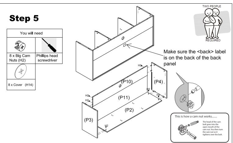
Position the Side Panel (P3,P4) to the Bottom Panel (P2) and Back Rail (P10) and Back Panel (P11). Insert the 8 x Big Cam Nuts (H2) to the Bottom Panel (P2) and Back Rail (P10) make sure the opening on nuts is facing incoming cam bolt, turn clockwise to lock. Insert the 8 x Covers (H14) onto the Big Cam Nut (H2).
