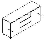
STEP 19.4 Adjust the gap between door panel and side panel
