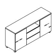
STEP 19.3 Adjust the flush between door panel and side panel
