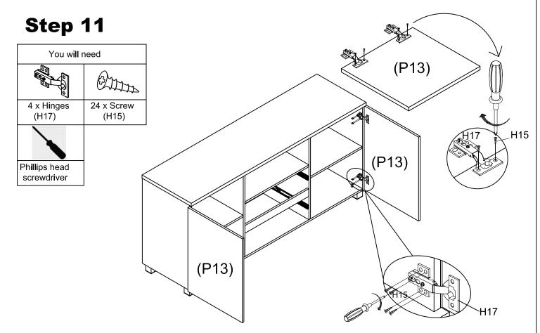
Attach 4 x Hinges (H17) onto the Door Panel (P13) by using 8 x Screw (H15).then attach 4 x Hinges (H17) to the Side Panel (P3,P4) by using 16 x Screw (H15).
