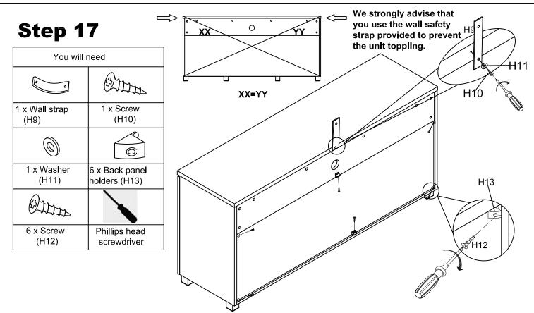
If necessary, gently adjust the Top Panel (P1) sideway in either direction untill XX and YY are equal Slide 6 x Back Panel holders (H13) into the grooves as shown. Insert 6 x Screw (H12) to fix them into place. Tighten the Screw (H12) with a Phillips Head Screwdriver Tighten the Wall Strap (H9) to the Top Panel (P1) with Screw (H10) and Washer (H11).
