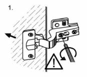
MOVE DOOR OUTWARD by turning this screw counter-clockwise
