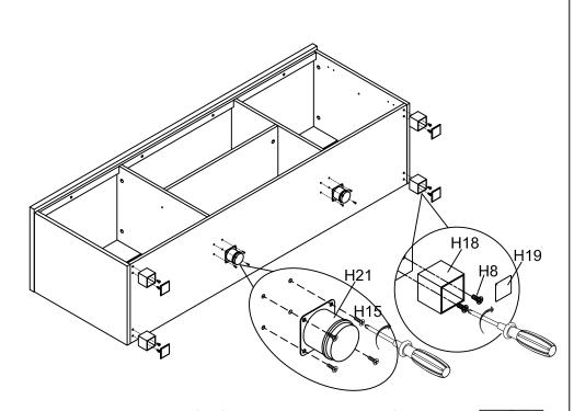
Attach 4 x Leg (H18) to Bottom Panel by using 8 x Bolt (H8), then insert 4 x Leg Cap (H19) onto Leg (H18). attach 2 x Leg (H21) to Bottom Panel by using 8 x Screw (H15).
