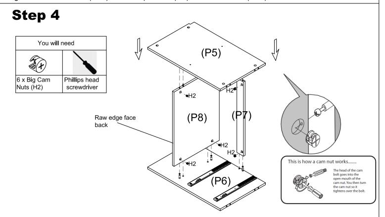
Position the Middle Panel (P5,P6) to the Middle Shelf Panel (P8) and Middle Rail (P7). Insert the 6 x Big Cam Nuts (H2) to the Panel (P7,P8) make sure the opening on nuts is facing incoming cam bolt,turn clockwise to lock.
