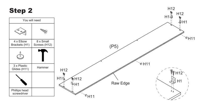
Attach 4 x Elbow Brackets (H1) to Base Panel (P5) with 8 x Small Screws (H12). Then hammer 3 x Plastic Glides (H11) on the bottom of Base Panel (P5).
