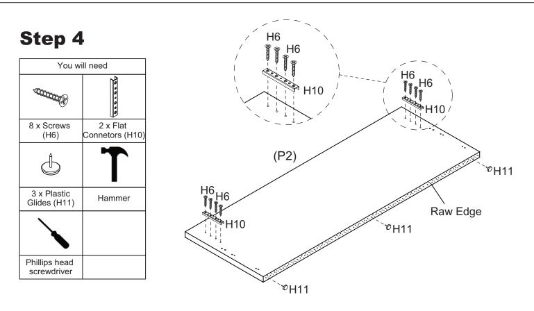
Attach 2 x Flat Connectors (H10) to Bedfoot (P2) with 8 x Screws (H6). Then hammer 3 x Plastic Glides (H11) on the bottom of Bedfoot (P2). www.fantasticfurniture.com.au
