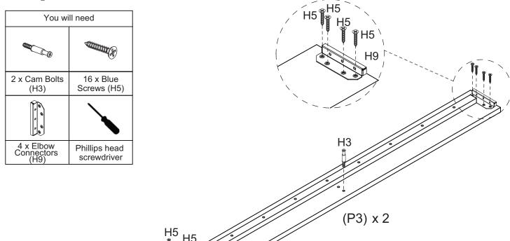
Attach 1 x Cam Bolt (H3) to each Side Rail (P3). Attach 2 x Elbow Connectors (H9) to each Side Rail (P3) with 8 x Blue Screws (H5).
