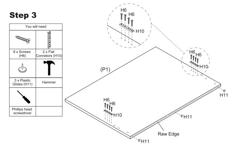
Attach 2 x Flat Connectors (H10) to Bedhead (P1) with 8 x Screws (H6). Then hammer 3 x Plastic Glides (H11) on the bottom of Bedhead (P1).
