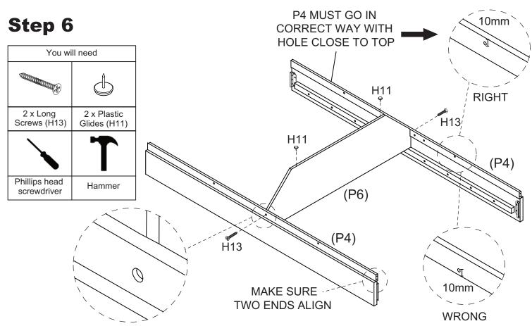
Attach Rails (P4) to Clapboard (P6) with 2 x Long Screws (H13). Then hammer 2 x Plastic Glides (H11) on the bottom of Clapboard (P6).
