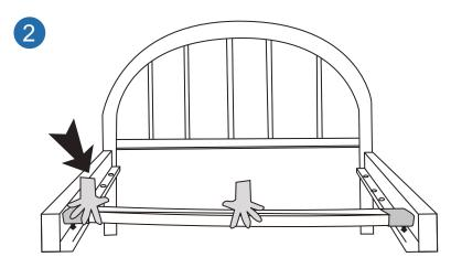
Place the slat in position then push down in the centre to flatten. Make sure the plastic prong lines up with the hole, then push in firmly.
