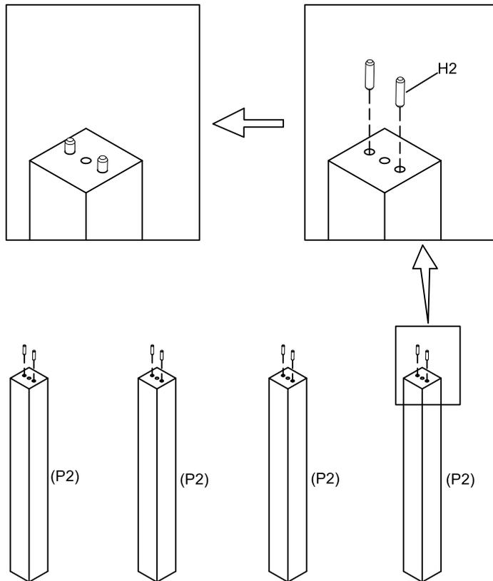
Using a Mallet if needed, Insert 8 x Wood Dowels (H2) to the hole on Leg (P2) as shown.
