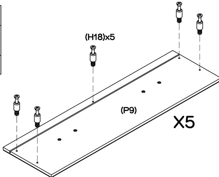
Attach 5 x small cam bolts (H18) to 1 x drawer front (P9) using a phillips head screwdriver. Repeat this step for the other 4 x drawer fronts (P9).
