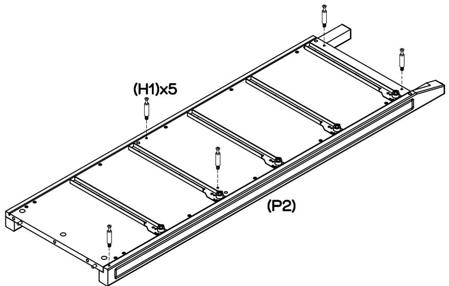
Attach 5 x large cam bolts (H1) into left side (P2) using a phillips head screwdriver.
