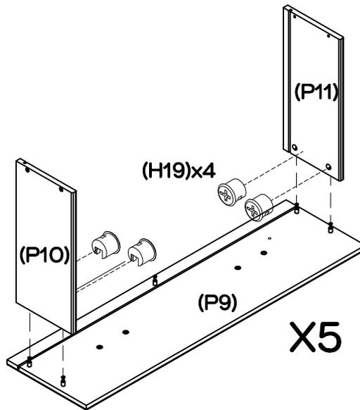
Attach 1 x drawer left side (P10) and 1 x drawer right side (P11) to 1 x drawer front (P9), ensuring the grooves on all the panels align. Insert 4 x small cam nuts (H19) into the drawer sides (P10,P11). Using a phillips head screwdriver, rotate the cam nuts so the arrow points towards the incoming cam bolts. Turn clockwise to lock. Repeat this process for the other 5 x drawer side panels (P10, P11).
