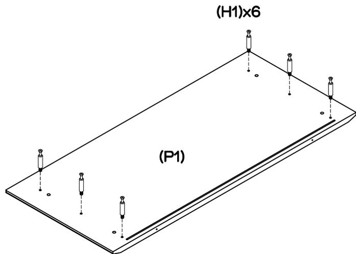
Attach 6 x large cam bolts (H1) to top panel (P1) using a phillips head screwdriver.
