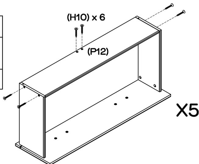
Attach 1 x drawer back panel (P12) to the side panels (P10, P11) and drawer support rail (P14) using 6 x medium screws (H10), tightening with a phillips head screwdriver. Repeat this process for the other 4 x drawer back panels (P12).
