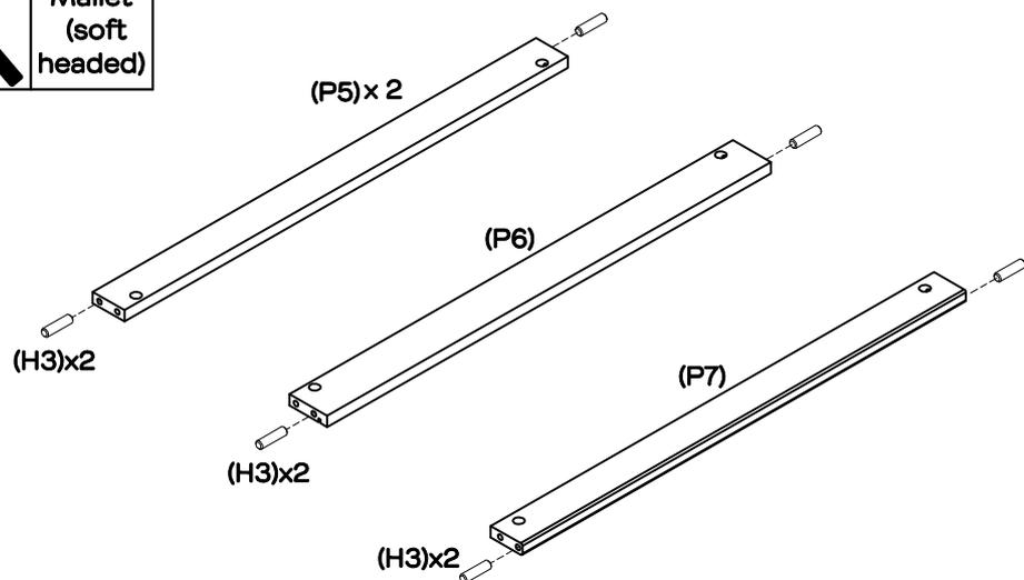
Insert 8 x wooden dowels (H3) into 2 x middle rails (P5), rear lower rail (P6) and front lower rail (P7).
