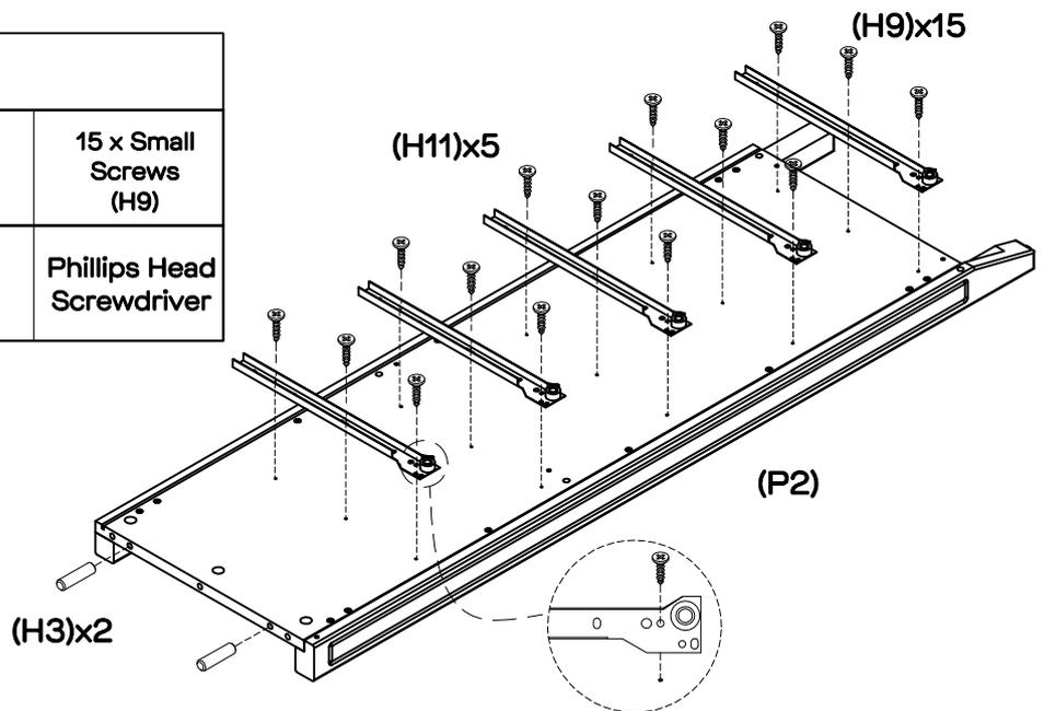
Insert 2 x wooden dowels (H3) into left side (P2). Attach 5 x left runner tracks (H11) to left side (P2) using 15 x small screws (H9), tightening using a phillips head screwdriver. Ensure the screws are inserted into the holes on the tracks (H11) as shown above.
