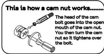
Attach top panel (P1) to unit as shown. Insert 6 x large cam nuts (H2) into the left and right side (P2, P3). Using a phillips head screwdriver, rotate the cam nuts (H2) so the arrow points towards incoming cam bolts. Turn clockwise to lock.
