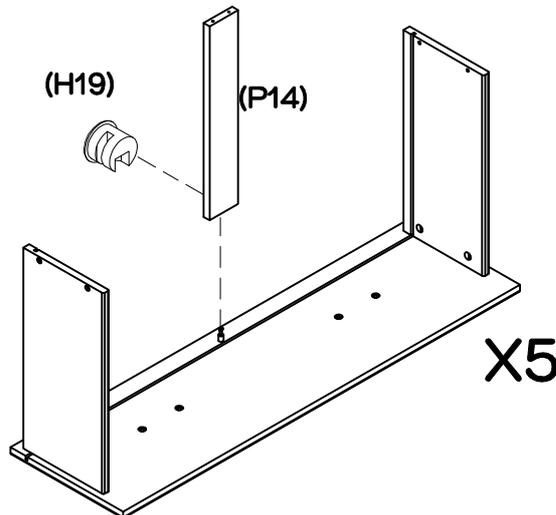
Attach 1 x drawer support rail (P14) to 1 x drawer front (P9), ensuring the side with the cam nut holes faces outwards. Insert 1 x small cam nut (H19) into the drawer support rail (P14). Using a phillips head screwdriver, rotate the cam nut so the arrows faces incoming cam bolt. Turn clockwise to lock. Repeat this process for the other 4 x support rails (P14).
