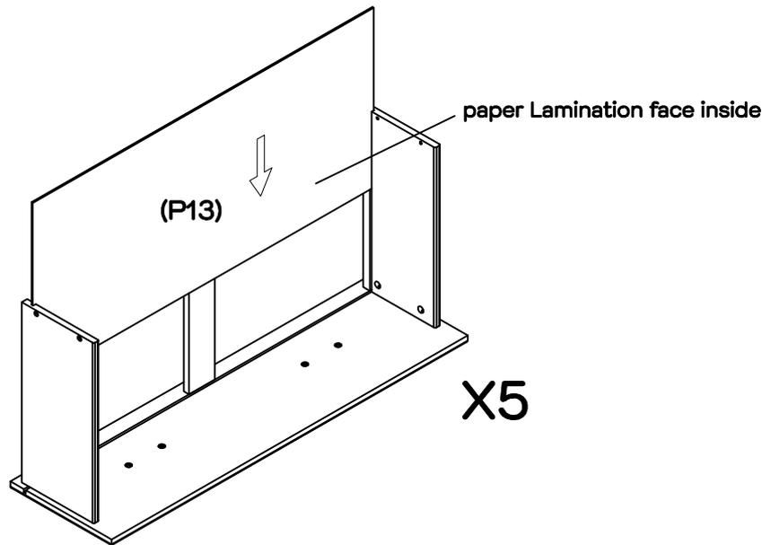
Slide 1 x drawer base (P13) into the grooves on the drawer sides (P10, P11) and drawer front (P9). Repeat this process for the other 4 x drawer bases (P15).
