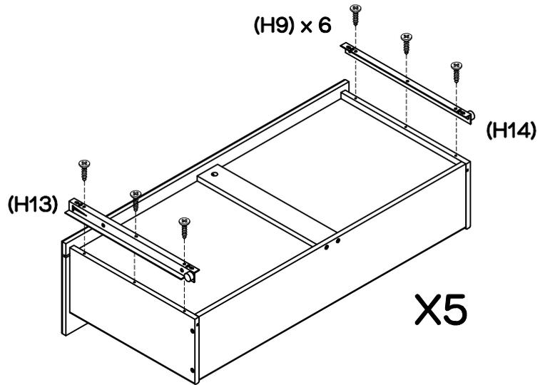
Attach 1 x left runner (H13) to the left drawer side (P10) and 1 x right runner (H14) to the right drawer side (P11) using 6 x small screws (H9), tightening with a phillips head screwdriver. Repeat this process for the other 4 x assembled drawers.
