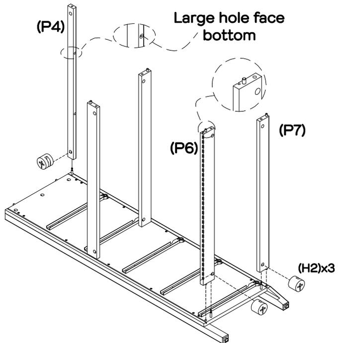
Attach front upper rail (P4) to right side (P3), ensuring the side with the cam nut hole faces inwards. Attach the rear lower rail (P6) and front lower rail (P7) to right side (P3), ensuring the sides with the cam nut holes faces outwards. Insert 3 x large cam nuts into the rails (P4, P6, P7). Using a phillips head screwdriver, rotate the cam nuts (H2) so the arrow points towards incoming cam bolts. Turn clockwise to lock.
