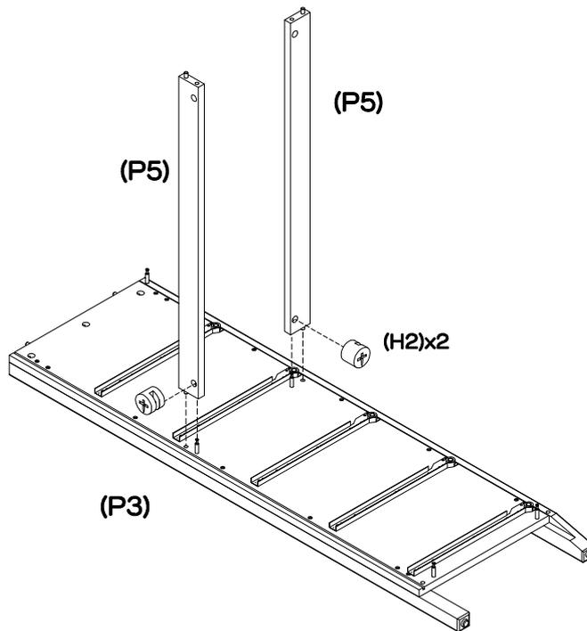
Attach 2 x middle rails (P5) to right side (P3), ensuring the sides with the cam nut holes are facing outwards. Using a phillips head screwdriver, rotate the cam nuts (H2) so the arrow points towards the incoming cam bolt. Turn clockwise to lock.
