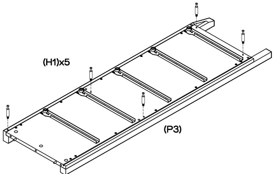
Attach 5 x large cam bolts (H1) into right side (P3) using a phillips head screwdriver.
