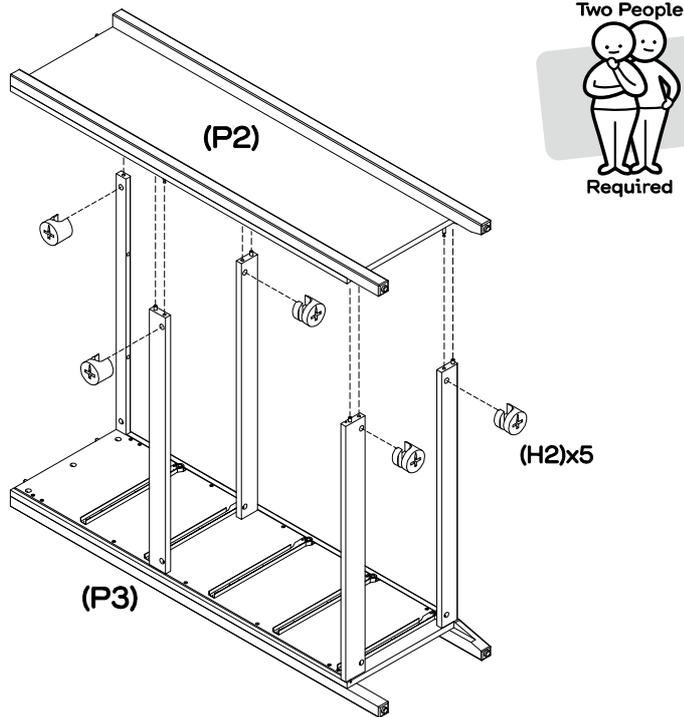
With assistance, attach left side (P2) to assembled unit. Insert 5 x large cam nuts into rails (P4, P5, P6, P7). Using a phillips head screwdriver, rotate the cam nuts (H2) so the arrows point towards the incoming cam bolt. Turn clockwise to lock.
