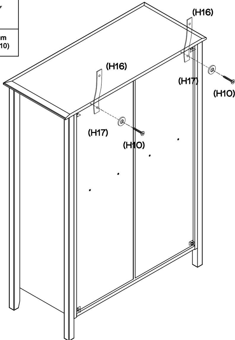
Attach 2 x wall straps (H16) to the back of top panel (P1) using 2 x medium screws (H10) and 2 x washers (H17), tightening using a phillips head screwdriver.
