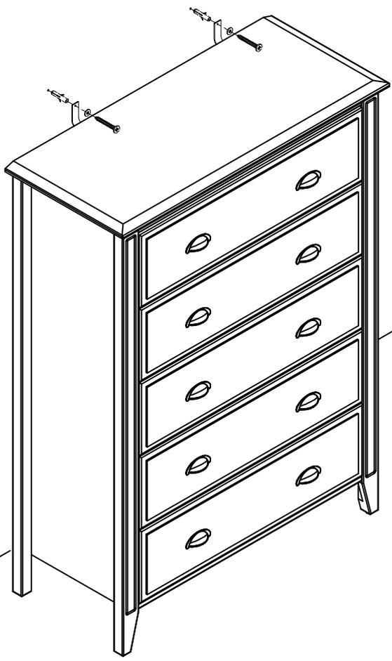
With assistance, move the tallboy to its final position. Attach the 2 x safety straps (H16) to the wall. Ensure it is firmly attached and secure.
