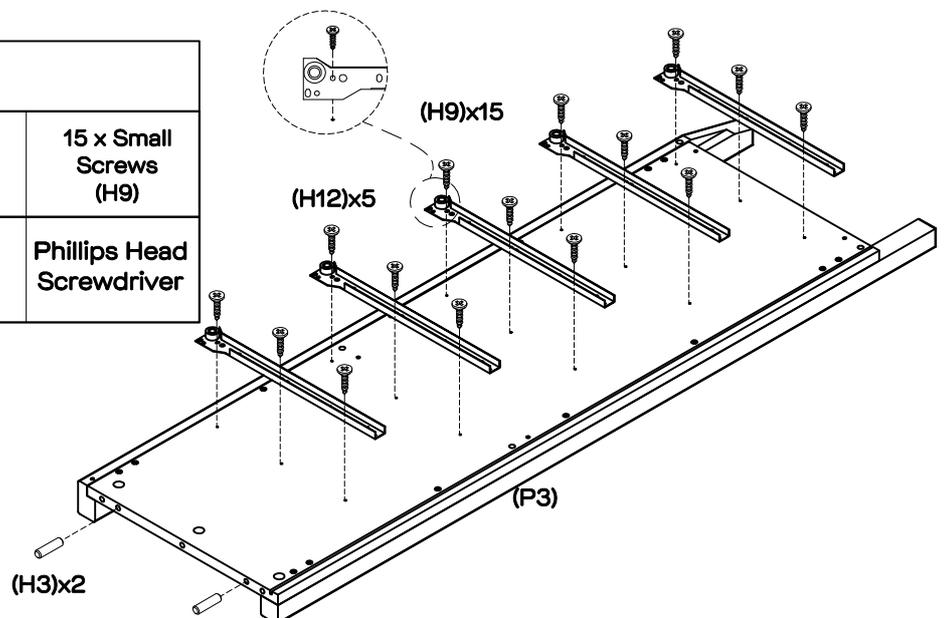
Insert 2 x wooden dowels (H3) into right side (P3). Attach 5 x right runner tracks (H12) to right side (P3) using 15 x small screws (H9), tightening using a phillips head screwdriver. Ensure the screws are inserted into the holes on the tracks (H12) as shown above.
