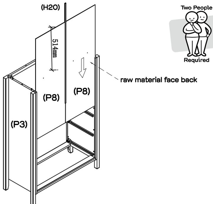
With assistance, carefully turn the unit upright. Slide the 2 x back panels (P8) into the grooves on the side panels (P2, P3) and rear lower rail (P6). Ensure the informative label is positioned as shown. Insert the plastic strip (H20) between the 2 x back panels (P8) as shown.
