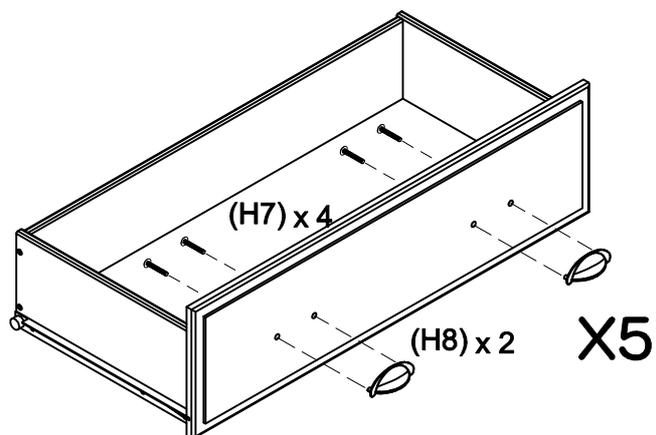
Attach 2 x handles (H8) to 1 x drawer front (P9) using 4 x handle screws (H7), tightening with a phillips head screwdriver. Repeat this process for the other 4 x assembled drawers.
