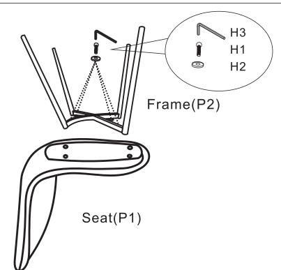
Align the holes on the Frame (P2) to the Screw holes of the seat (P1). Fix Frame (P2) to the Seat (P1) with 4 X Washes (H2) and 4 X Screws (H1). Fully tighten the bolts using Allen Key (H3).
