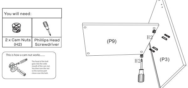
Insert 2 x Cam Nuts(H2) into Short Shelf(P9) as shown.Rotate the cam nuts so the arrows point towards the incoming cam bolts. Attach Short Shelf(P9) to Right Panel(P3) by tightening the cam nuts(H2) with the Phillips Head Screwdriver
