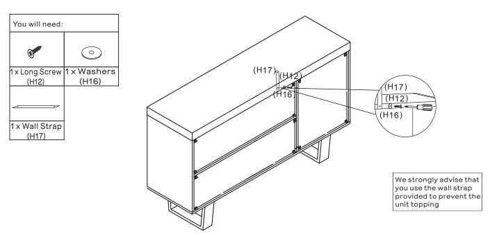
Use the Washer( H16 )and Long Screw(H12) to connect the Wall Strap (H17) to the Middle of top Shelf (P1) using the Phillips head Screwdriver.
