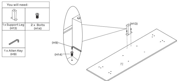
Using  $2 \times Bolts(H14)$  secure the Support Leg(H13) to the Unit Bottom(P2) by tightening with Allen Key(H9).
