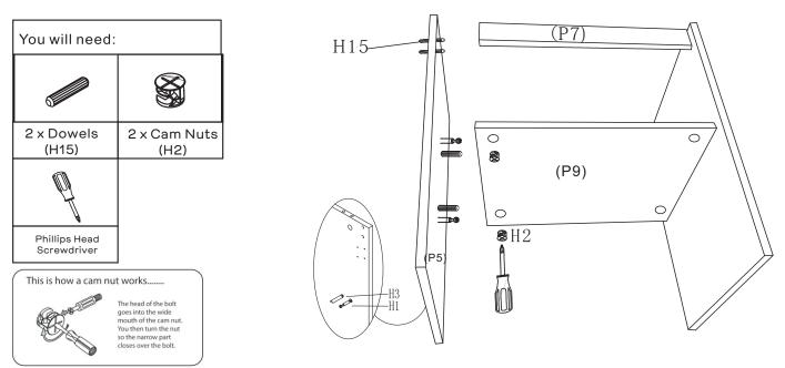
Insert 2 x Dowels(H15) into Middle Panel(P5) Insert 2 x Cam Nuts(H2) into Short Shelf(P9) as shown. Rotate the cam nuts so the arrows point towards the incoming cam bolts. Attach the Short Shelf (P9) and Short Support(P7) to Middle Panel(P5) by tightening the Cam Nuts(H2) with the Phillips Head Screwdriver.
