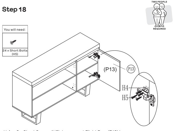
Using 8 x Short Screws(H5) to connect Right Door(P13) to Buffet by tightening with a Phillips head screwdriver. Repeat previous step for Right Door(P13) and Left Door(P12) TWO PEOPLE
