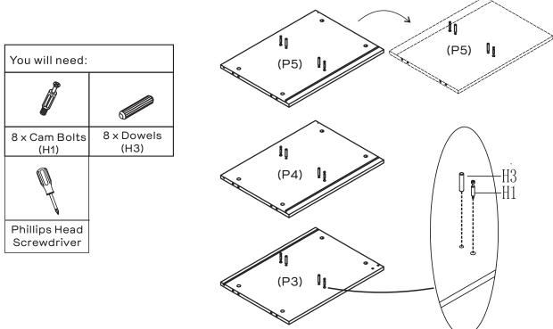
Insert 2 x Dowels(H3) into Right Panel(P3) and secure 2 x Cam Bolts(H1) to Right Panel(P3) by tightening with the Phillips Head Screwdriver. Repeat previous step for Left Panel (P4)
