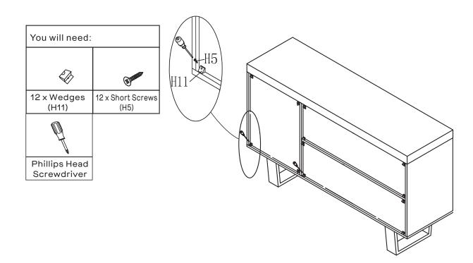
Insert 12 x Wedges(H11) into all corners of the back of the assembled unit as shown. Secure Wedges(H11) by tightening 12 x Short Screws(H5) with the Phillips Head Screwdriver.
