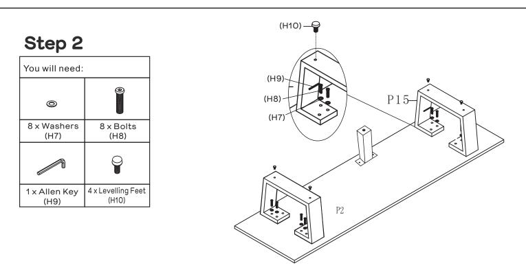
Use 8 x Bolts(H8) and 8 x Washers(H7) to secure the Leg(P15) to Bottom(P2). Tighten with Allen Key (H9), do not tighten fully. Screw in 4 x Levelling Feet(H10) to the bottom of the 2 x Legs(P15). Ensure they are secure, and if required can be adjusted accordingly.
