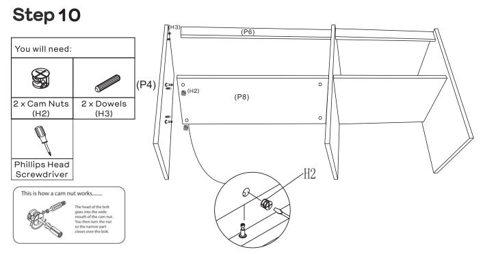
Connect Long Support(P6) to Middle Panel(P5) by Dowels(H15). Insert 2 x Dowels(H3) into Left Panel(P4) to connect with Long Support(P6). Insert 2 x Cam Nuts (H2) into Long Shelf(P8) as shown. Rotate the cam nuts so the arrows point towards the incoming cam bolts. Attach Long Shelf(P8) to Left Panel(P4) by tightening the Cam Nuts(H2) with the Phillips Head Screwdriver
