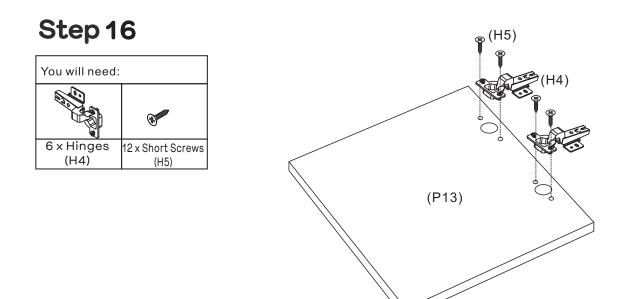
Using 4 x Short Screws(H5) to connect 2 x Hingers(H4) to Right Door(P13) Adjust the door then tighten all screws with a Phillips Head Screwdriver. Repeat previous step for Anther Right Door(P13) and Left Door(P12)
