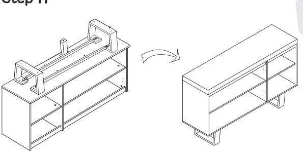
With assistance, carefully turn the unit upright. Note: Avoid using the centre support leg as a handle or pivoting point when turning the buffet over
