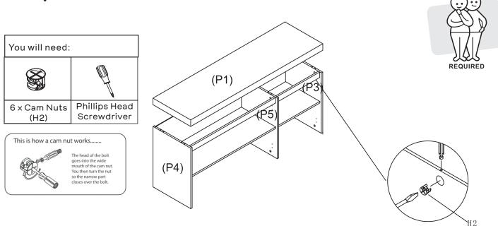
Insert 6 x Cam Nuts(H2) into Panel(P3&P4&P5) as shown.Rotate the cam nuts so the arrows point towards the incoming cam bolts. With assistance, attach Top(P1) to Panel(P3&P4&P5) by tightening the Cam Nuts(H2) with the Phillips Head Screwdriver
