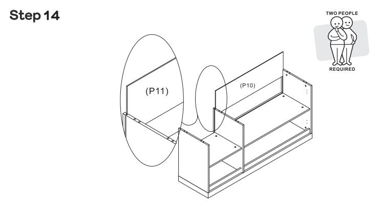
With assistance, carefully turn the buffet upside down. Slide another Long Back Panel(P10) and Short Back Panel(P11)into the groove.
