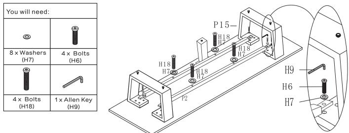
Align the 2 x Connectors(P14) onto the Bottom(P2) as shown. Use 4 x Bolts(H6) and 4 x Washers(H7) to secure the 2 x Connectors(P14) to the 2 x Legs(P15), tightening with Allen Key(H9). Use 4 x Bolts(H18) and 4 x Washers (H7) to secure the 2 x Connectors(P14) to the Bottom (P2), tightening with Allen Key(H9). Ensure bolts are fully tightened.
