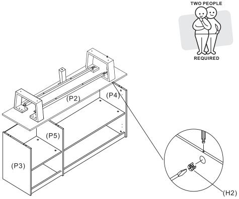
Insert 6 x Cam Nuts(H2) into Panel(P3&P4&P5) as shown. Rotate the cam nuts so the arrows point towards the incoming cam bolts. With assistance, attach Bottom(P2) to Panel(P3&P4&P5) by tightening the Cam Nuts(H2) with the Phillips Head Screwdriver
