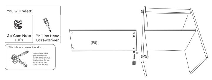
Insert 2 x Cam Nuts(H2) into Long Shelf(P8) as shown. Rotate the cam nuts so the arrows point towards the incoming cam bolts. Attach Long Shelf(P8) to Middle Panel(P5) by tightening the Cam Nuts(H2) with the Phillips Head Screwdriver
