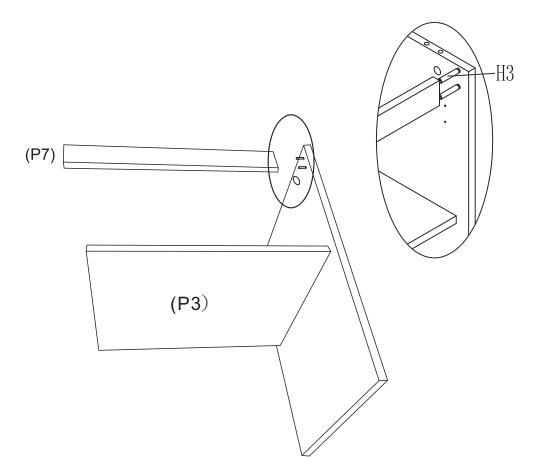
Insert 2 x Dowels(H3)into Right Panel(P3) and connect Short Support(P7) to Right Panel(P3).
