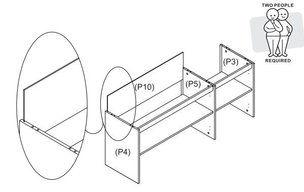
With assistance, carefully turn the buffet upright. Slide Long Back Panel(P10) into the groove of Left Panel(P4) and Middle Panel(P5) as shown.
