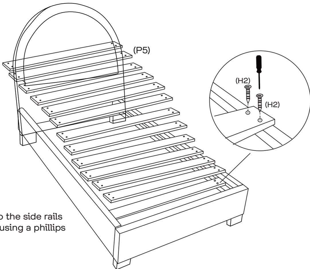
Attach the 13 x slats (P5) to the side rails (P3) with 52 x screws (H2) using a phillips head screwdriver.
