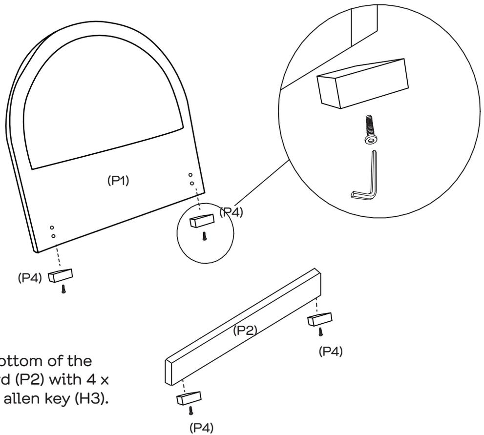
Attach 2 x legs (P4) to the bottom of the headboard (P1) and footboard (P2) with 4 x bolts (H1) by tightening with allen key (H3).
