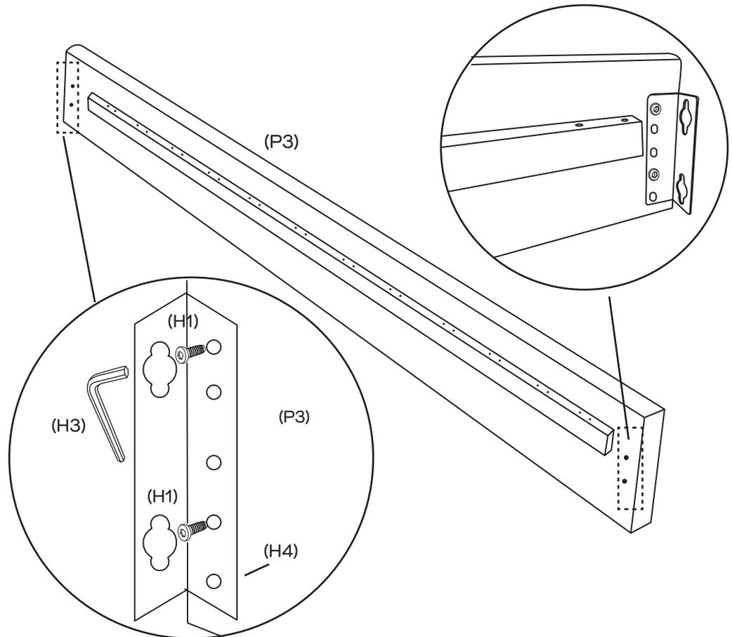
Attach the 4 x brackets (H4) to the ends of the side rails (P3) as shown. Screw in 2 x bolts (H1) into each bracket with the allen key (H3). Ensure to fully tighten all bolts.
