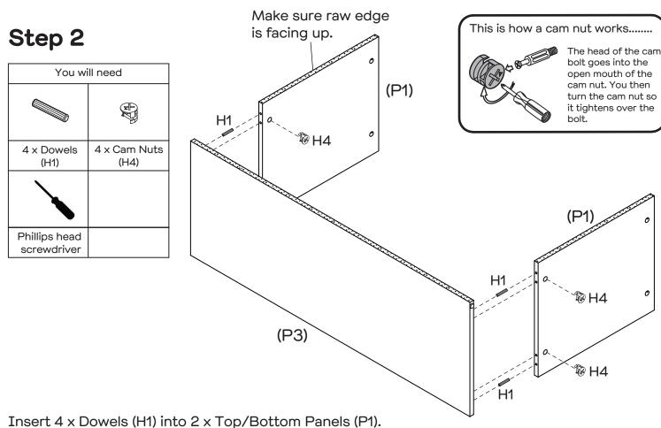
Insert 4 x Cam Nuts (H4) into the holes of 2 x Top/Bottom Panels (P1).
