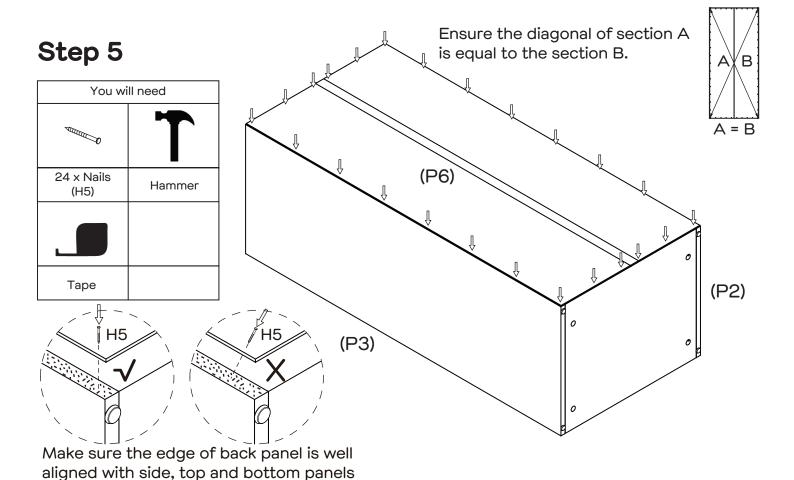
Attach Back Panel (P6) to the cabinet with 24 x Nails (H5) using hammer. Please measure with a tape to ensure that the spacing of the nails is consistent, and make sure the tip of the nails are vertically centered on the edge of the Side Panels(P2, P3) and Top/Bottom Panels (P1).
