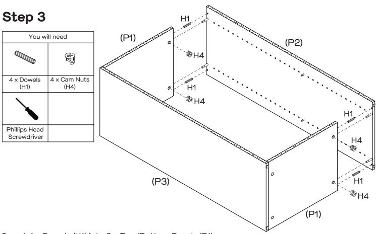
Insert 4 x Dowels (H1) into 2 x Top/Bottom Panels (P1). Insert 4 x Cam Nuts (H4) into the holes of 2 x Top/Bottom Panels (P1). Rotate the cam nuts so the arrows point towards the incoming cam bolts. Push Left Side Panel (P2) into place and tighten the cam nuts.
