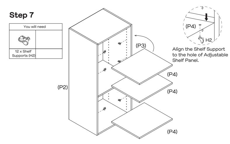
Insert 12  $\times$  Shelf Supports (H2) into the holes of Side Panels (P2, P3) as shown. Insert 3  $\times$  Adjustable Shelf Panels (P4) into the cabinet.
