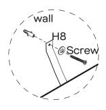
Move the cabinet to the final position. Attach the safety strap to the wall. Make sure it is firmly attached and make sure it is a snug fit.
