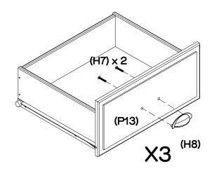
Attach 1 x drawer handle (H8) to 1 x drawer front (P13) using 2 x drawer handle screws (H7), tightening with a phillips head screwdriver. Repeat this process for the other 2 x drawers.
