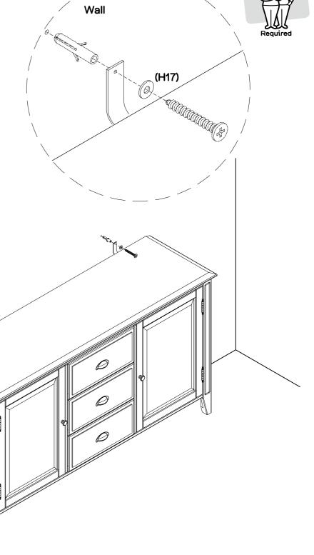
With assistance, move the buffet to its final position. Attach the  $2\times$  wall straps to the wall, ensuring it is firmly attached and secure.
