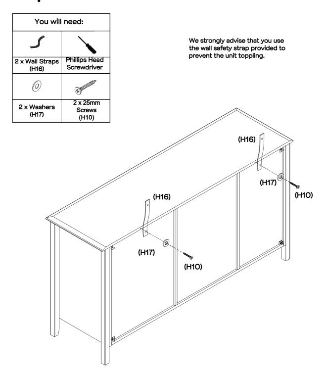
Attach 2 x wall straps (H16) to the back of the top panel (P1) using 2 x 25mm screws (H10) and 2 x washers (H17).
