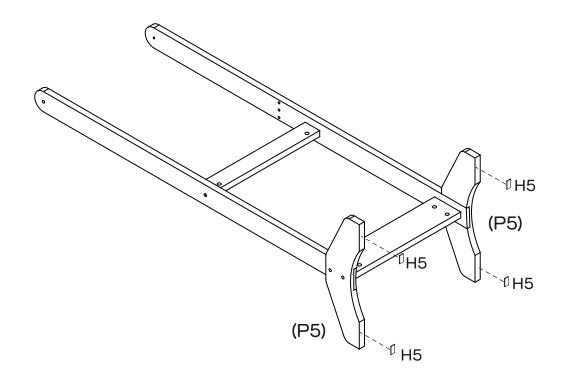
Apply 4 x Felt pads (H5) to bottom of Legs (P5) as shown.
