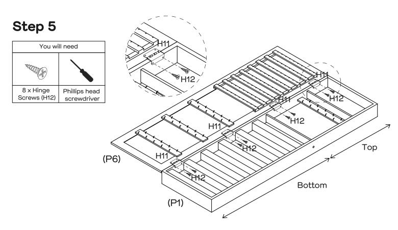
Secure Door panel (P6) to Cabinet (P1) by attaching reverse of 4 x Hinges (H11) with 8 x Hinge Screws (H12) by tightening with Phillips Head Screwdriver.
