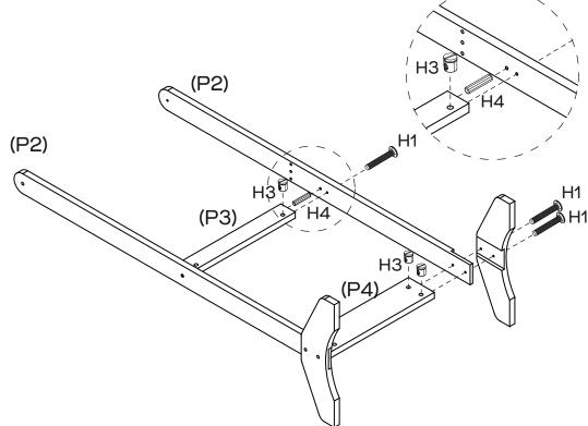
Insert 1 x Dowel (H4) & 1 x Barrel (H3) into Support Rail (P3) and 2 x Barrels (H3) into Support Rail (P4). Ensure the Barrels (H3) are rotated horizontally with the Flat Head Screwdriver ready for the incoming Bolts. Use 3 x Bolts (H1) to attach Support Leg (P5) and Support Rails (P3&P4) to Frame (P2) as shown by tightening the Bolts with the Phillips Head Screwdriver.
