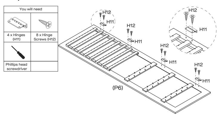
Attach 4 x Hinges (H11) to Door panel (P6) and secure by tightening 8 x Hinge Screws (H12) with the Phillips Head Screwdriver.
