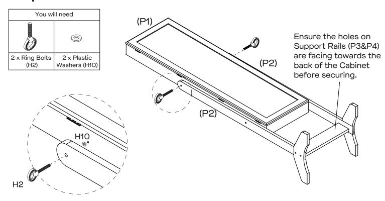
Thread the Ring Bolts (H2x2) and Plastic Washers (H10x2) through each side of the Frame (P2) and secure to the Cabinet (P1) by winding the Ring Bolts (H2x2) to tighten.
