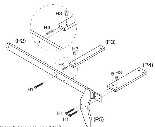
Insert 1 x Dowel (H4) & 1 x Barrel (H3) into Support Rail (P3) and 2 x Barrels (H3) into Support Rail (P4). Ensure the Barrels (H3) are rotated horizontally with the Flat Head Screwdriver ready for the incoming Bolts. Use 3 x Bolts (H1) to attach Support Leg (P5) and Support Rails (P3&P4) to Frame (P2) as shown by tightening the Bolts with the Phillips Head Screwdriver.
