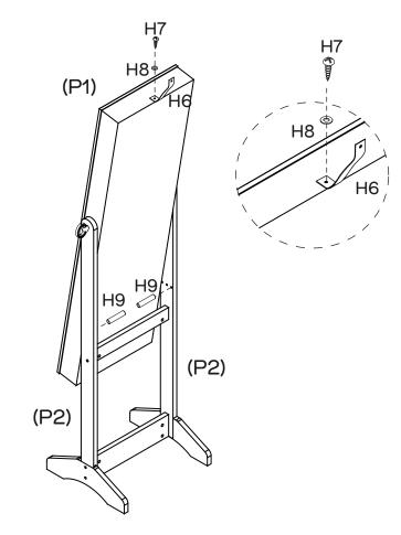
of the Cabinet (P1) use 1 x Washer (H8) and Screw (H7) by tightening with the Phillips Head Screwdriver. We strongly suggest you use the wall strap provided to prevent the unit from toppling.
