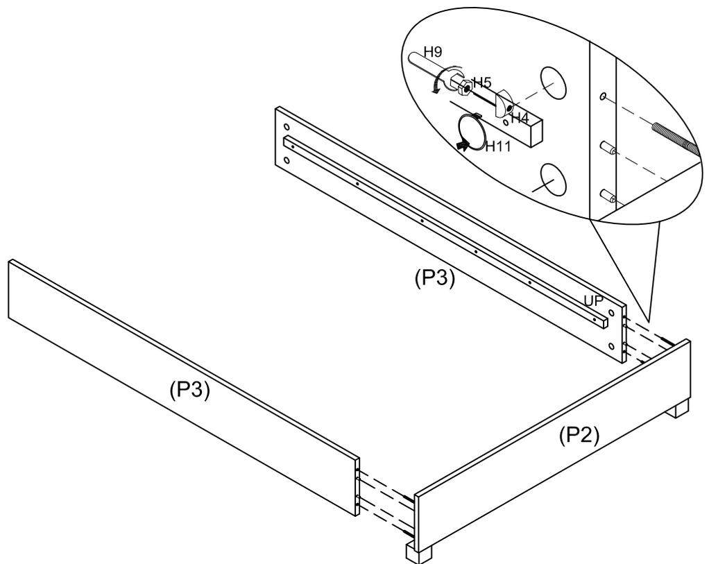
Attach 2 x Side Rails (P3) to Footboard (P2) by using 4 x Hexagonal Nuts (H5) 4 x Halfround Nut (H4) as show, tighten with a Spanner (H9), insert 4 x Caps (H11)
