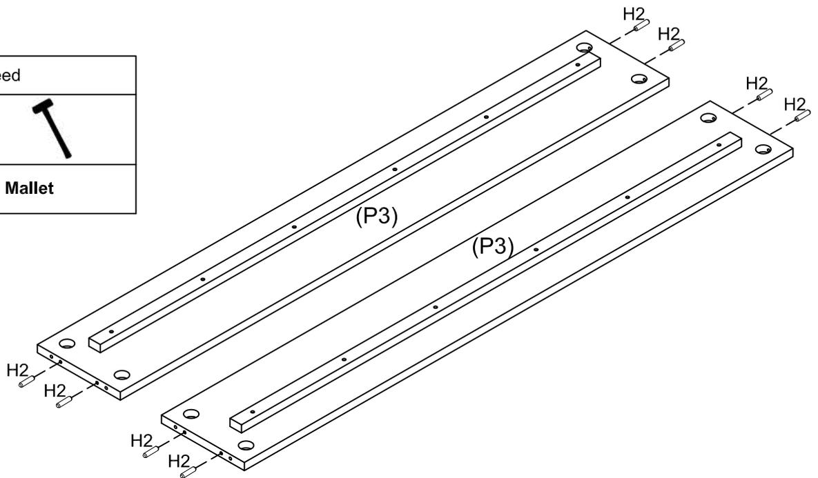
Using the Mallet if needed, Insert 8 x Wooden Dowels (H2) to the hole on Side Rails (P3) as shown.
