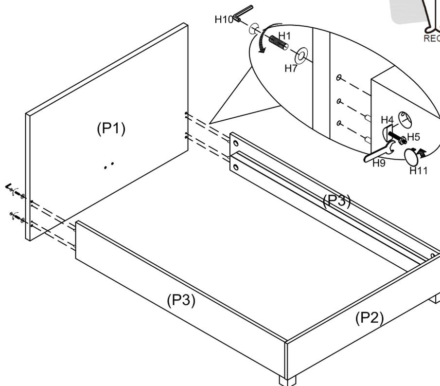
Attach Headboard (P1) to Side Rail (P3) by using 4 x Bolt (H1) 4 x Hexagonal Nuts (H5) 4 x Half Round Nut (H4) and 4 x Washer (H7) as shown, tighten with a Spanner (H9) and Allen Key (H10), and insert 4 x Caps (H11)
