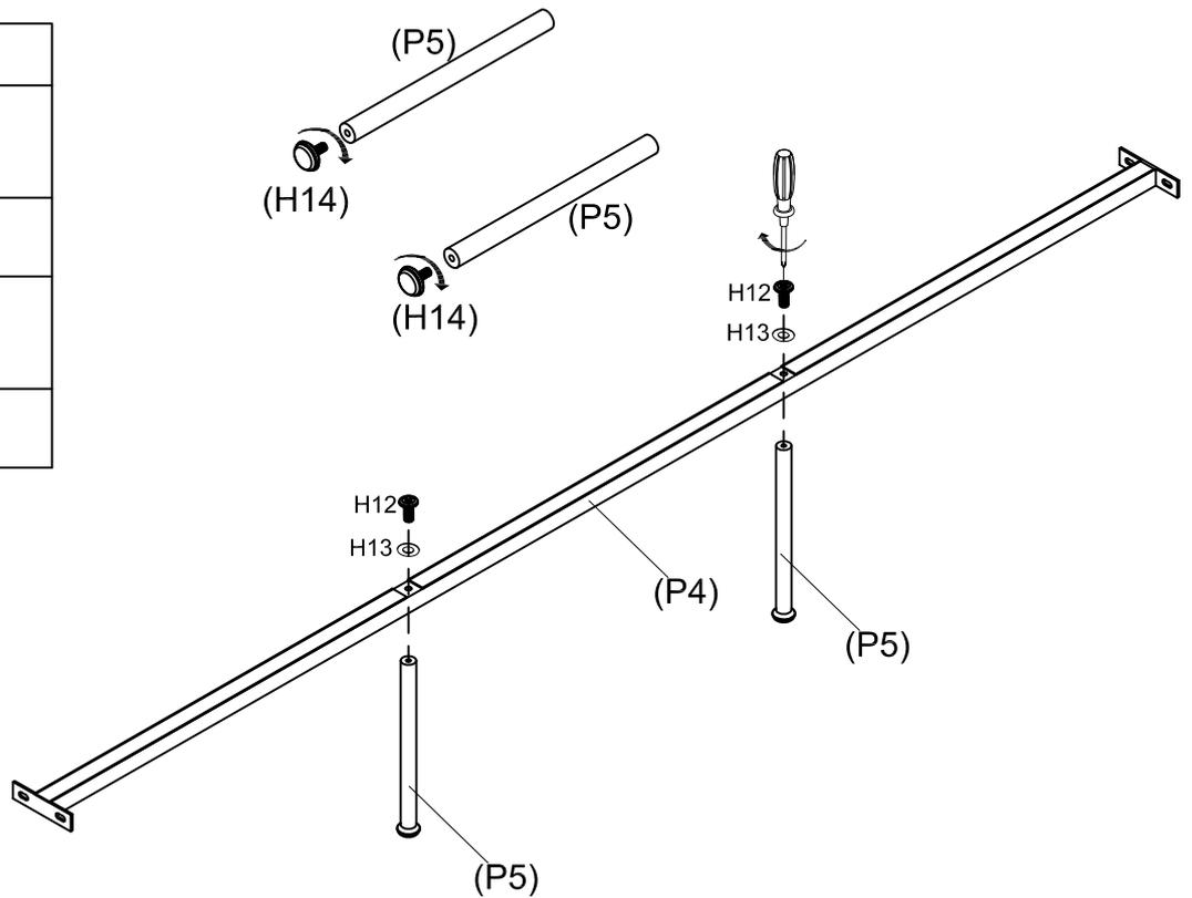
Insert the 2 x Stoppers (H14) to the 2 x Support legs (P5). Attach 2 x Support Legs (P5) to Centre Rail (P4) by using 2 x Bolt (H12) and Washer (H13) tighten with a Phillips Head Screwdriver.
