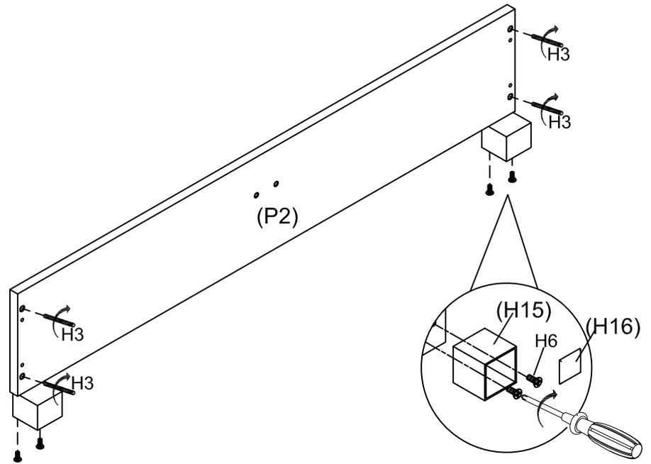
Screw 4 x Bolt (H3) onto Footboard (P2) Attach 2 x Legs (H15) to Footboard (P2) by using 4 x Bolt (H6), and tighten with a Phillips Head Screwdriver. Then insert the Leg cap (H16) as shown.
