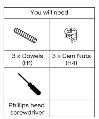
Insert 3 x Dowels (H1) & 3 x Cam Nuts (H4) into Shelf panel (P5) and Rail (P11). Attach Divider panel (P4) to Shelf panel (P5) and Rail (P11), secure by tightening Cam Nuts (H4) with a Phillips Head Screwdriver.
