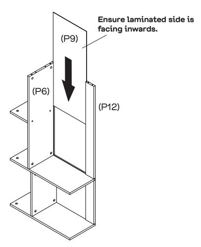
Slide Back panel (P9) into the grooves of the Shelf panel (P6) and Rail (P12) as shown.
