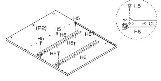
Attach 2 x CL Runner Tracks (H6) to Left Side Panel (P2) with  $6 \times 8$  Small Screws (H5) by tightening with the Phillips Head Screwdriver.
