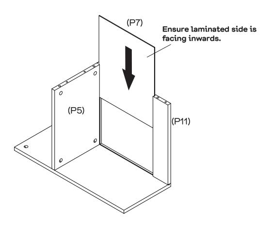
Slide Back panel (P7) into the grooves of the Shelf panel (P5) and Rail (P11) as shown.
