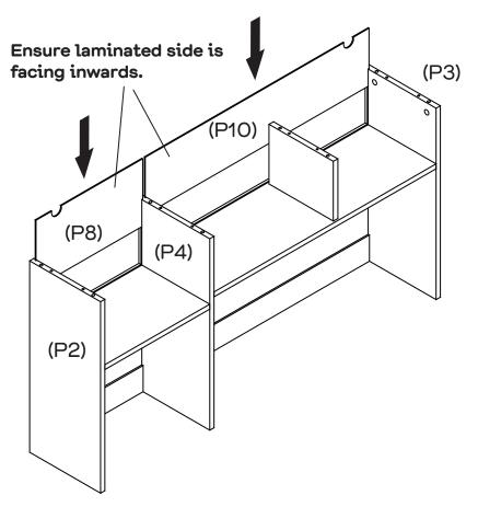
Slide Back panels (P8) & (P10) into the grooves of the Left panel (P2), Divider panel (P4) & Right panel (P3) as shown.
