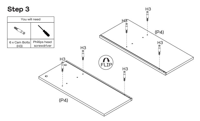
Secure 3 x Cam Bolts (H3) to Divider Panel (P4) by tightening with the Phillips Head Screwdriver. Flip the Divider Panel (P4) over and secure another  $3 \times 1$  Cam Bolts (H3) to the other side by tightening with the Phillips Head Screwdriver.
