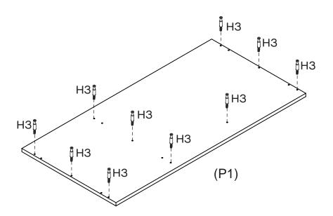
Attach 10 x Cam Bolts (H3) to Top Panel (P1) by tightening with the Phillips Head Screwdriver.
