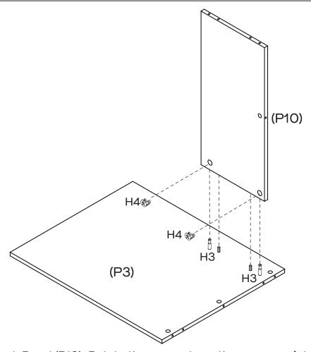
Insert 2 x Cam Nuts (H4) into Back Panel (P10). Rotate the cam nuts so the arrows point towards the incoming cam bolts. Attach Back Panel (P10) to Right Side Panel (P3) by tightening cam nuts with the Phillips Head Screwdriver.
