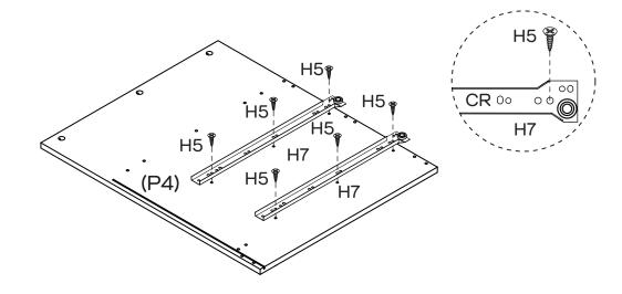
Attach  $2 \times CR$  Runner Tracks (H7) to Divider (P4) with  $6 \times Small$  Screws (H5) by tightening with the Phillips Head Screwdriver.
