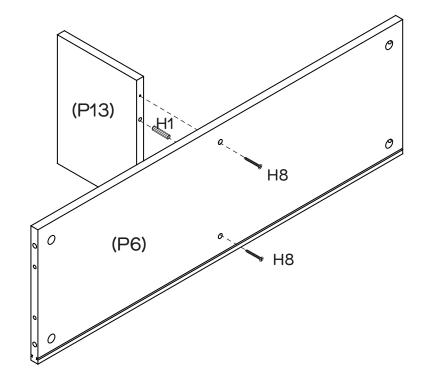
Insert 2  $\times$  Dowels (H1) into Shelf panel (P6), attach to Divider panel (P13) and secure with 2  $\times$  Large Screws (H8) by tightening with a Phillips Head Screwdriver.
