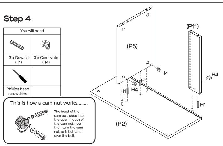
Insert 3  $\times$  Dowels (H1) & 3  $\times$  Cam Nuts (H4) into Shelf panel (P5) and Rail (P11). Attach Left panel (P2) to Shelf panel (P5) and Rail (P11), secure by tightening Cam Nuts (H4) with a Phillips Head Screwdriver.
