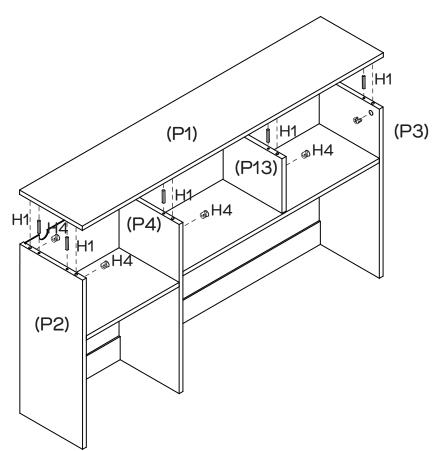
Insert 8 x Dowels (H1) & 8 x Cam Nuts (H4) into the Left Side Panel (P2), Right Side panel (P3), Divider Panel (P4) and Divider Panel (P13). Attach Top Panel (P1) to the unit and secure by tightening the Cam Nuts (H4) with the Phillips Head Screwdriver.
