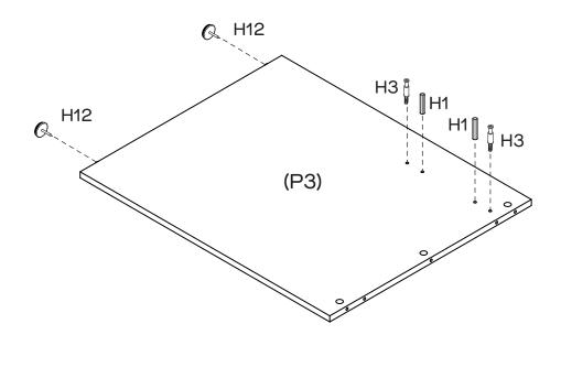
Insert 2 x Dowels (H1) into Right Side Panel (P3). Attach 2 x Cam Bolts (H3) to Right Side Panel (P3) by tightening with the Phillips Head Screwdriver. Use the Hammer to secure the  $2 \times Plastic$  Glides (H12) to the bottom of Right Side Panel (P2) as shown.
