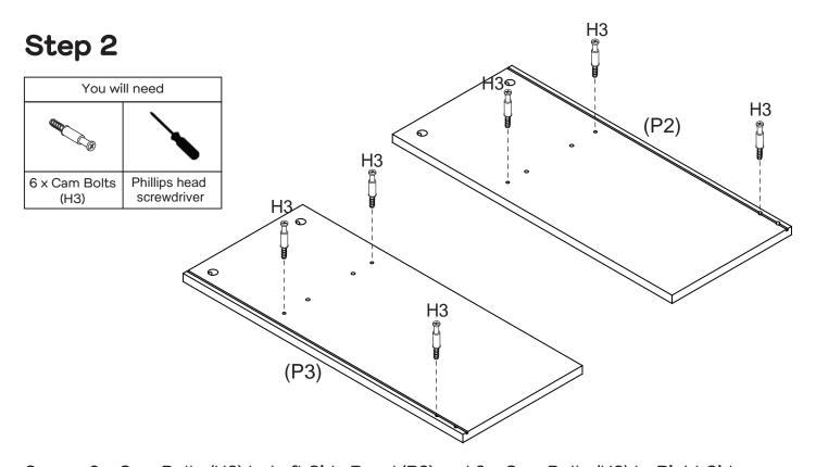
Secure 3  $\times$  Cam Bolts (H3) to Left Side Panel (P2) and 3  $\times$  Cam Bolts (H3) to Right Side Panel (P3) by tightening with the Phillips Head Screwdriver.
