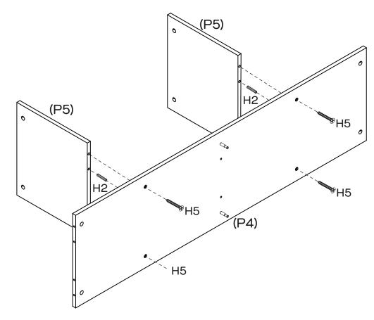
Insert 4 x Small Dowels (H2) into the holes of Shelf Panel (P4) as shown. Attach Dividers (P5) to Shelf Panel (P4) with 4 x Long Screws (H5). Tighten the screws with a Phillips Head Screwdriver.
