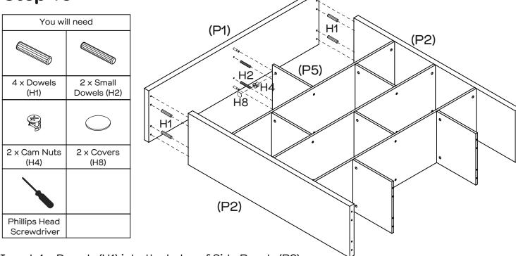
Insert 4 x Dowels (H1) into the holes of Side Panels (P2).
