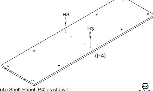
Attach 2 x Cam Bolts (H3) into Shelf Panel (P4) as shown.
