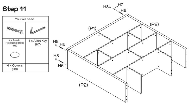
Secure Top Panel (P1) to Side Panels (P2) with 4 x Inside Hexagonal Bolts (H6) using an Allen Key (H7). Seal the holes with 4 x Covers (H8) as shown.
