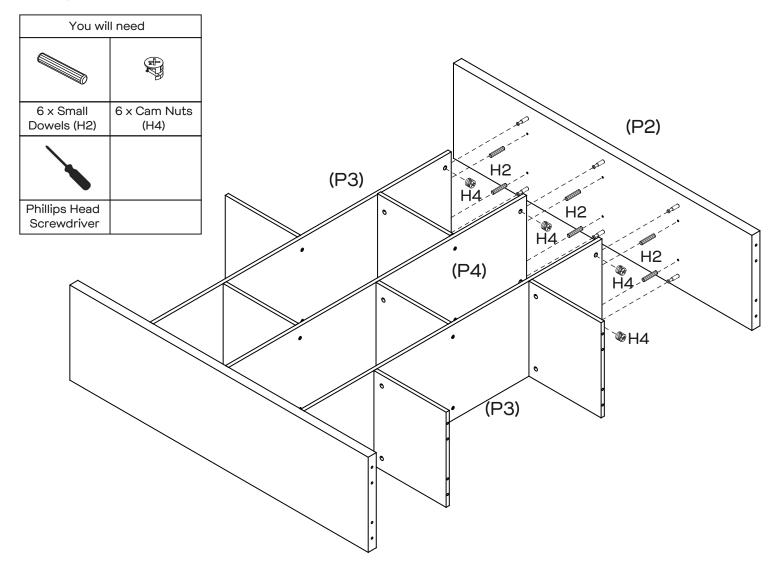
Insert 6 x Small Dowels (H2) into the holes of Shelf Panels (P3, P4). Insert 6 x Cam Nuts (H4) into the holes of Shelf Panels (P3, P4). Rotate the Cam Nuts so the arrows point towards the incoming Cam Bolts. Push Side Panel (P2) into place and then tighten the Cam Nuts.
