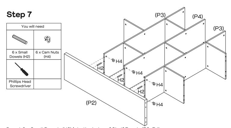
Insert 6 x Small Dowels (H2) into the holes of Shelf Panels (P3, P4).
