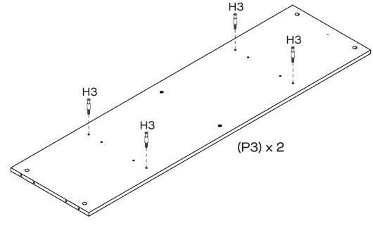
Attach 4 x Cam Bolts (H3) into each Shelf Panel (P3) as shown.
