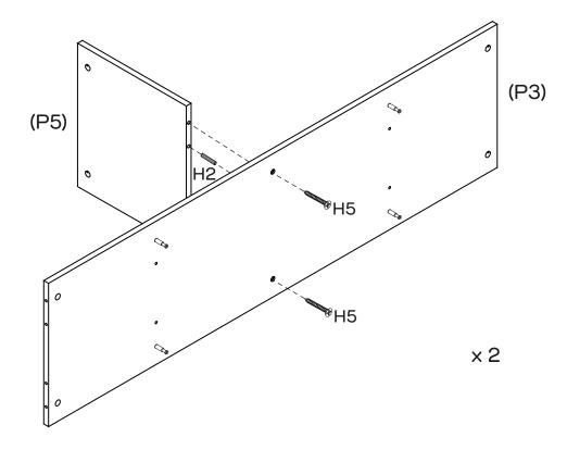
Insert 2 x Small Dowels (H2) into the holes of Divider (P5) as shown. Attach Shelf Panel (P3) to Divider (P5) with 2 x Long Screws (H5). Tighten the screws with a Phillips Head Screwdriver. Repeat Step 4 for the other Divider (P5) and Shelf Panel (P3).
