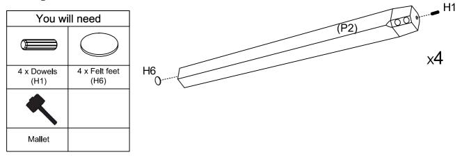
Insert each dowel (H1) into leg (P2). Attach each felt feet (H6) onto leg (P2).
