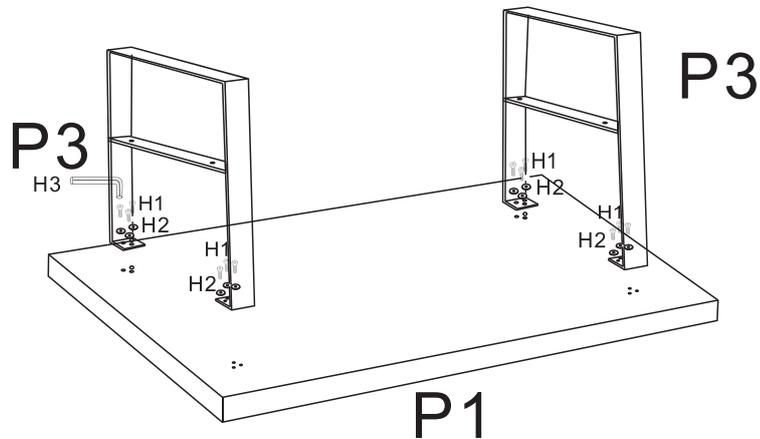
Using 6 x Washers(H2) and 6 x Short Bolts (H1) secure the Table Leg (P3) to the Table Top(P1) by tightening 70% with Allen Key (H3)
