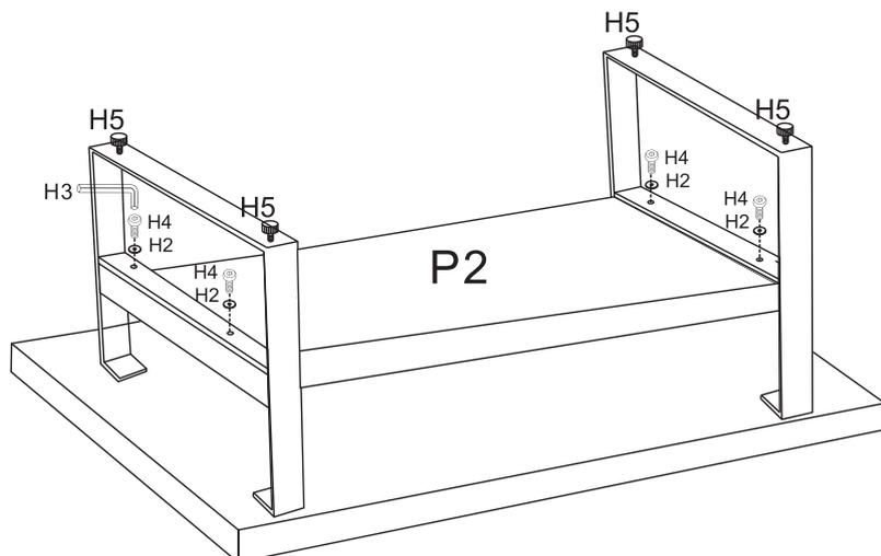
Using 4 x Washers (H2) and 4 x Long Bolts (H4) to secure the Table leg (P3) to the Table Shelf (P2) by tightening with Allen Key (H3)
