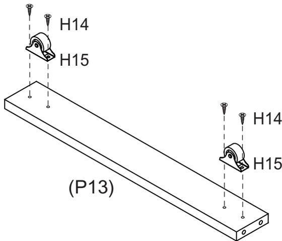
Attach 2 x Wheels (H15) to Drawer Support (P13) with 4 x Small Screws (H14). Repeat Step 2 again with the other Drawer Support (P13).
