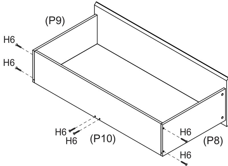
Attach Drawer Back (P10) to Drawer Sides (P8,P9) with 4 x Screws (H6),
