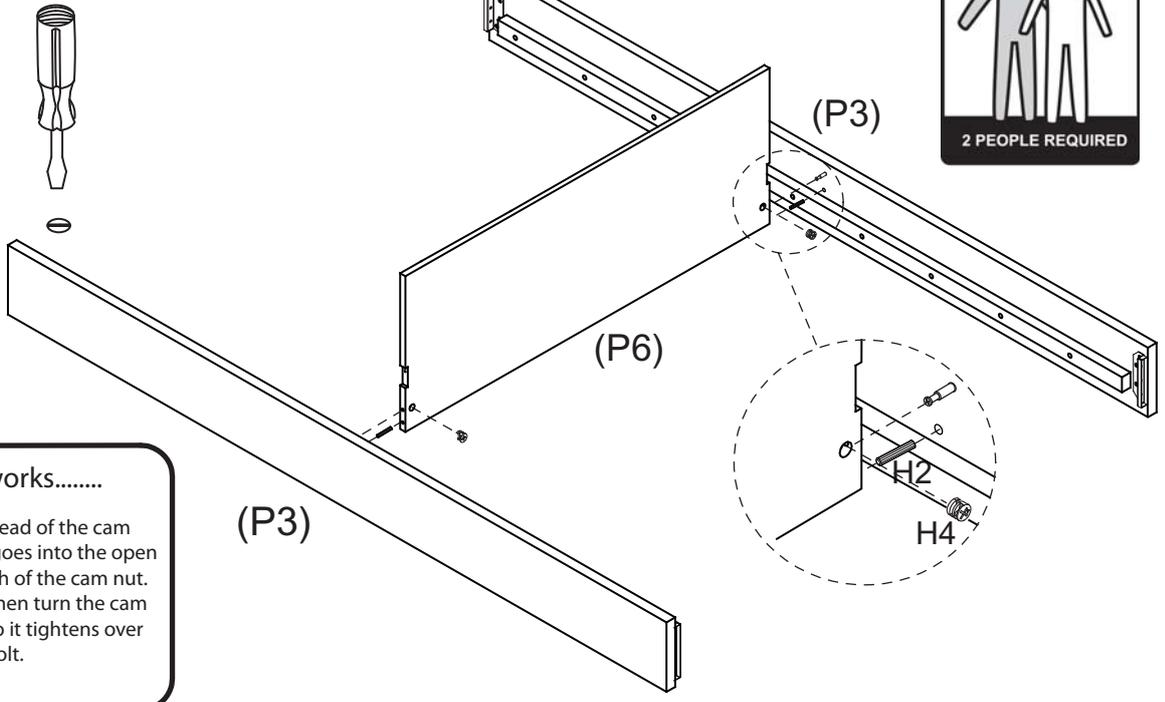
**This is how a cam nut works.....**
