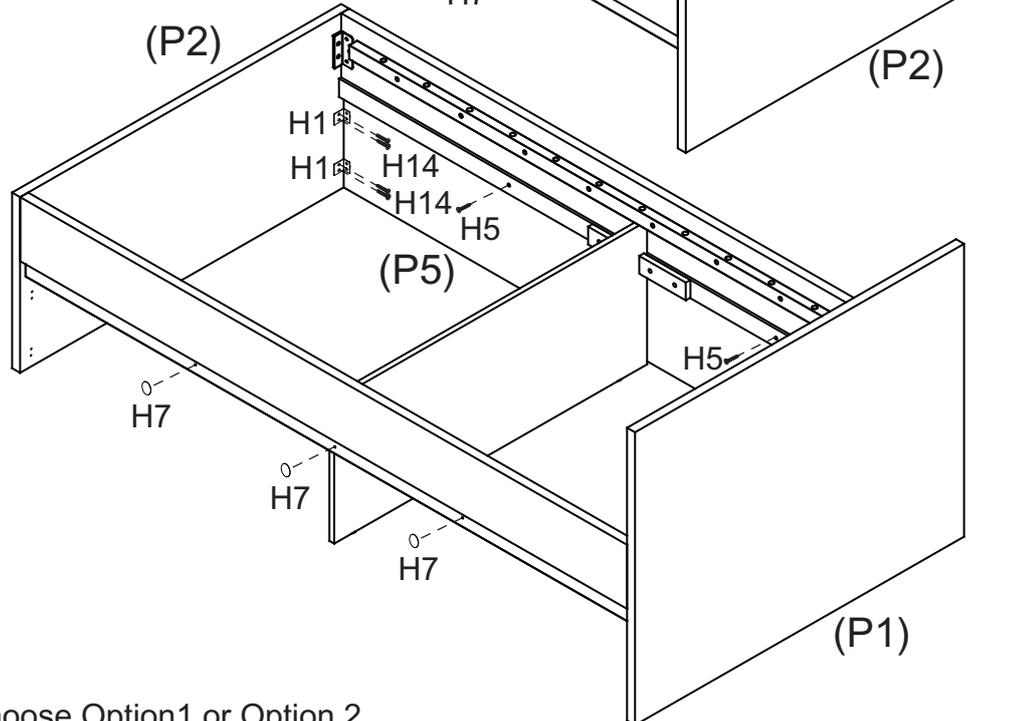
Whether you would like to choose Option 1 or Option 2, please attach Base Panel (P5) to Bedboard (P1,P2) with 8 x Small Screws (H14). Attach Base Panel (P5) to Rails (P4) with 2 x Screws (H5). Attach 3 x Stickers (H7) to the holes of Rail (P4). And then follow the rest steps to assemble.
