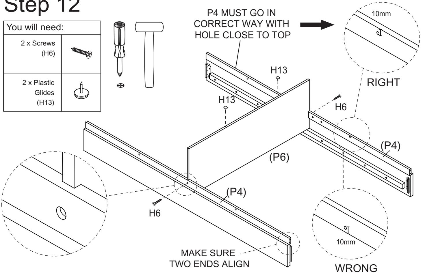
Attach Rails (P4) to Clapboard (P6) with 2 x Screws (H6).
