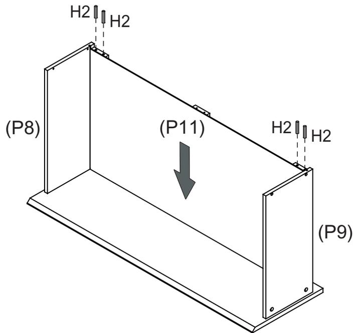
Slide Drawer Base (P11) into the groove in the Drawer Sides (P8,P9).
