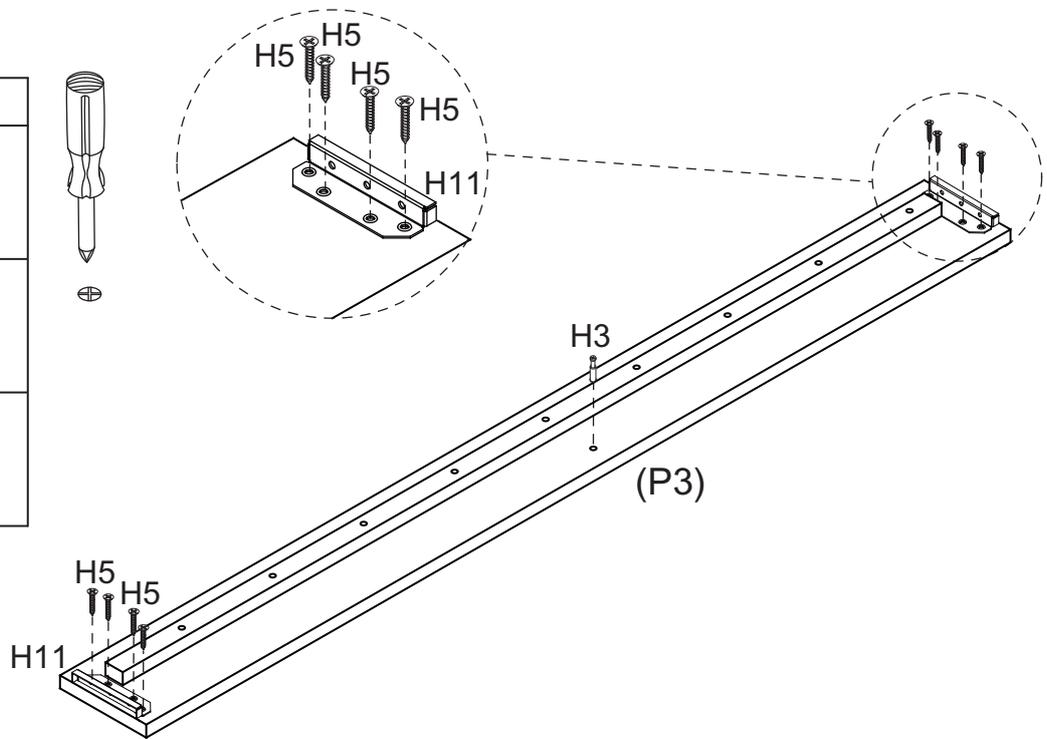
Attach 1 x Cam Bolt (H3) to Side Rail (P3).
