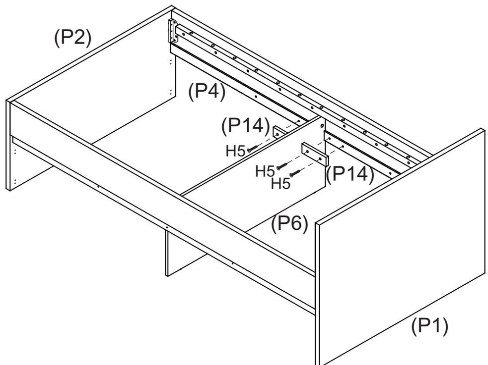
Attach 2 x Blocks (P14) to Rail (P4) with 4 x Screws (H5).
