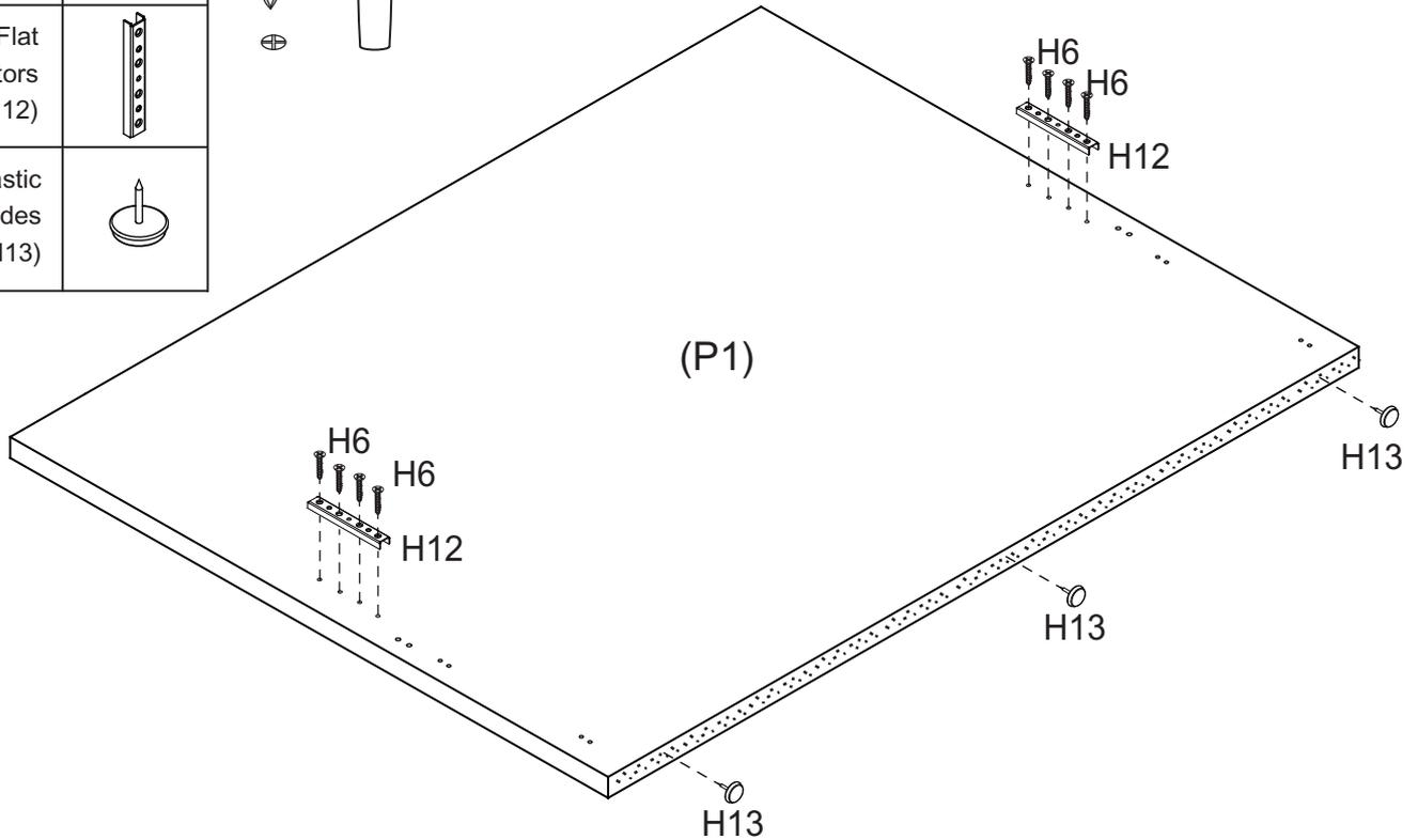
Attach 2 x Flat Connectors (H12) to Bedhead (P1) with 8 x Screws (H6).
