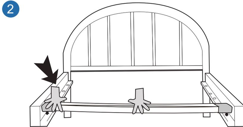
Place the slat in position then push down in the centre to flatten. Make sure the plastic prong lines up with the hole, then push in firmly.
