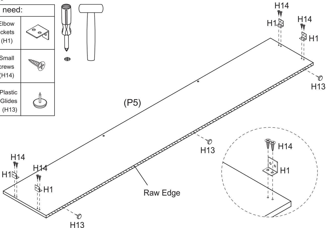
Attach 4 x Elbow Brackets (H1) to Base Panel (P5) with 8 x Small Screws (H14).
