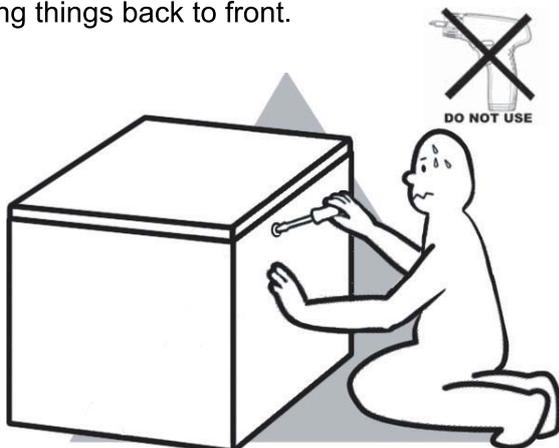
**DO NOT** fully tighten screws (leave slightly loose). When the item is fully assembled tighten the screws - but do not over tighten.
