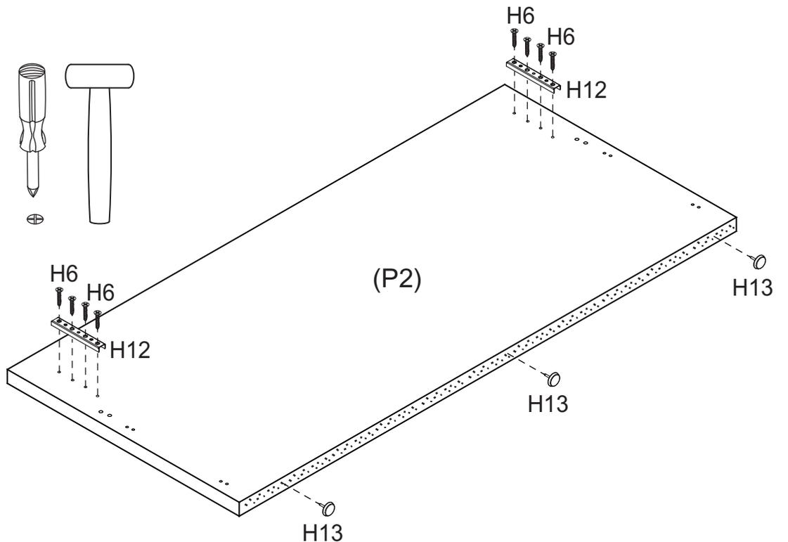
Attach 2 x Flat Connectors (H12) to Bedfoot (P2) with 8 x Screws (H6).
