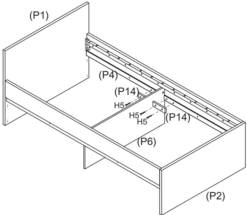
Attach 2 x Blocks (P14) to Rail (P4) with 4 x Screws (H5).
