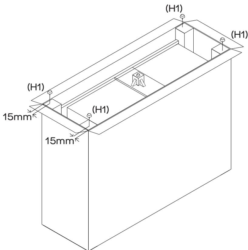
Use a Soft Headed Mallet to nail the gliders (H1) into the middle of the each leg.
