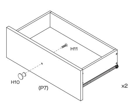
Attach 2 x Handles (H10) to Drawer Fronts (P7x2) with 2 x Handle Bolts (H11) by tightening with the Phillips Head Screwdriver.
