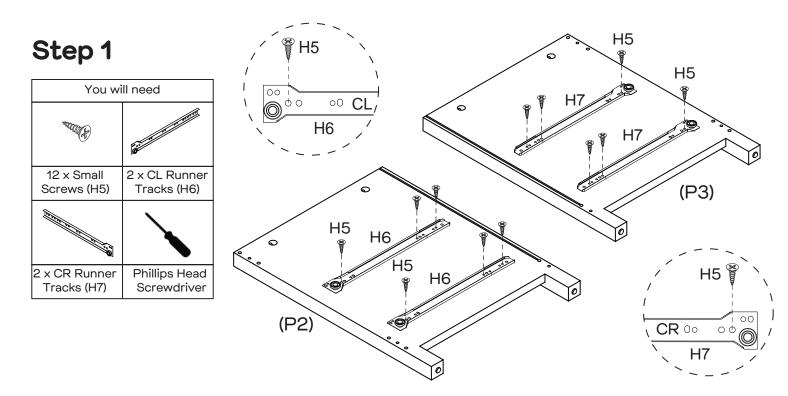
Attach  $2 \times CL$  RunnerTracks (H6) and  $2 \times CR$  Runner Tracks (H7) to Left&Right Side Panels (P2&P3) with 12 x Small Screws (H5) by tightening with the Phillips Head Screwdriver.
