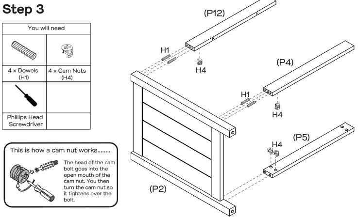
Insert 4x Dowels (H1) into Left Side Panel (P2). Insert 4 x Cam Nuts (H4) into Rails (P4&P5&P12) as shown. Rotate the cam nuts so the arrows point towards the incoming cam bolts. Attach Rails (P4&P5&P12) to Left Side Panel (P2) by tightening all cam nuts with the Phillips Head Screwdriver.
