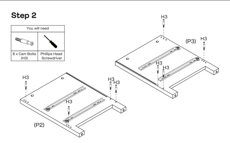
Attach 8 x Cam Bolts (H3) to Left&Right Side Panels (P2&P3) by tightening with the Phillips Head Screwdriver.
