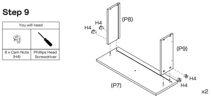
Attach Drawer Sides (P8x2&P9x2) to Drawer Front (P7x2). Insert 8 x Cam Nuts (H4) into the holes of Drawer Sides (P8x2, P9x2). Make sure the opening on cam nuts point towards the incoming cam bolts. Tighten with a Phillips Head Screwdriver.
