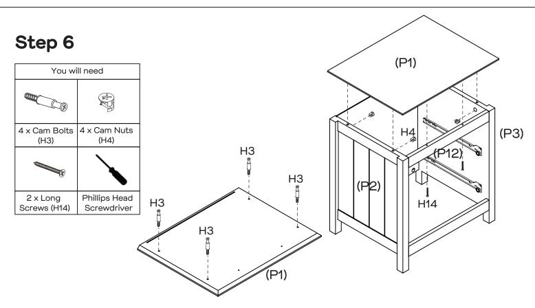
Attach 4 x Cam Bolts (H3) to Top Panel (P1) by tightening with the Phillips Head Screwdriver. Insert 4 x Cam Nuts (H4) into Left & Right Side Panel (P2&P3) as shown. Rotate the cam nuts so the arrows point towards the incoming cam bolts. Attach Top Front Rail (P12) to Top Panel (P1) with 2x Long Screws (H4). Attach Top Panel (P1) to Left & Right Side Panel (P2&P3) by tightening all cam nuts with the Phillips Head Screwdriver.
