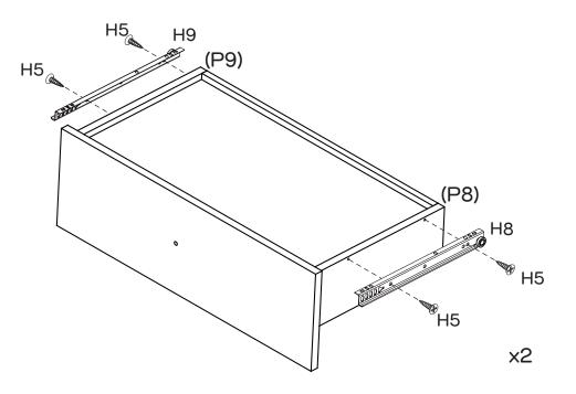
Attach  $2 \times DL$  Runners (H8) to Left Drawer Sides (P8x2) and  $2 \times DR$  Runners (H9) to Right Drawer Side (P9x2) with  $8 \times Small$  Screws (H5) using a Phillips Head Screwdriver.
