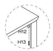
Secure Back Panel (P6) in place with 4 x Wedges (H12) using 4 x Wedge Screws (H13). Tighten with a Phillips Head Screwdriver.
