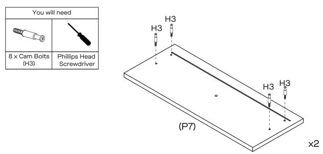
Attach 8 x Cam Bolts (H3) to Drawer Fronts (P7x2). Tighten with a Phillips Head Screwdriver.
