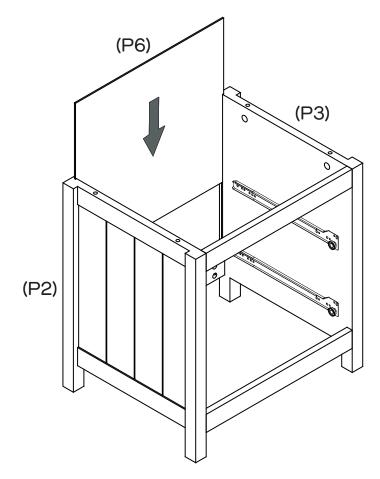
Slide Back Panel (P6) into the grooves of Left&Right Side Panels (P2&P3).
