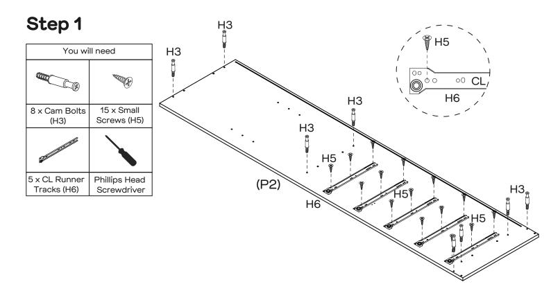
Attach 8 x Cam Bolts (H3) to Left Side Panel (P2) as shown by tightening with the Phillips Head Screwdriver. Attach 5 x CL Runner Tracks (H6) to Left Side Panel (P2) with 15 x Small Screws (H5) by tightening with the Phillips Head Screwdriver.
