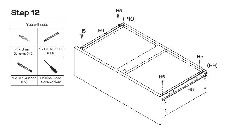
Attach 1 x DL Runner (H8) to the bottom of Left Drawer Side (P9) and 1 x DR Runner (H9) to the bottom of Right Drawer Side (P10) with  $4 \times Small Screws$  (H5) by tightening with the Phillips Head Screwdriver.
