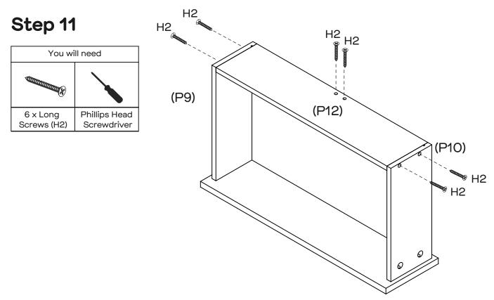
Attach Drawer Back (P12) to Left & Right Drawer Sides (P9 & P10) and Support Rail (P13) with 6 x Long Screws (H2) by tightening with the Phillips Head Screwdriver. Ensure the drawer base lines up with the grooves all the way around the drawer before securing.
