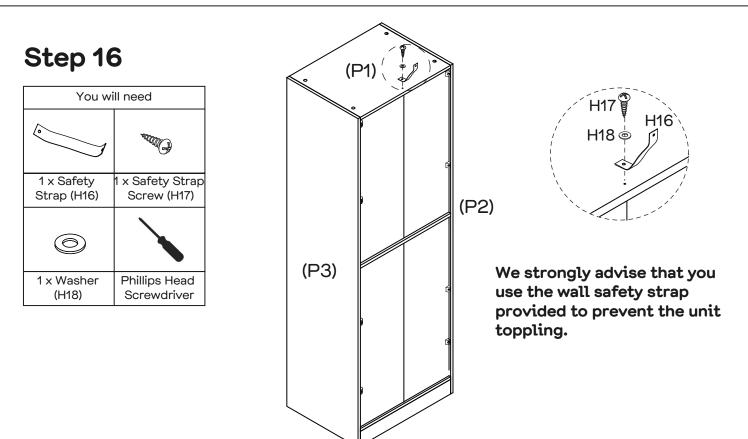
Attach the Safety Strap (H16) to the Top Panel (P1) with  $1 \times \text{Safety Strap Screw}$  (H17) &  $1 \times \text{Washer}$  (H18) by tightening with the Phillips Head Screwdriver.
