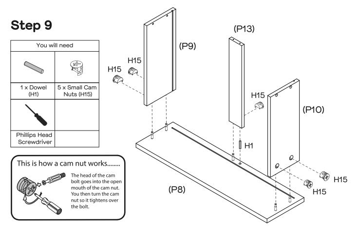
Insert 1 x Dowel (H1) into Drawer Front (P8). Insert 5 x Small Cam Nuts (H15) into Left & Right Drawer Sides (P9 & P10) and Support Rail (P13). Rotate the nuts so the arrows point towards the incoming bolts. Attach the Left & Right Drawer Sides (P9 & P10) and Support Rail (P13) to Drawer Front (P8) by tightening all nuts with the Phillips Head Screwdriver.
