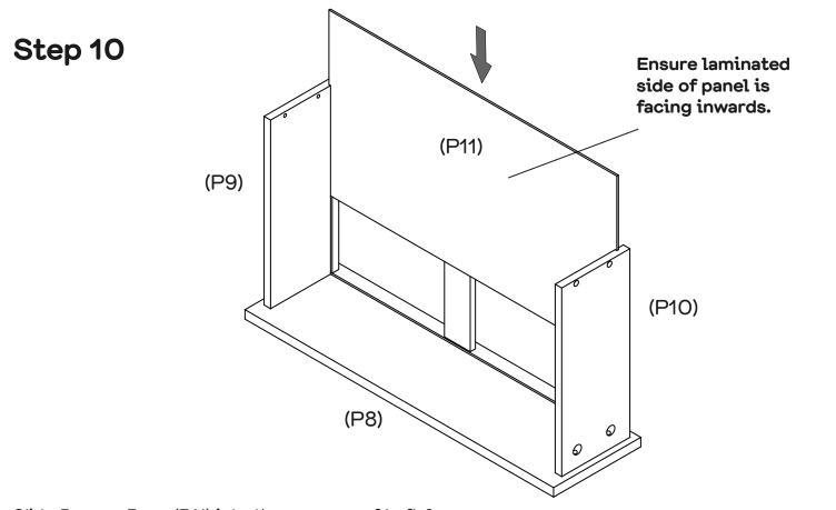
Slide Drawer Base (P11) into the grooves of Left & Right Drawer Sides (P9 & P10) and Drawer Front (P8).
