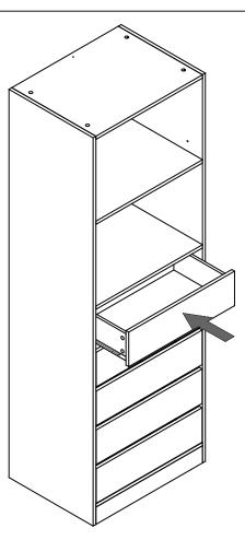
Gently insert the assembled drawers into the unit by carefully lining up the drawer runners with the drawer runner tracks.
