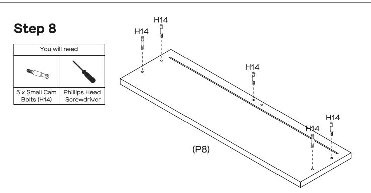
Attach 5 x Small Cam Bolts (H14) to Drawer Front (P8) as shown by tightening with the Phillips Head Screwdriver.
