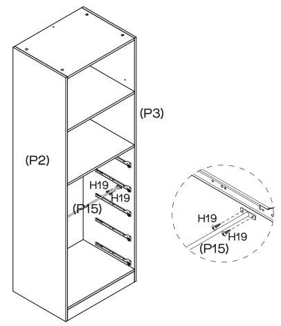
Attach Rail (P15) to Left & Right Side Panels (P2 & P3) with 4  $\times$  Screws (H19) by tightening with the Phillips Head Screwdriver.
