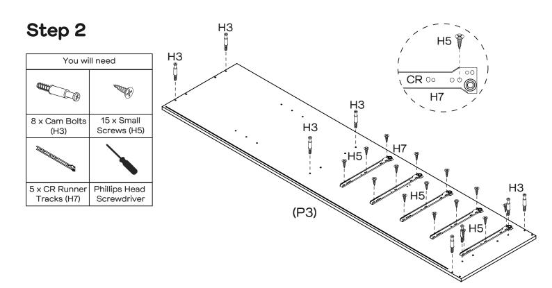
Attach 8 x Cam Bolts (H3) to Right Side Panel (P3) as shown by tightening with the Phillips Head Screwdriver. Attach 5 x CR Runner Tracks (H7) to Right Side Panel (P3) with 15 x Small Screws (H5) by tightening with the Phillips Head Screwdriver.
