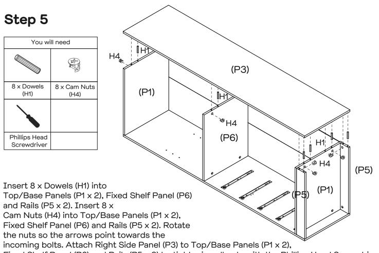
Fixed Shelf Panel (P6) and Rails (P5  $\times$  2) by tightening all nuts with the Phillips Head Screwdriver.
