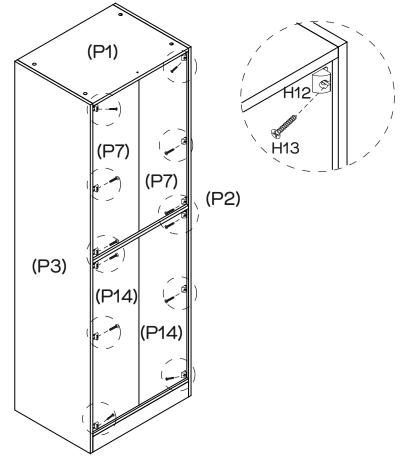
Secure Back Panels (P7 x 2 & P14 x 2) in place with 12 x Wedges (H12) and 12 x Wedge Screws (H13) by tightening with the Phillips Head Screwdriver.
