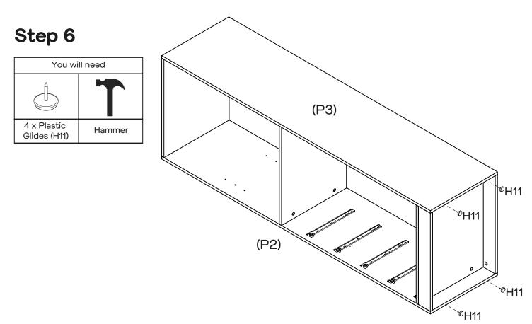
Secure 4 x Plastic Glides (H11) to the bottom of Left & Right Side Panels (P2 & P3) as shown using the Hammer.
