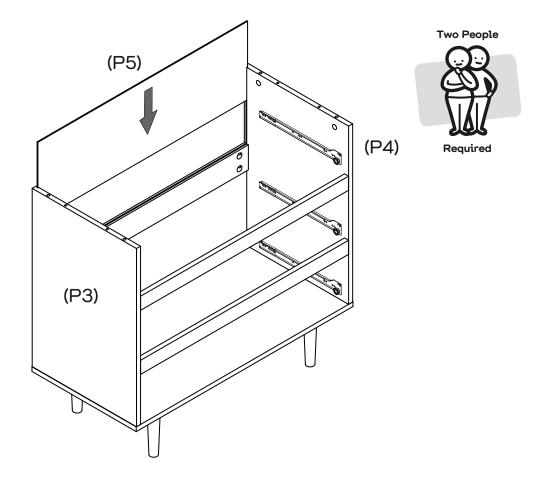
Gently stand the unit upright. Slide 1 x Back Panel (P5) into the grooves of Left & Right Side Panel (P3 & P4).
