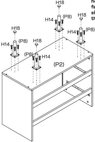
holes on the Leg Plate are facing up, so that the Screws sit flush with the top of the Leg Plate once attached.
