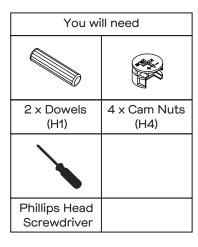
Insert 4 x Cam Nuts (H4) and 2 x Dowels (H1) into Rails (P6 x 2 & P7) as shown. Rotate the cam nuts so the arrows point towards the incoming cam bolts. Attach Left Side Panel (P3) to Rails (P6 x 2 & P7) by tightening all cam nuts with the Phillips Head Screwdriver.
