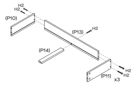
Attach Left & Right Drawer Side (P10  $\times$  3 & P11  $\times$  3) and Support Rail (P14  $\times$  3) to Drawer Back (P13  $\times$  3) with 15  $\times$  Long Screws (H2) by tightening with the Phillips Head Screwdriver.
