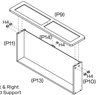
Insert 15 x Cam Nuts (H4) into Left & Right Drawer Side (P10 x 3 & P11 x 3) and Support Rail (P14 x 3) as shown. Rotate the cam nuts so the arrows point towards the incoming cam bolts. Attach Drawer Front (P9 x 3) to Left & Right Drawer Side (P10 x 3 & P11 x 3) and Support Rail (P14 x 3) by tightening all cam nuts with the Phillips Head Screwdriver.
