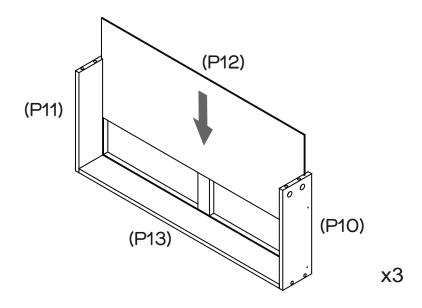
Slide the Drawer Bases (P12  $\times$  3) into the grooves of Left & Right Drawer Sides (P10  $\times$  3 & P11  $\times$  3) as shown.
