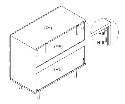
Secure Back Panels (P5  $\times$  2) in place with 4  $\times$  Wedges (H15) using 4  $\times$  Wedge Screws (H16) by tightening with the Phillips Head Screwdriver.
