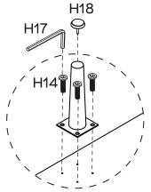
Secure 4 x Leg Plates (H12) to  $4 \times \text{Legs}$  (P8) with  $8 \times \text{Long Bolts}$  (H13) by tightening with an Allen Key (H17). Attach  $4 \times \text{Legs}$  (P8) to Bottom Panel (P2) with  $16 \times \text{Short Bolts}$  (H14) by tightening with an Allen Key (H17). Hammer  $4 \times \text{Plastic Glides}$  (H18) onto the bottom of Legs (P8).
