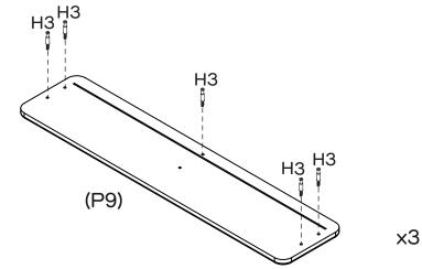
Attach 15 x Cam Bolts (H3) to Drawer Front Panels (P9 x 3) by tightening with the Phillips Head Screwdriver.
