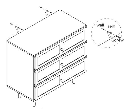
Move the unit to the final position, and attach the safety strap to the wall securely. Make sure it is firmly attached and snug fit.
