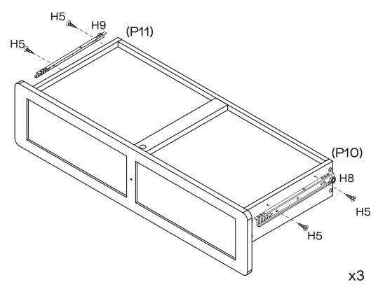
Attach 3 x DL Runners (H8) to the bottom of Left Drawer Side (P10 x 3) and 3 x DR Runner (H9) to the bottom of Right Drawer Side (P11 x 3) with 12 x Small Screws (H5) by tightening with the Phillips Head Screwdriver.
