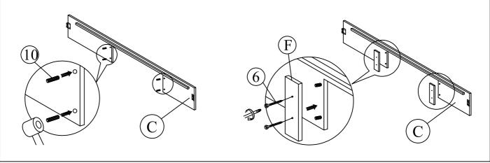
Step 4: Attach side rail (C) to headboard (A) and footboard (B) by pushing the bracket down to fit it.
