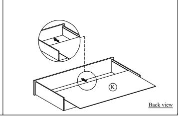
Step 8 : Tighten the bottom panel support (O & P) with screws (7) using screw Step 9 : Tighten the roller (9) with screws (5) using screw driver driver (not included). Attach the bottom panel with Nail (11) using the
